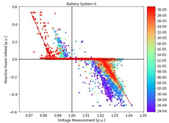
Fig. 11. Reactive power infeed versus the voltage measurement for the battery system G. The colour indicates the time course and the learning progress of the system.
