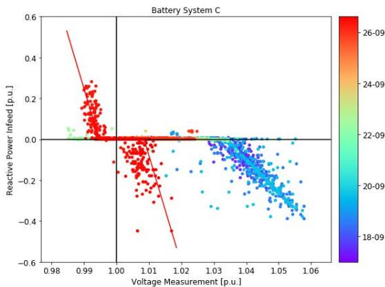
Fig. 14. Reactive power infeed versus the voltage measurement for the battery system C. The colour indicates the time course.
