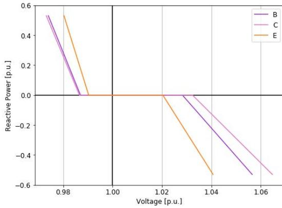
Fig. 8. Parameterised  $Q(U)$  characteristic curve of three battery inverters at different positions.
