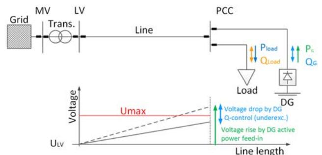
Fig. 1. Impact of active and reactive power on the voltage. [4]
