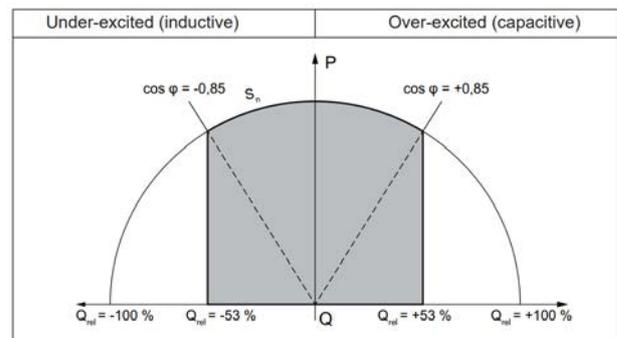
Fig. 4. Possible working area of the inverter. All valid operating points defined by active and reactive power,  $P$  and  $Q$ , are within the grey area. [5]
