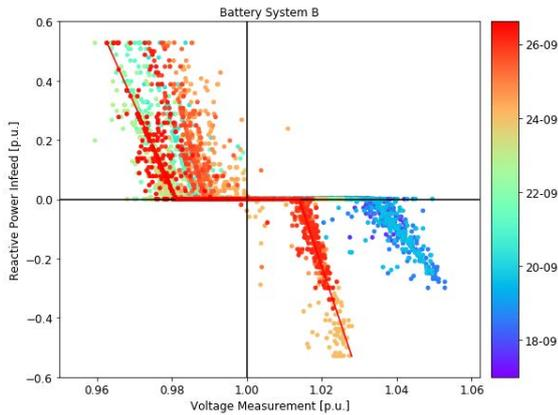
Fig. 13. Reactive power infeed versus the voltage measurement for the battery system B. The colour indicates the time course.
