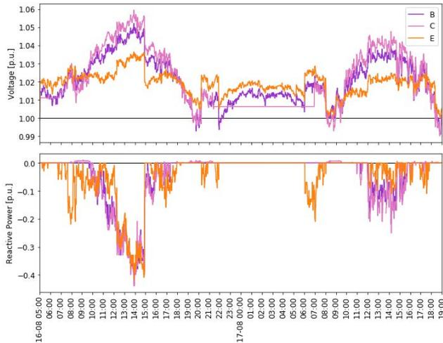
Fig. 9. Example of the voltage dependent reactive power control of three battery inverters at different positions. Top: Measured voltage. Bottom: Reactive power infeed.
