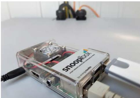
Fig. 2. One of the seven SNOOPI-Boxes controlling a battery inverter installed during the field test.
