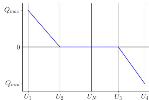
Fig. 3.  $Q(U)$  characteristic curve.
