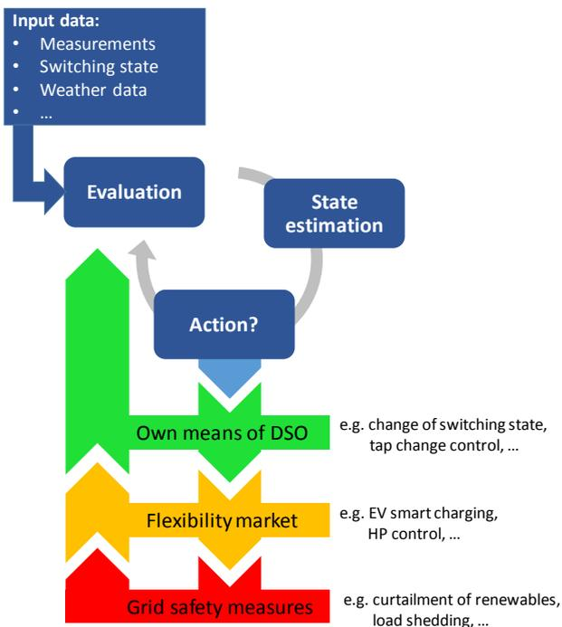
Figure 3. Flow chart of the traffic light concept
