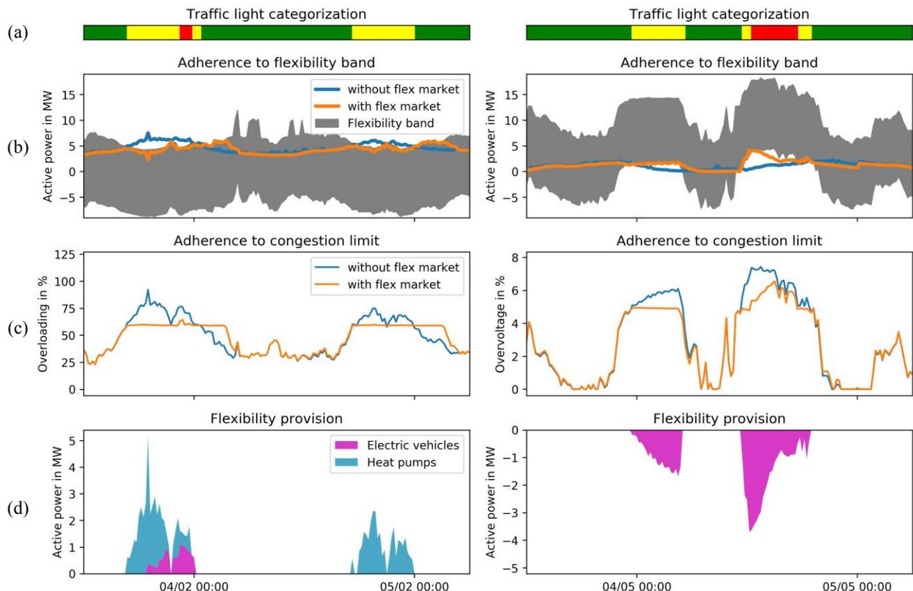
Figure 6. Simulation results with and without flexibility market for two cold winter days (left) and two summer days with high PV and wind energy production (right)
