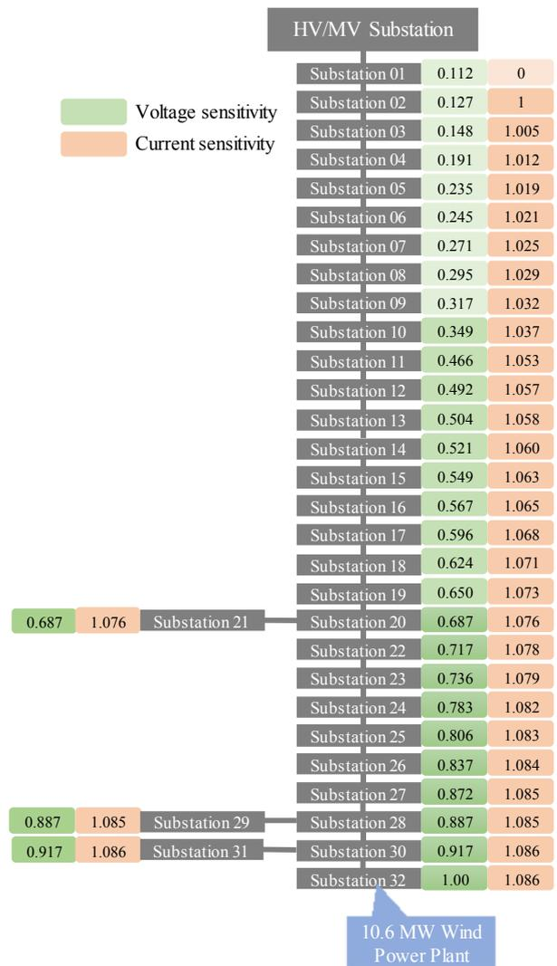
Figure 4. Determination of sensitivities in case of voltage violations and overloading
