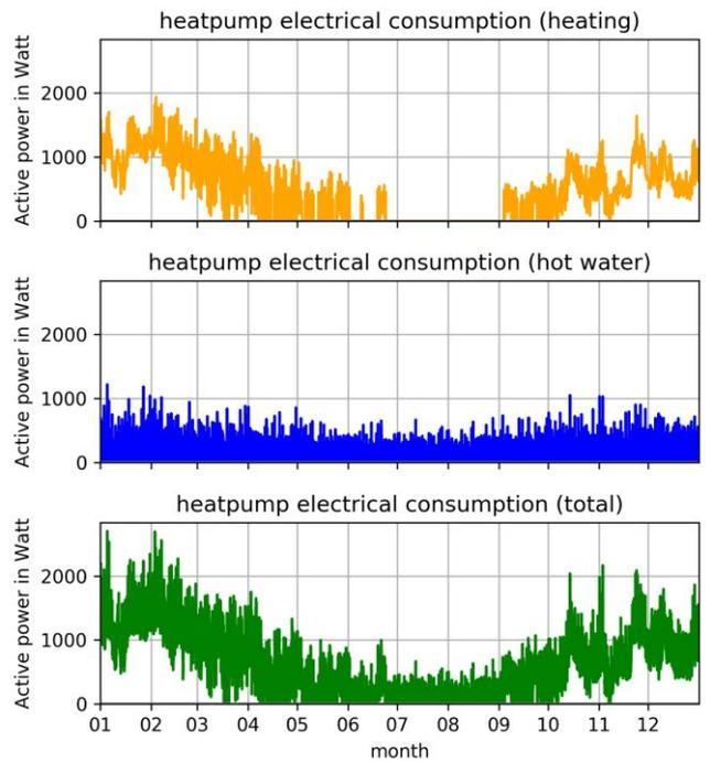
Figure 1. Electrical demand of the heat pump for heating, hot water and in total
