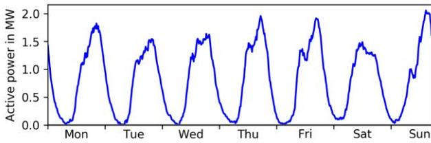
Figure 2. Aggregated electric vehicle charging profile of one week
