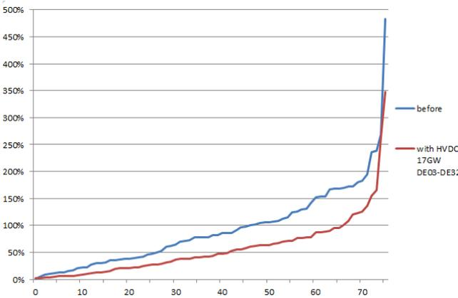
Fig. 2. Loading as a percentage of the thermal limits of the 76 lines in Germany on a windy winter day, with and without an HVDC line carrying 17 GW from Hamburg (DE03) to Freiburg (DE32).
