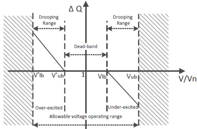
Fig.2 : Graphical schematic of droop-based voltage control.
