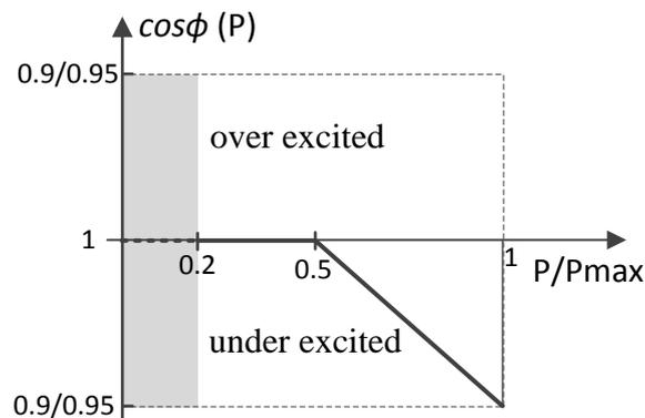
Fig. 1: Standard characteristic curve for  $\cos\phi (P)$
