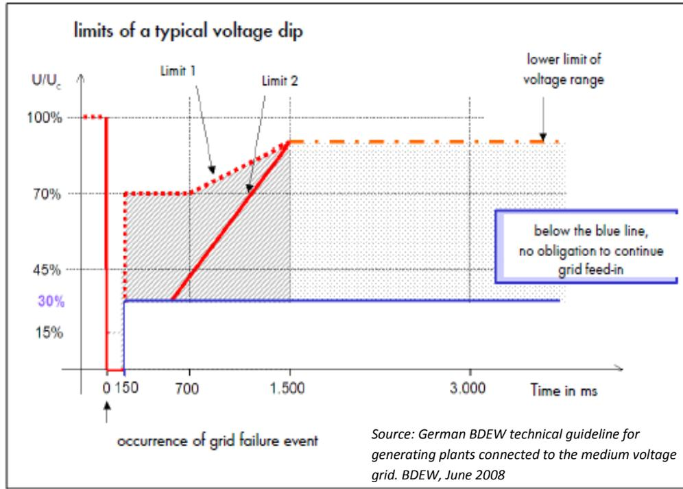
Figure 6-3 Voltage support that must be given by generating plants connected to medium voltage network
