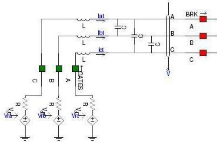
Figure 2-8 A transient model of PV inverter in a study on fault contribution of grid-connected inverters [14]
