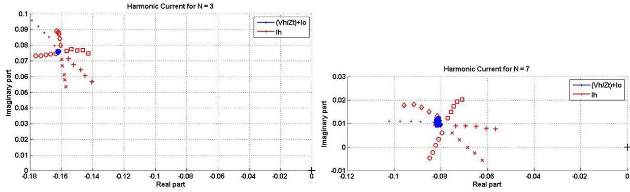
Figure 4-19 3Φ inverter's 3<sup>rd</sup> and 7<sup>th</sup> harmonic currents produced by 5<sup>th</sup> harmonic voltage at output power 0.8kWac
