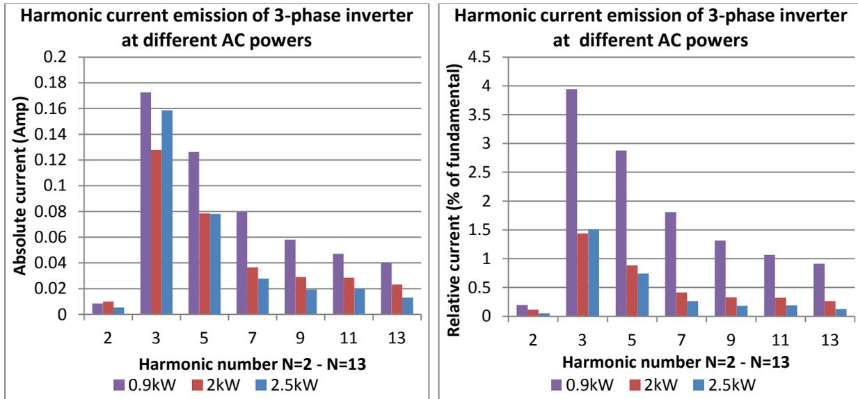
Figure 5-6 Harmonic current emission of 3Φ inverter at various AC output power, shown in absolute value (Amp) and relative to fundamental (%)
