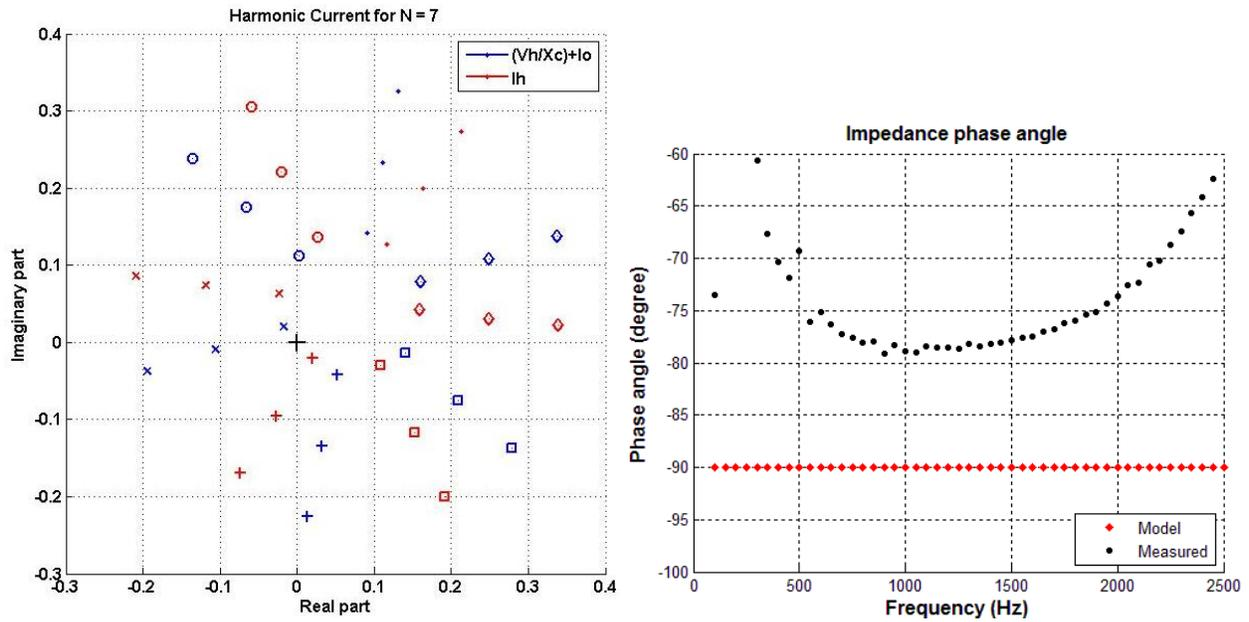
Figure 4-14 7<sup>th</sup> harmonic fingerprint of measured and model current with phase angle profile of measured data and model of Inverter3, there is about 20° phase angle difference
