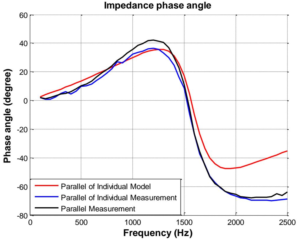
Figure F-8 Impedance phase angle profile of aggregation of 3Φ inverter and power router
