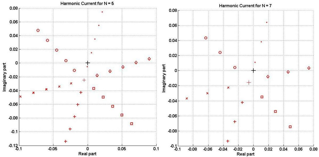
Figure 5-1 Harmonic fingerprints of Inverter1 for 5<sup>th</sup> and 7<sup>th</sup> harmonic showing the harmonic current with and without harmonic background voltage
