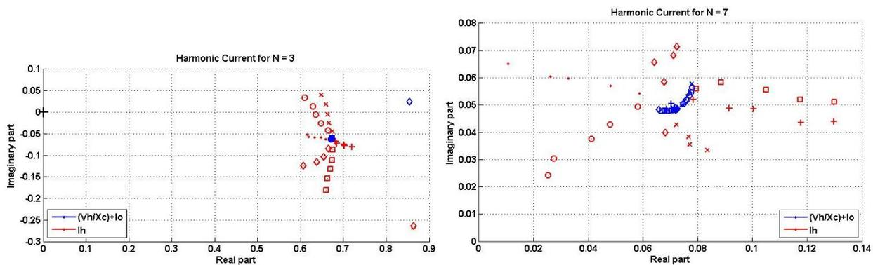
Figure 4-18 Inverter3’s 3<sup>rd</sup> and 7<sup>th</sup> harmonic currents produced by 5<sup>th</sup> harmonic voltage at output power 0.8kWac
