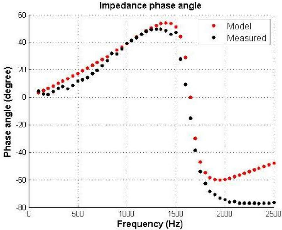
Figure 4-16 Power router model phase angle profiles compared to measured phase angle profiles
