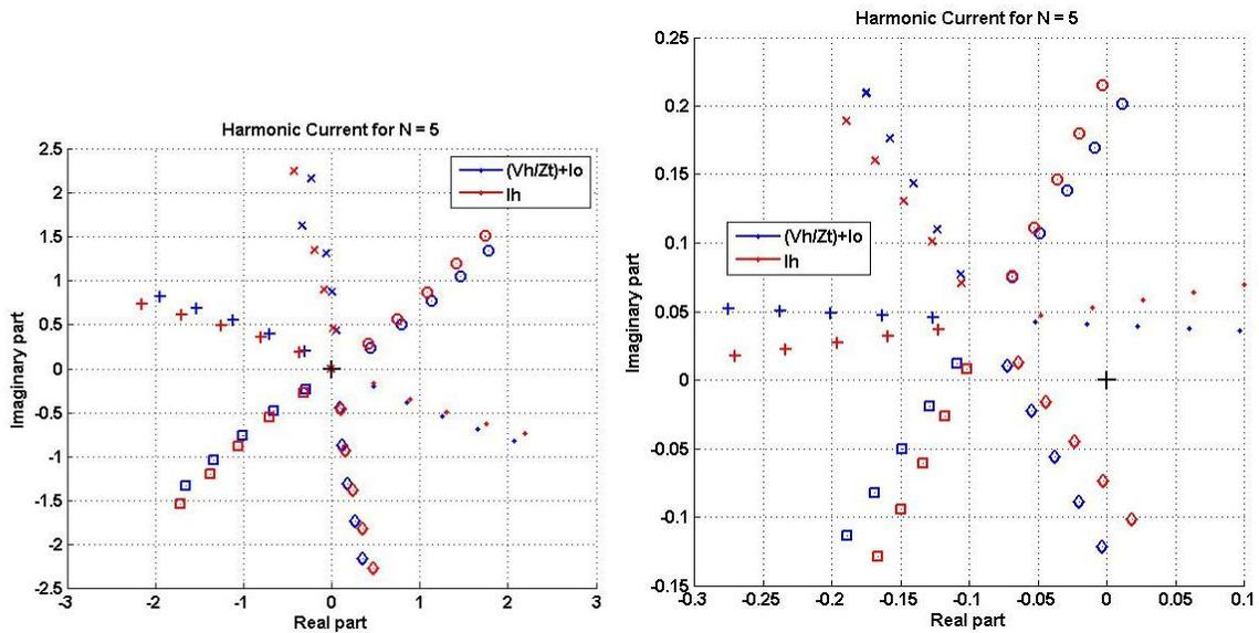
Figure 4-17 The 5<sup>th</sup> harmonic current fingerprint of measured and model current of power router and 3Φ inverter, respectively
