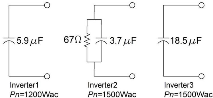
Figure 4-5 The impedance models of single phase PV inverters
