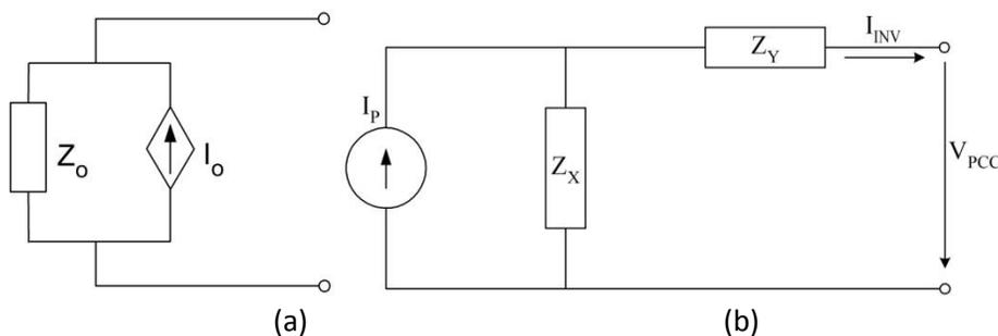
Figure 2-10 Norton model of PV inverter: (a) all output impedances are represented by  $Z_o$  and (b) output capacitor is represented with  $Z_x$  while output resistor and/or inductor is represented by  $Z_y$
