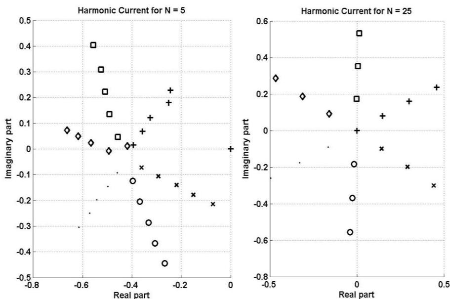
Figure 4-1 Comparison of current behaviour at 5<sup>th</sup> and 25<sup>th</sup> harmonic at single-phase inverter
