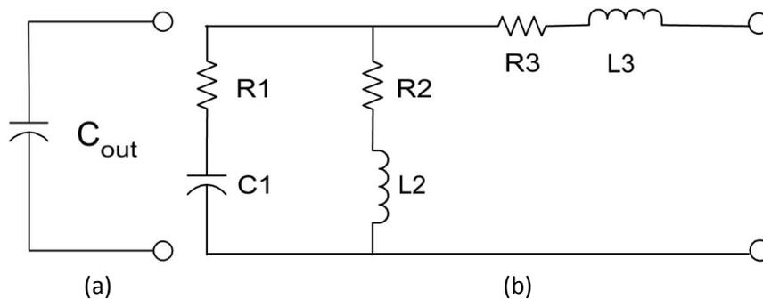
Figure 7-1 Simple model for 1 $\Phi$  inverters in the class 0-2kW and more complex model for 1 $\Phi$  inverters in the class 2-5kW
