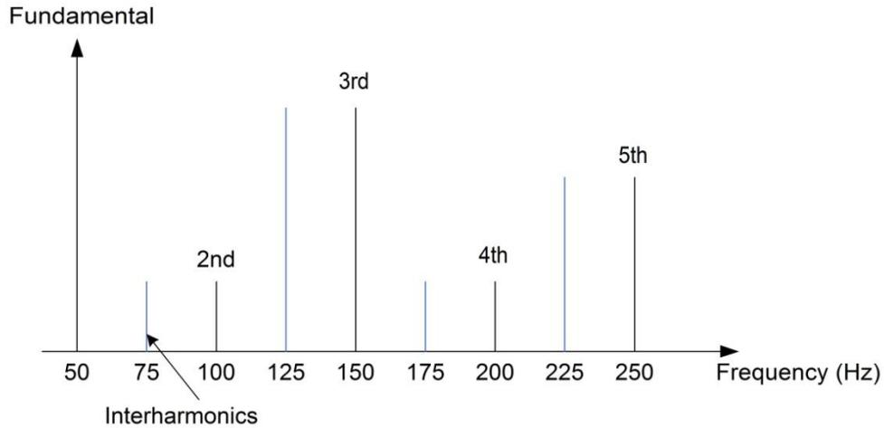
Figure 3-2 The interharmonic signals used for the measurement
