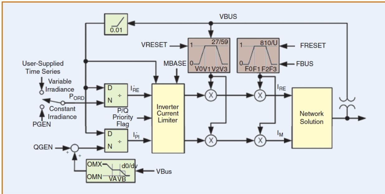
Figure 2-7 An example of dynamic model of PV system
