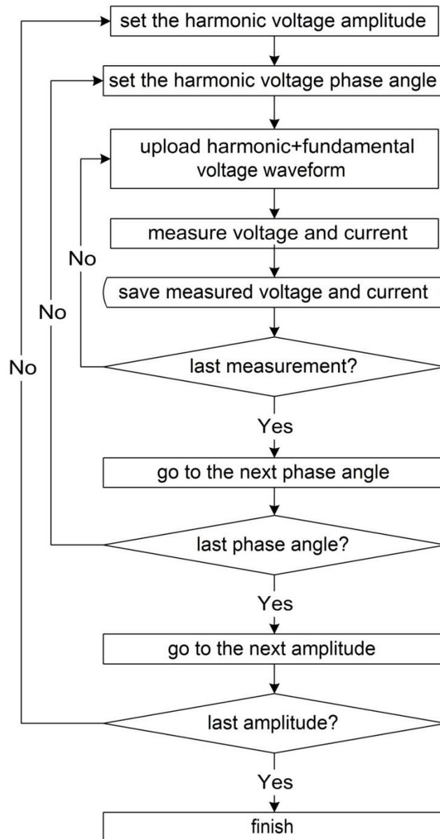
Figure 3-5 Process flow of the PV inverter impedance measurement system
