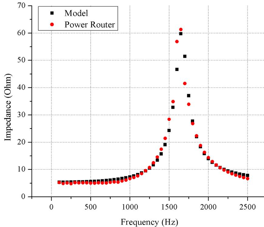
Figure 4-6 The impedance profile of power router and the fitted curve
