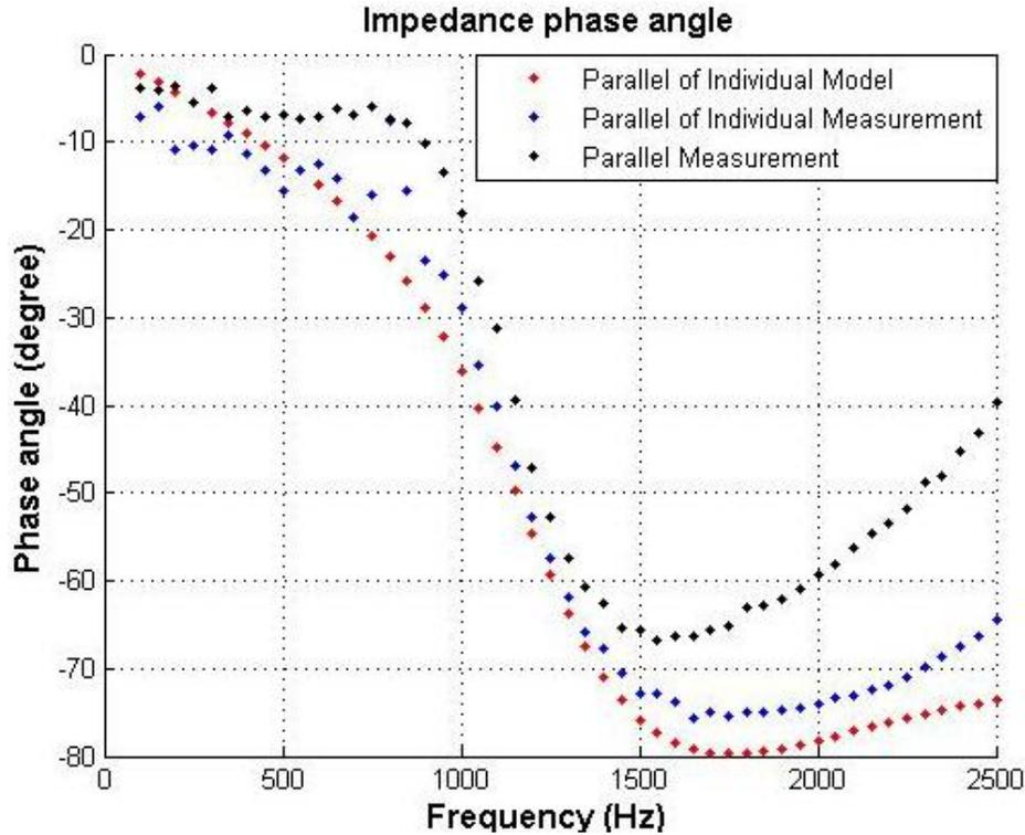
Figure 7-5 Impedance phase angle profile of the aggregation of all inverters
