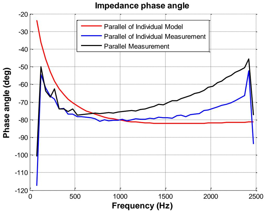
Figure F-11 Impedance phase angle profile of aggregation of Inverter1, Inverter2, Inverter3, and 3Φ inverter
