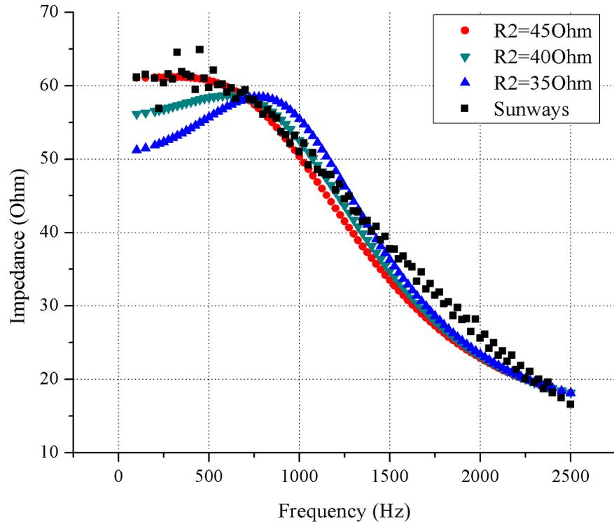
Figure 4-8 The impedance profile of three phase inverter and the fitted curve for different damping resistor values
