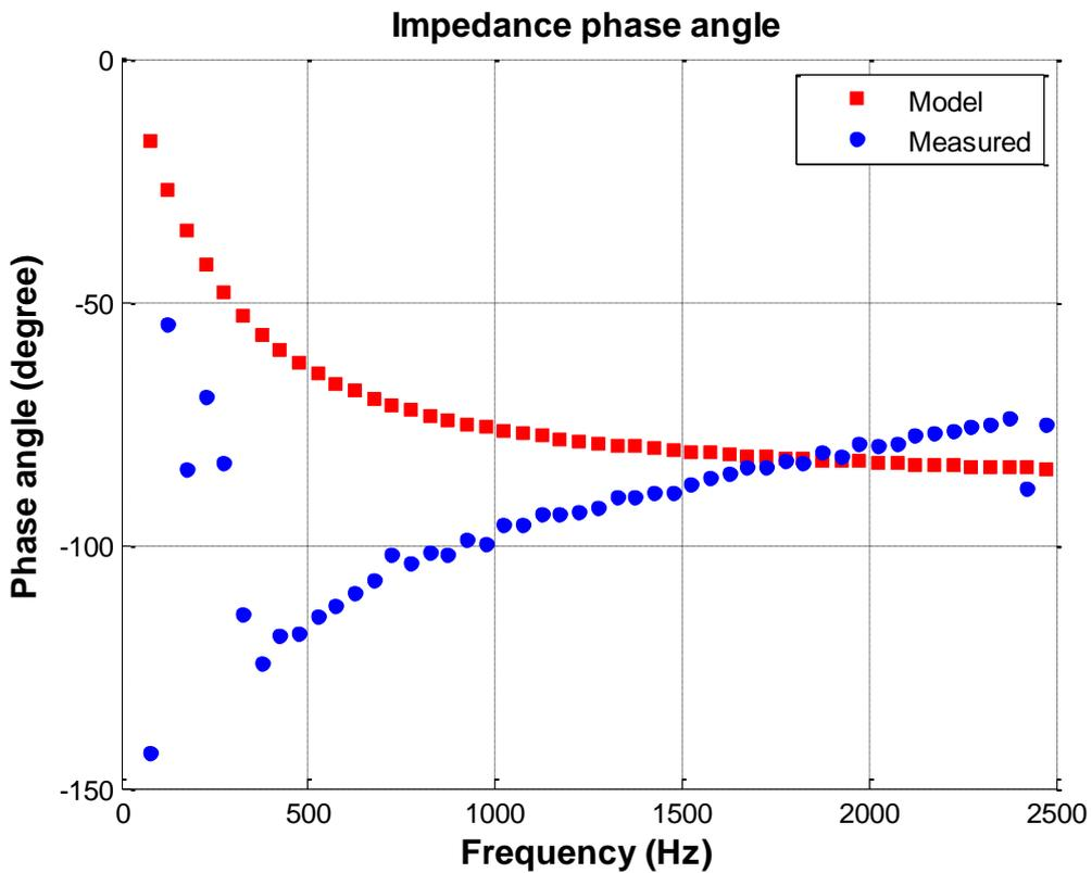
Figure F-2 Impedance phase angle profile of aggregation of Inverter1 and Inverter2
