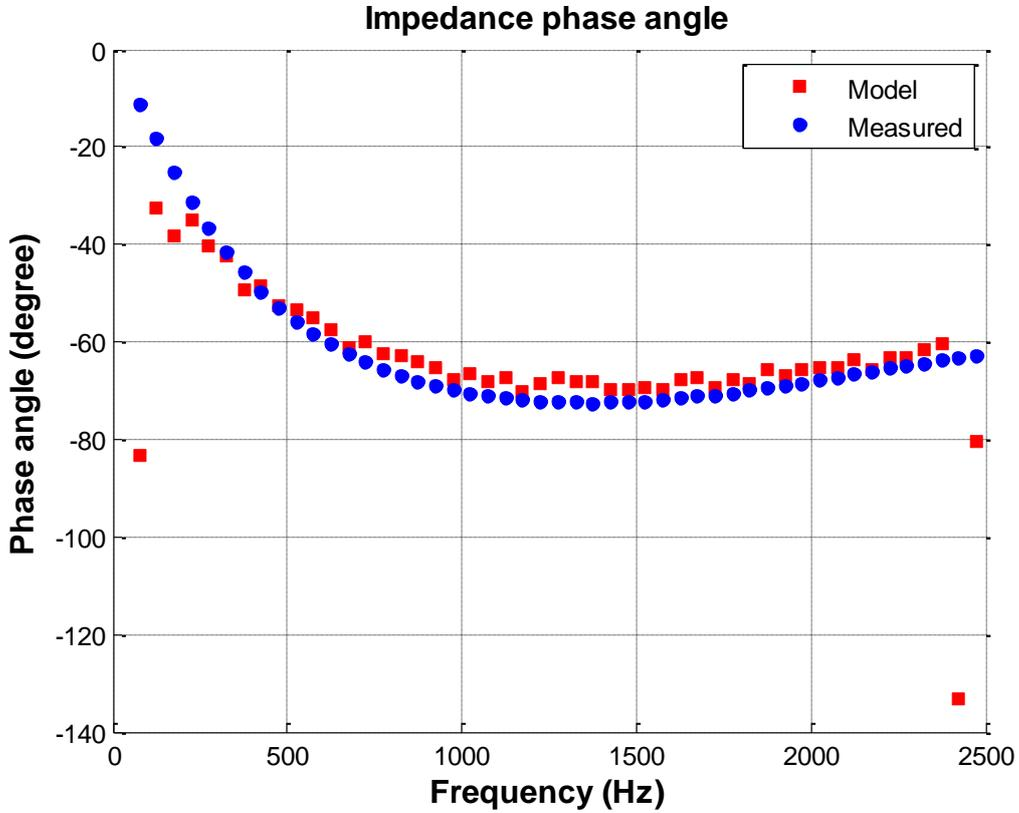
Figure F-6 Impedance phase angle profile of aggregation of Inverter1 and 3Φ inverter
