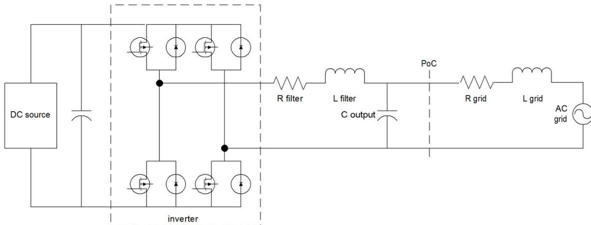
Figure 2-1 Topology of a single phase grid-connected inverter
