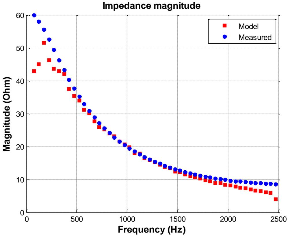
Figure F-5 Impedance magnitude profile of aggregation of Inverter1 and 3Φ inverter
