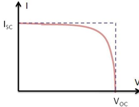
Figure 5-2 IV curve of solar cell as mimicked by PV simulator, the outer line shows the IV curve of DC supply
