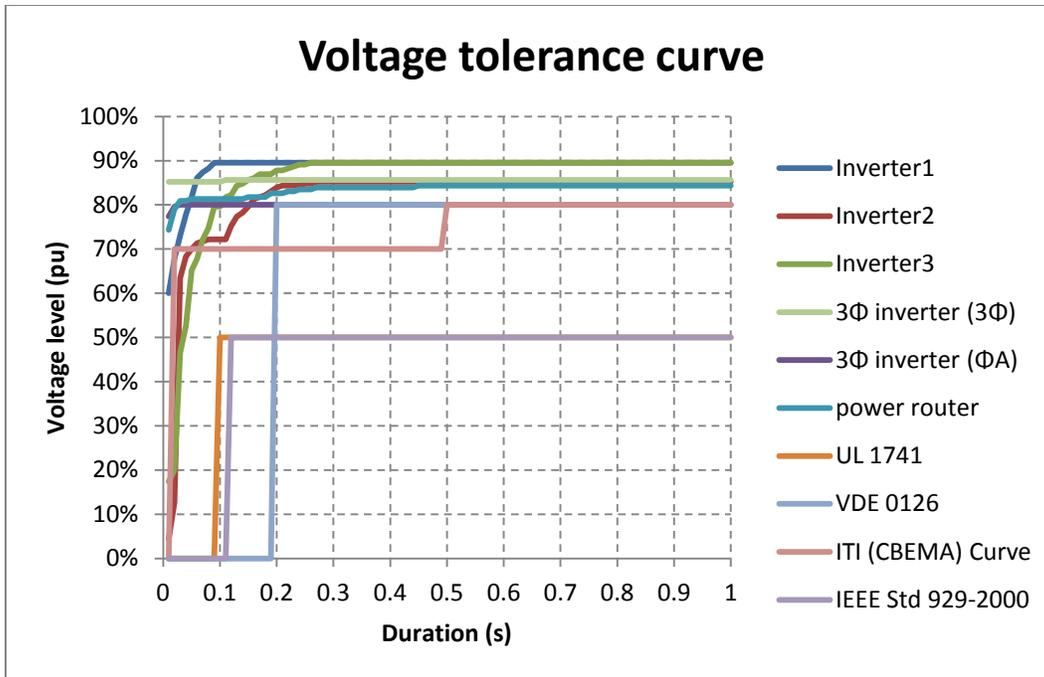
Figure 6-2 Voltage tolerance curve for all inverters, compared to several known requirements
