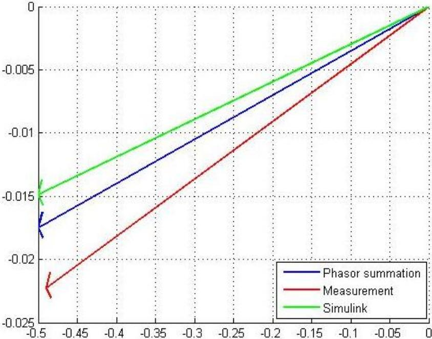
Figure 7-6 Comparison of aggregated 5<sup>th</sup> harmonic current from Inverter1 and Inverter3
