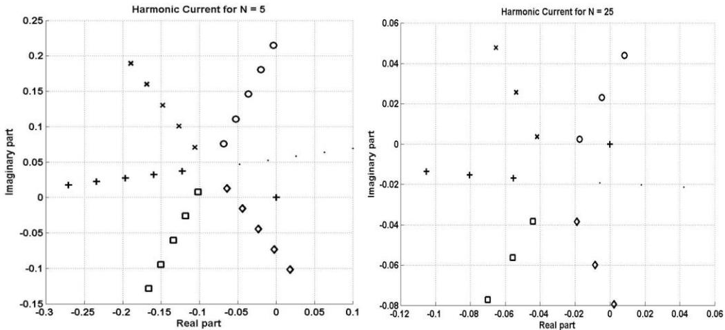
Figure 4-10 Comparison of current behaviour at 5<sup>th</sup> and 25<sup>th</sup> harmonic of 3Φ inverter
