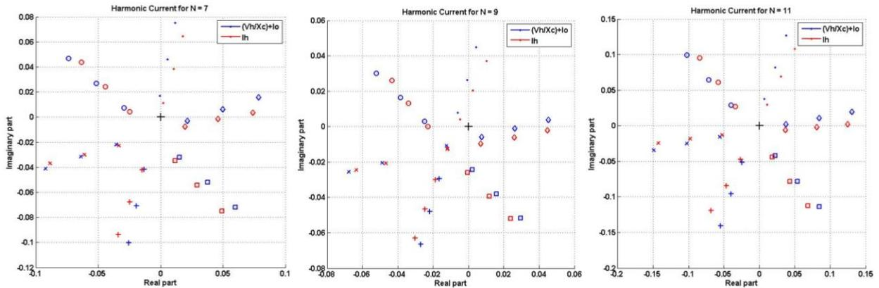
Figure 4-15 7<sup>th</sup>, 9<sup>th</sup>, and 11<sup>th</sup> harmonic fingerprint of measured and model current of Inverter1
