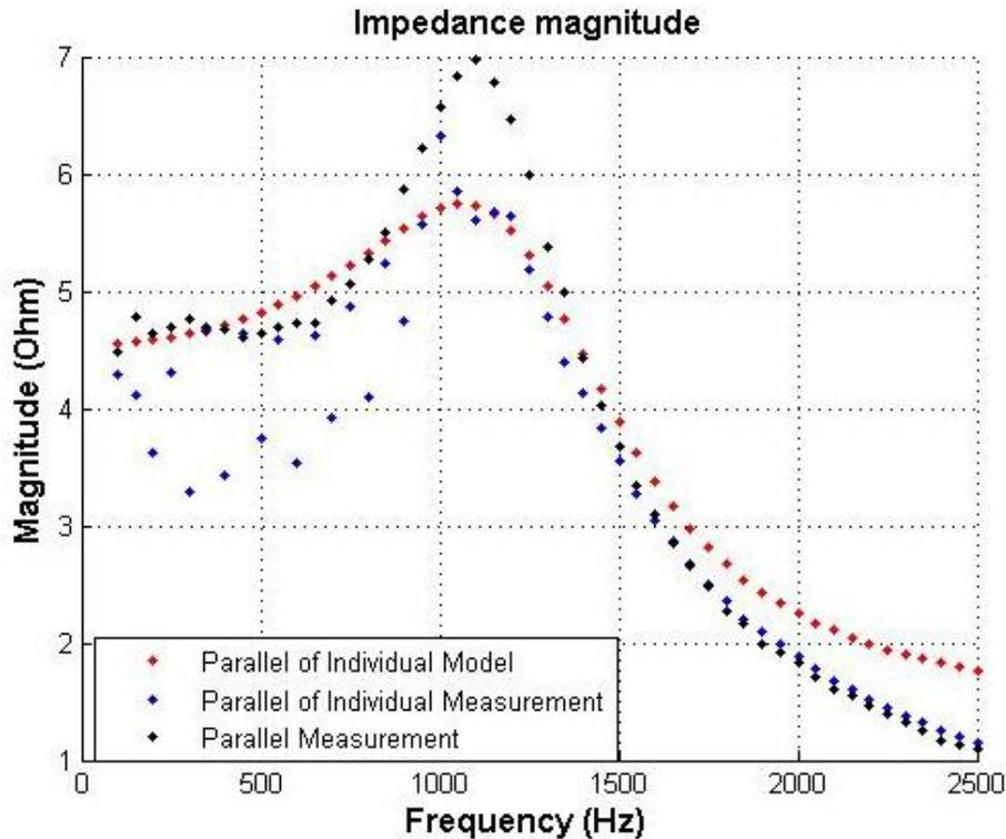
Figure 7-4 Impedance profile of the aggregation of all inverters
