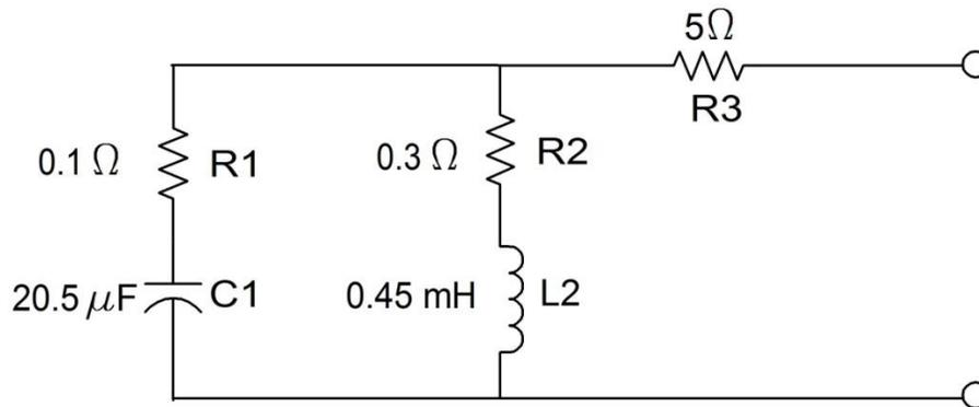
Figure 4-7 The impedance model of single-phase power router
