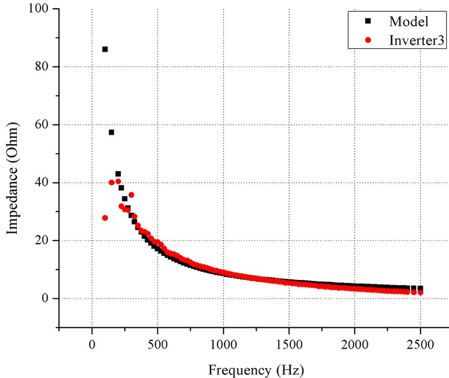
Figure 4-4 The impedance profile of Inverter3 and fitted curve
