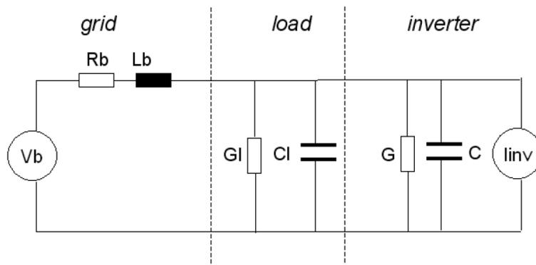
Figure 2-9 A model of grid-connected PV inverter using parallel capacitor and conductor
