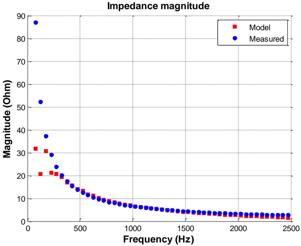
Figure F-3 Impedance magnitude profile of aggregation of Inverter1 and Inverter3
