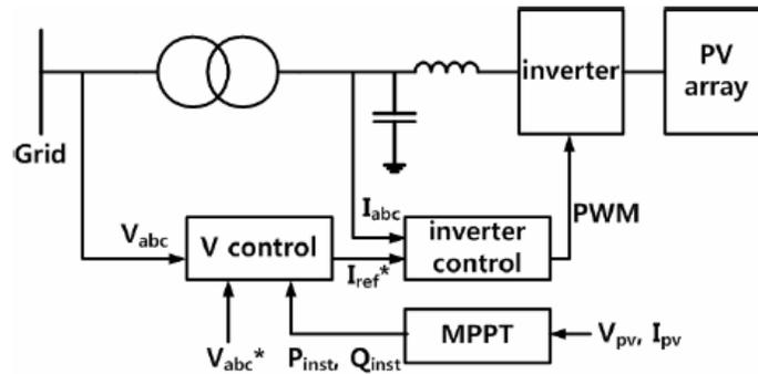
Figure 2-5 The proposed operation scheme of PV inverter that adjusts its active and reactive power to regulate the voltage of the network
