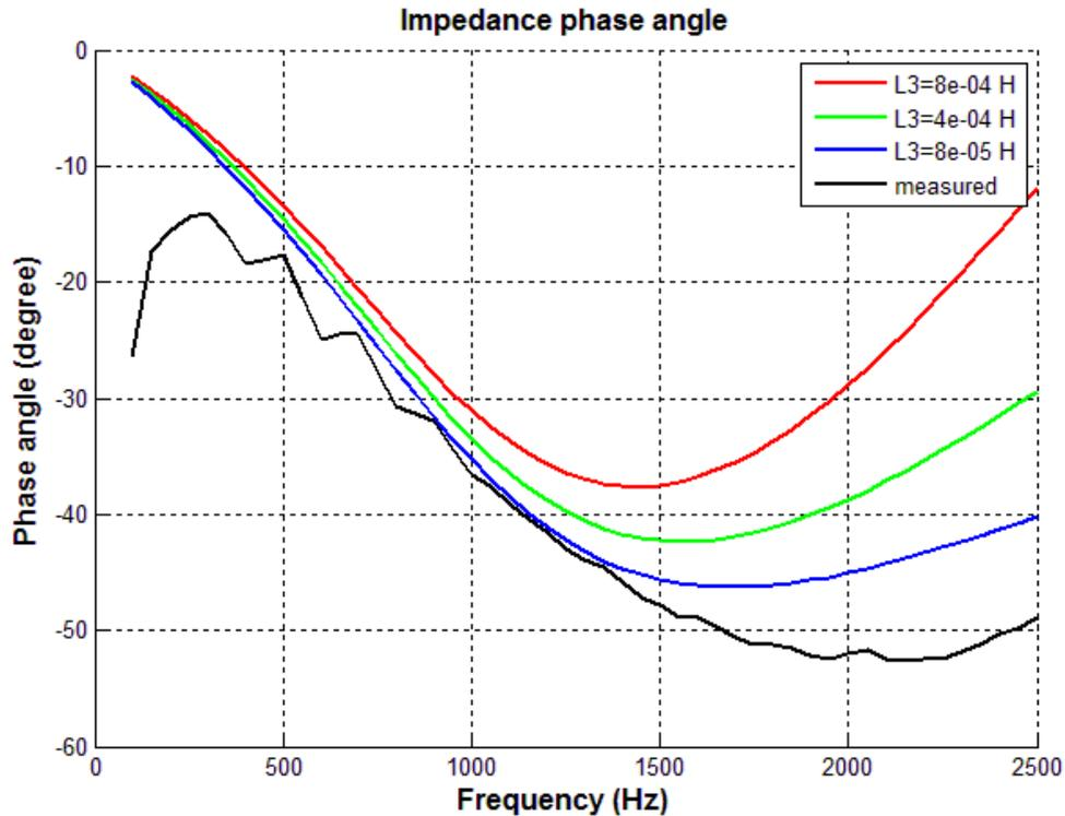
Figure 4-11 Three-phase inverter model phase angle profiles when the series inductance is changed, compared to measured phase angle profiles
