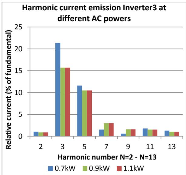
Figure 5-5 Harmonic current emission of Inverter3 at various AC output power, shown in absolute value (Amp) and relative to fundamental (%)
