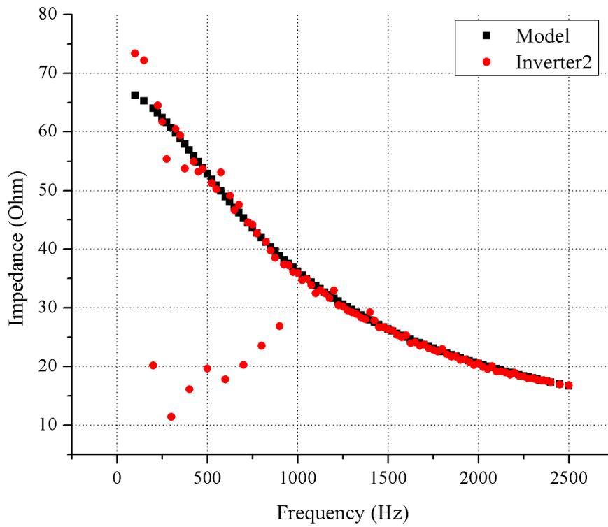
Figure 4-3 The impedance profile of Inverter2 and fitted curve
