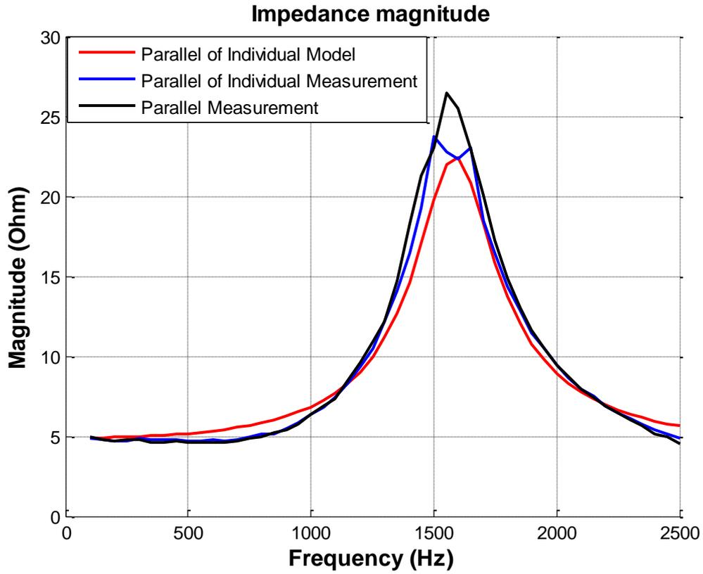
Figure F-7 Impedance magnitude profile of aggregation of 3Φ inverter and power router
