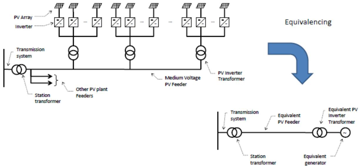
Figure 2-6 Equivalent circuit of utility-scale PV plants [12]
