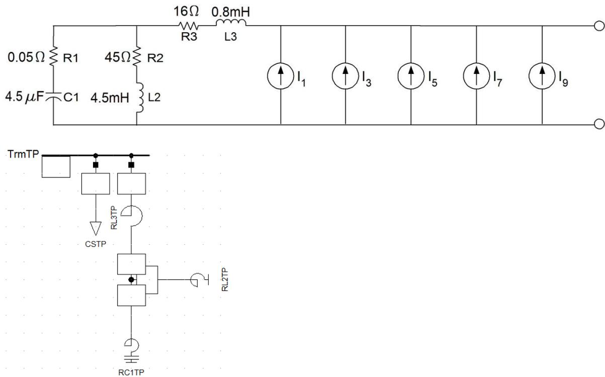
Figure C-4 Complete model of 3Φ Inverter in Simulink and PowerFactory simulation
