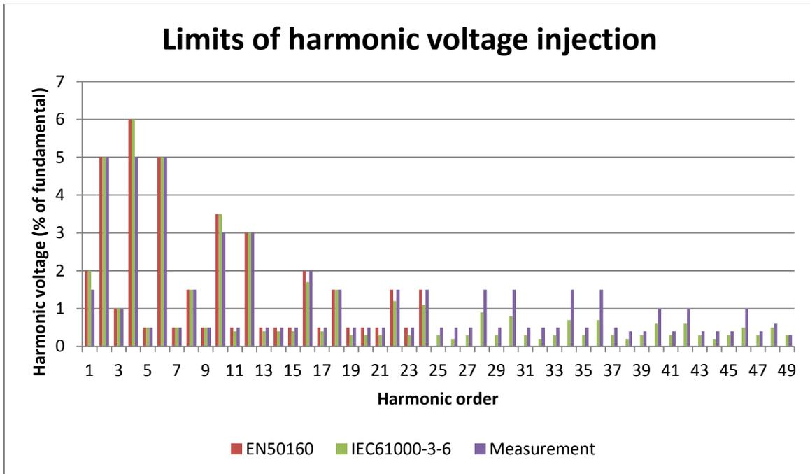
Figure 3-3 The stimuli amplitude spectrum compared to EN50160 and IEC61000-3-6 limits
