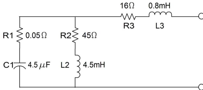
Figure 4-9 The impedance model of 3Φ inverter
