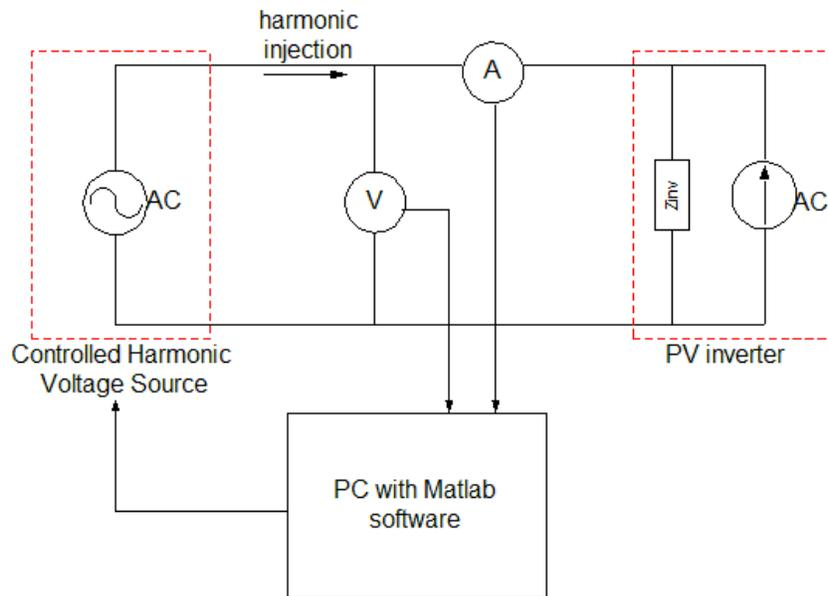
Figure 3-4 PV inverter impedance measurement set-up
