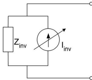
Figure 2-11 A model of PV inverter used harmonic study
