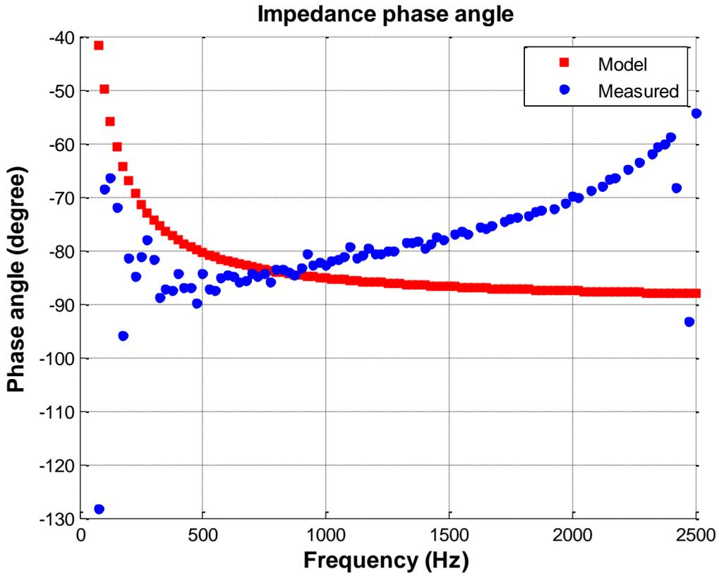
Figure F-9 Impedance phase angle profile of aggregation of Inverter1, Inverter2 and Inverter3
