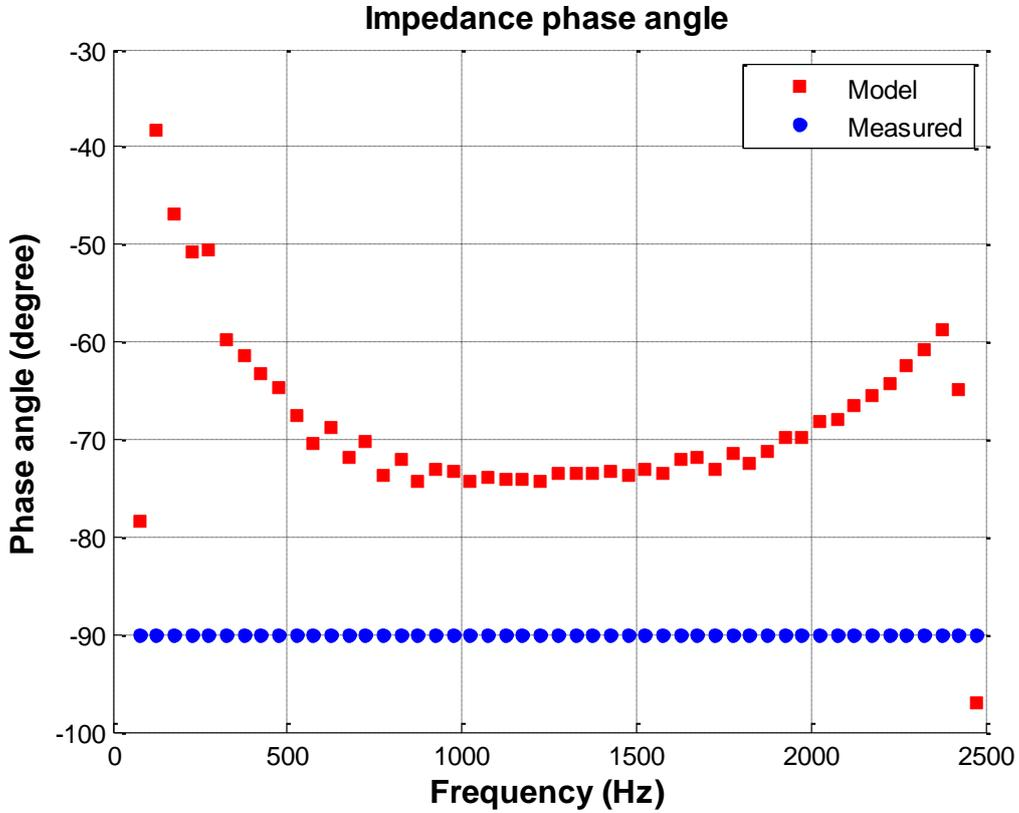
Figure F-4 Impedance phase angle profile of aggregation of Inverter1 and Inverter3
