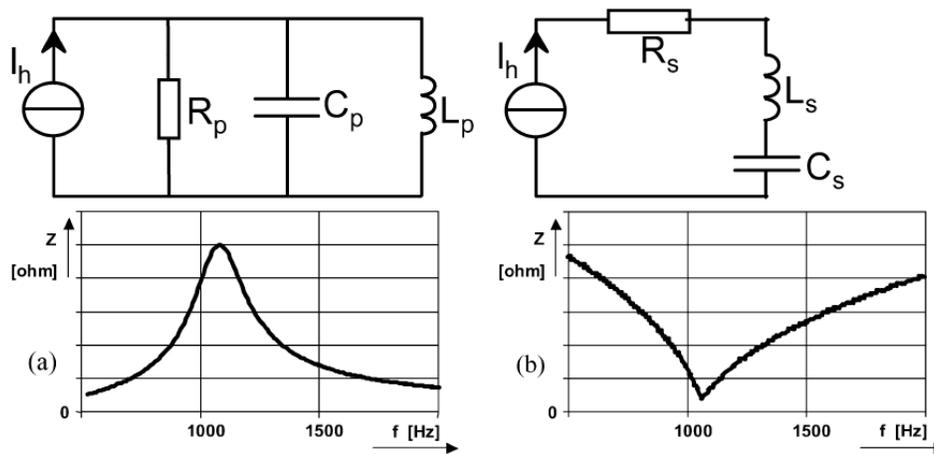
Figure 2-2 Mechanism of series and parallel resonance [2]
