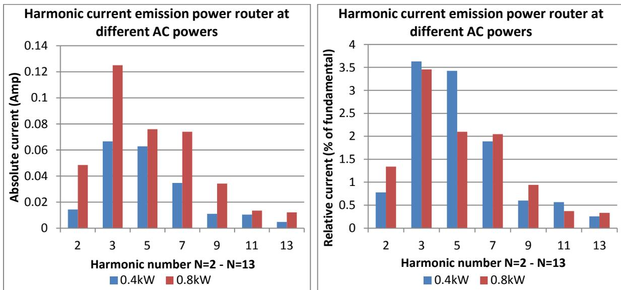
Figure 5-7 Harmonic current emission of power router at various AC output power, shown in absolute value (Amp) and relative to fundamental (%)
