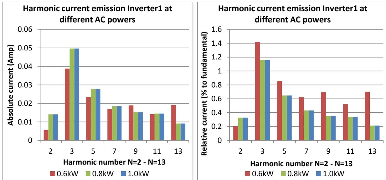
Figure 5-3 Harmonic current emission of Inverter1 at various AC output power, shown in absolute value (Amp) and relative to fundamental (%)
