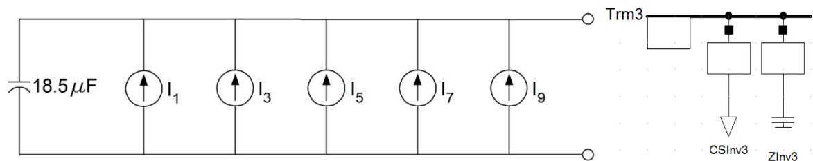
Figure C-3 Complete model of Inverter3 in Simulink and PowerFactory simulation
