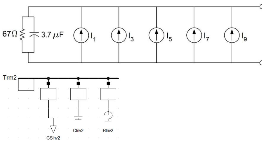
Figure C-2 Complete model of Inverter2 in Simulink and PowerFactory simulation
