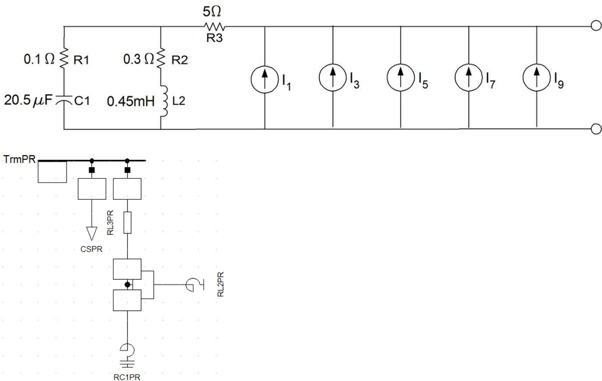
Figure C-5 Complete model of power router in Simulink and PowerFactory simulation
