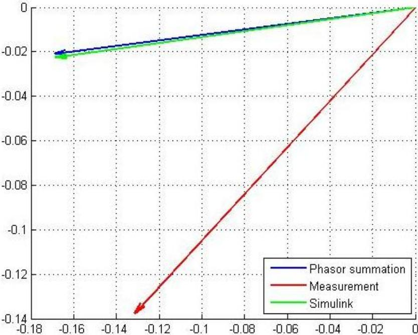
Figure 7-7 Comparison of aggregated 7<sup>th</sup> harmonic current from all inverters
