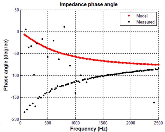
Figure 4-13 7<sup>th</sup> harmonic fingerprint of measured and model current with phase angle profile of measured data and model of Inverter2, there is about 120° phase angle difference
