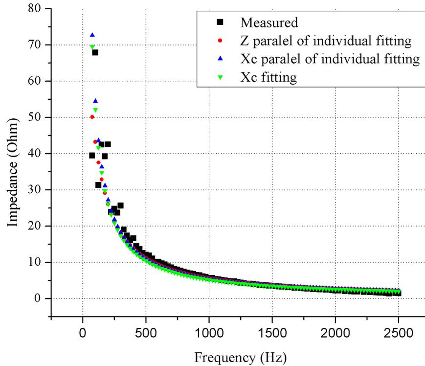
Figure 7-3 The impedance profile of an aggregation of three 1Φ inverters
