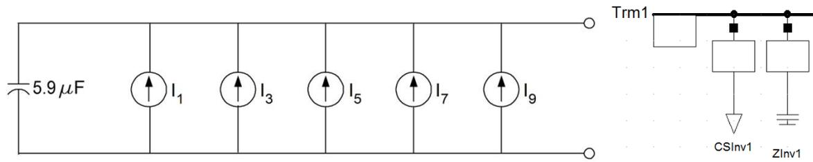
Figure C-1 Complete model of Inverter1 in Simulink and PowerFactory simulation
