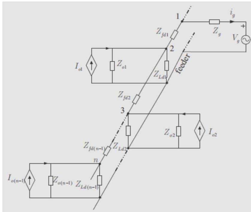
Figure 2-12 Impedance-model representation of a distribution grid with multiple inverter systems connected
