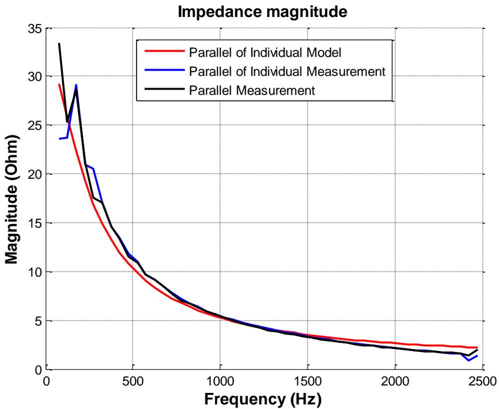
Figure F-10 Impedance magnitude profile of aggregation of Inverter1, Inverter2, Inverter3, and 3Φ inverter
