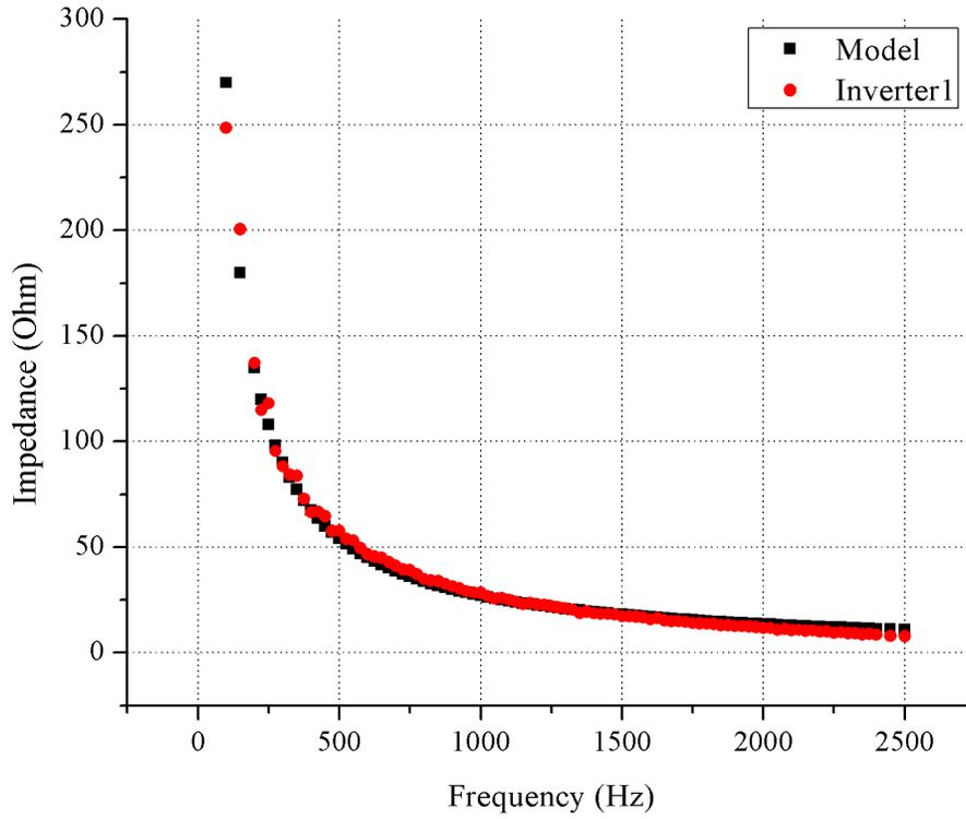
Figure 4-2 The impedance profile of Inverter1 and fitted curve
