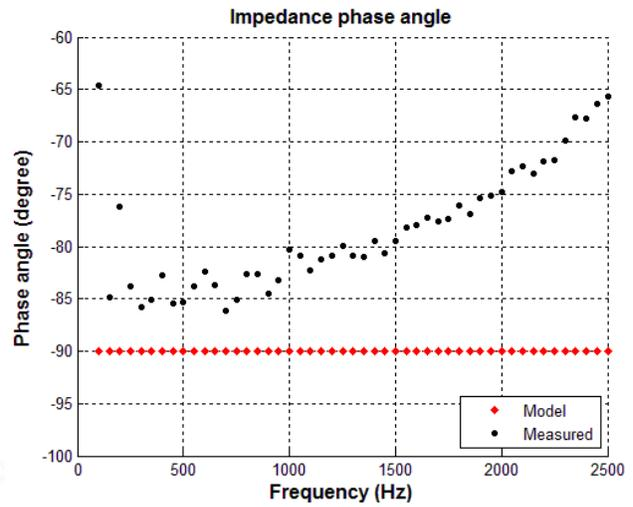
Figure 4-12 7<sup>th</sup> harmonic fingerprint of measured and model current with phase angle profile of measured data and model of Inverter1, there is about 5° phase angle difference
