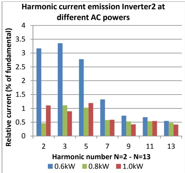
Figure 5-4 Harmonic current emission of Inverter2 at various AC output power, shown in absolute value (Amp) and relative to fundamental (%)
