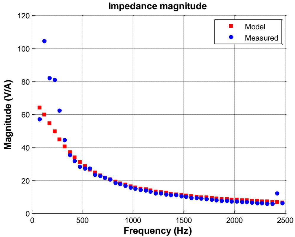
Figure F-1 Impedance magnitude profile of aggregation of Inverter1 and Inverter2
