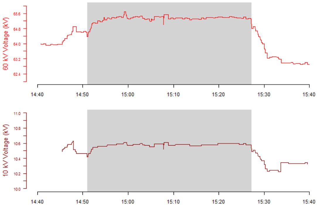
Figure 34 BID Substation Voltage Control during Islanding (60 and 10 kV). The traces compare the 60 kV and the 10 kV voltages at the BID substation during the test.
