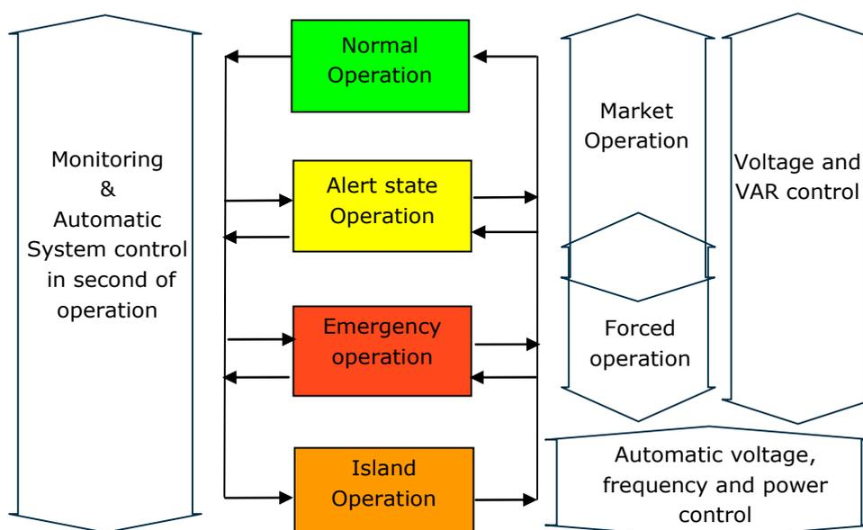
Figure 48 Parallel Operating Forms for Cells and Transmission Areas
