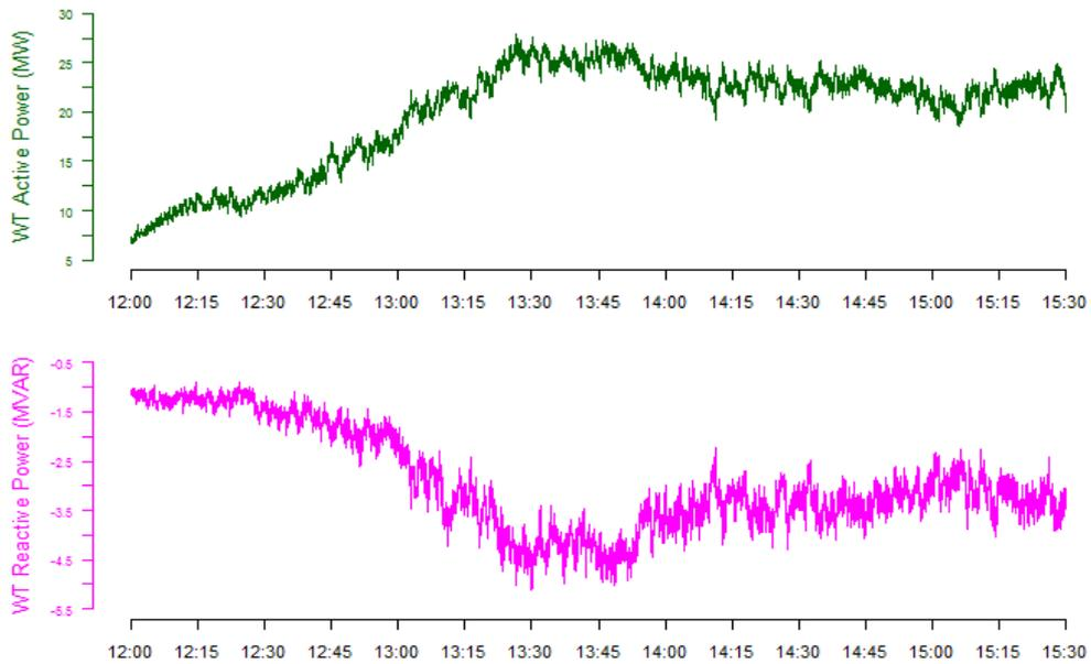
Figure 42: Total wind turbine power production and reactive power consumption
