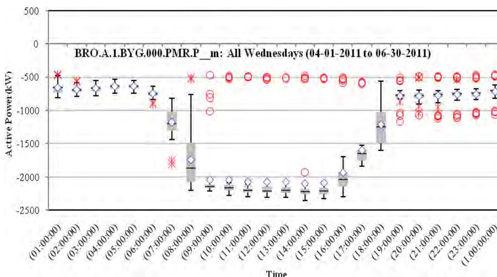
Figure 20 Load as Function of Hour of Day for an Industrial Feeder. The boxplots summarise the quantiles of the observed load (kW), by hour of the day, for all Wednesdays between 2011-04-01 and 2011-06-30; the grey boxes capture the middle 50%; outliers are indicated by red symbols.
