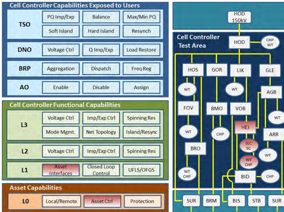
Figure 26 Cell Controller Configuration during Mini-Island Test (Wind Only Operation).
