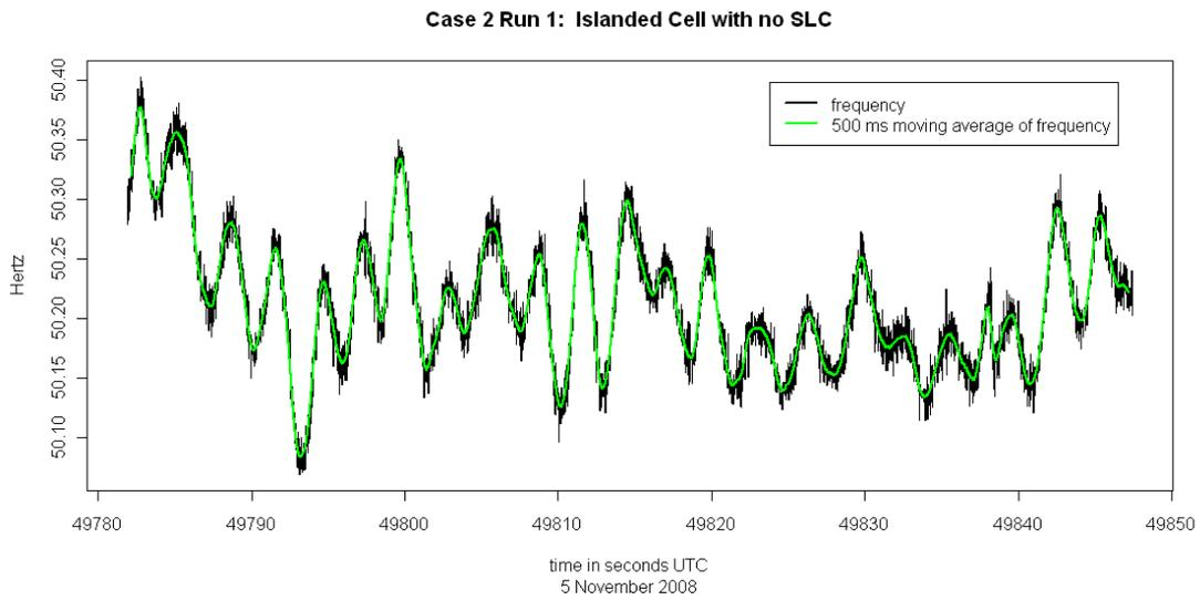
Figure 23 *Islanded Cell with Inactive SLC – Frequency Signal. One minute "snapshot" of the entire trace collected during testing. The black trace plots the metered high speed data and the green trace plots the 50 ms moving average. Note the strong presence of periodicity in the time series when the SLC is offline.*
