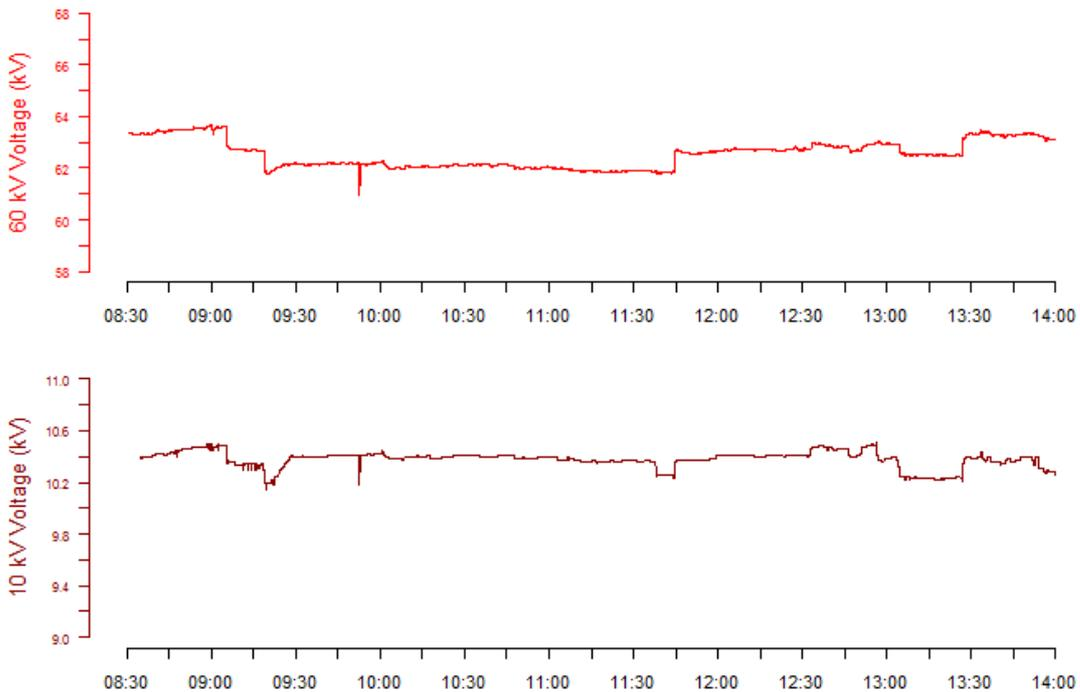
Figure 45 Recorded high (60 kV) and low (10 kV) side voltages at the primary interconnect (HOD) during testing of Multi-Function Operations
