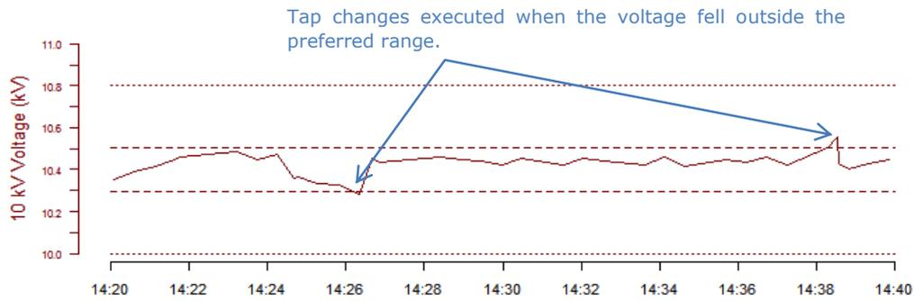
Figure 41 Example of Cell Controller adjusting tap on 60/10 kV transformer. The preferred and allowable ranges are indicated by the dashed and dotted lines, respectively.
