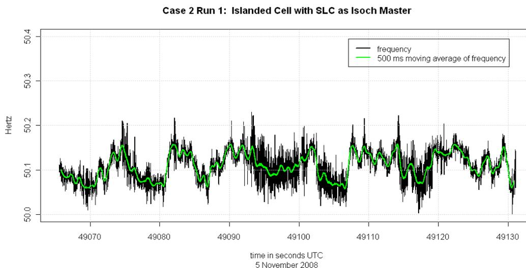
Figure 25 *Islanded Cell with SLC in Isochronous Frequency Master mode – Frequency Signal. One minute “snapshot” of the entire trace collected during testing. The black trace plots the metered high speed data and the green trace plots the 50 ms moving average. Similar to the baseload case, the periodicity observed when the SLC was offline has been significantly reduced.*
