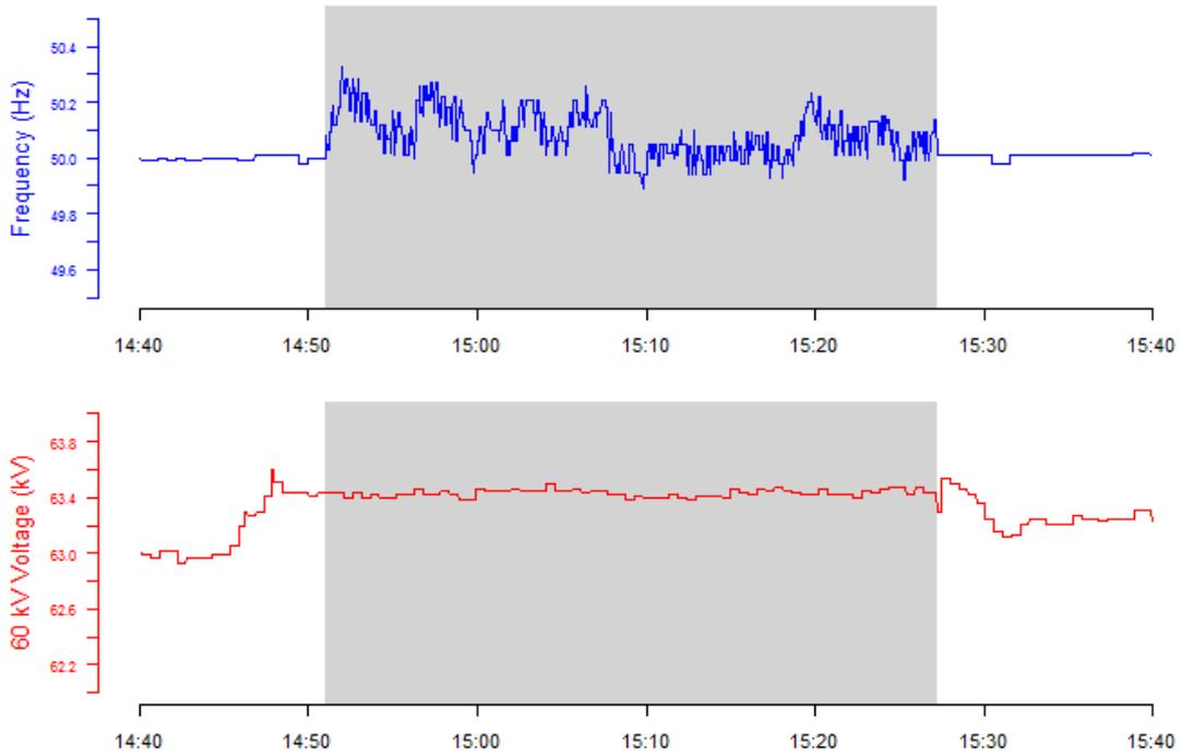
Figure 33 Cell Frequency and 60 kV Island Voltage Control as measured at the primary interconnect at Holsted. The region shaded grey indicates the time when the primary interconnect was open.
