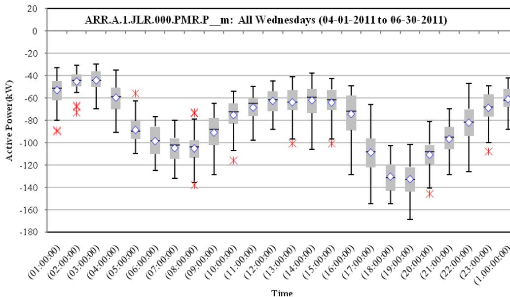
Figure 19 Load as a Function of Hour of Day for a Residential Feeder. The boxplots summarise the quantiles of the observed load (kW), by hour of the day, for all Wednesdays between 2011-04-01 and 2011-06-30; the grey boxes capture the middle 50%; outliers are indicated by red stars.
