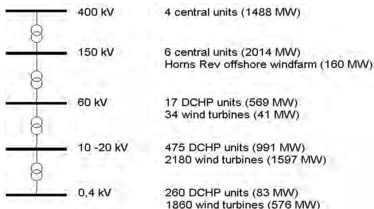
Figure 3 Production capacity per voltage level in the western part of Denmark in 2004.
