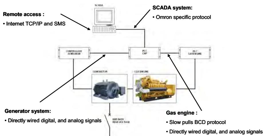
Figure 8 Typical existing communication system loop of a gas engine CHP unit designed for parallel operation with the grid. Exhaust boiler system not shown.
