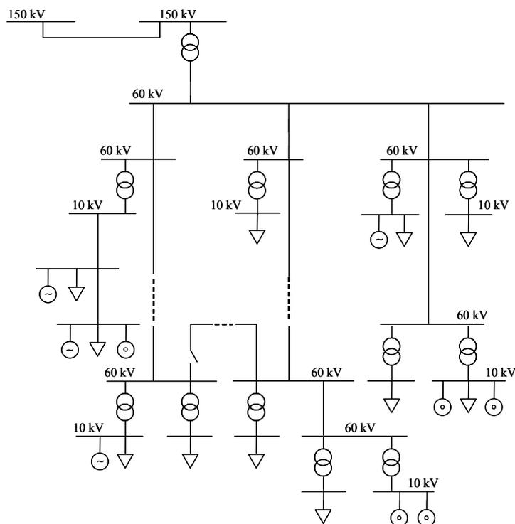
Figure 5 Simplified section of typical 60 kV distribution grid with DCHP plants (synchronous generators), WTs (induction generators) and 10 kV load feeders indicated.
