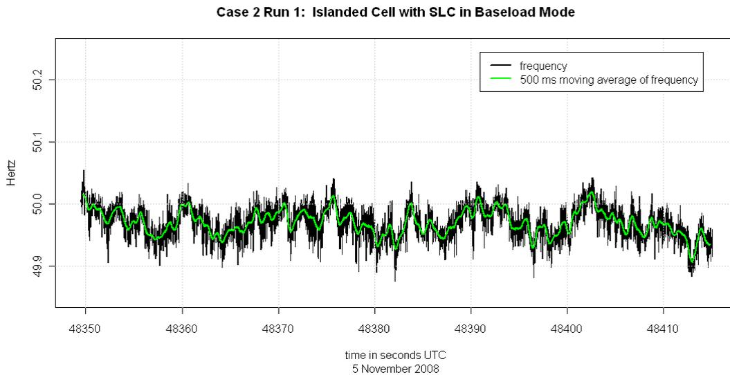
Figure 24 *Islanded Cell with SLC in Baseload Mode – Frequency Signal. One minute "snapshot" of the entire trace collected during testing. The black trace plots the metered high speed data and the green trace plots the 50 ms moving average. The periodicity observed when the SLC was offline is significantly reduced.*
