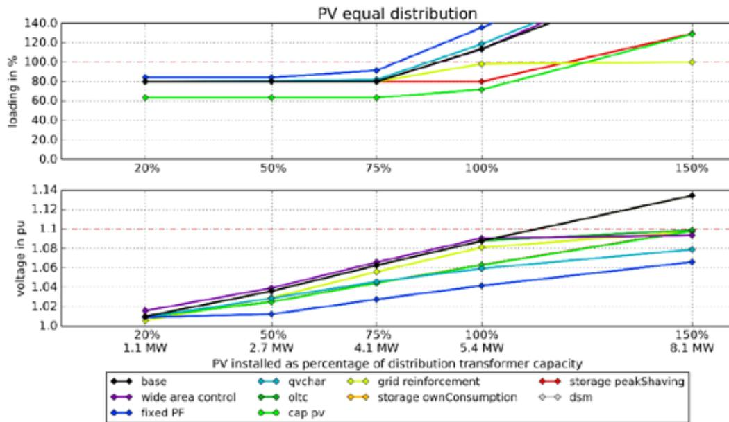
**Figure 59: Simulation results for urban feeder with LV network and equal PV distribution.**
