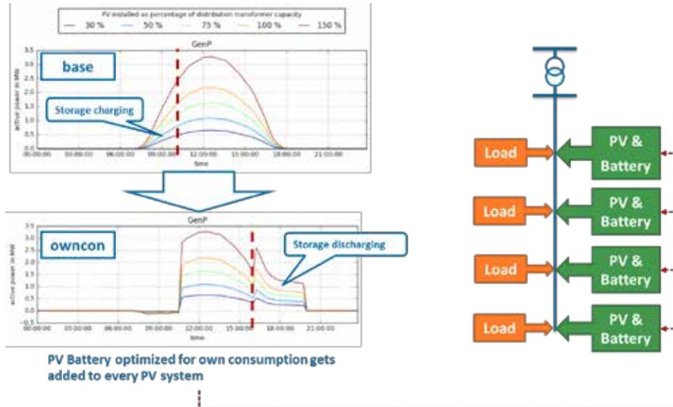
**Figure 54: PV Battery implementation with own consumption optimization**
