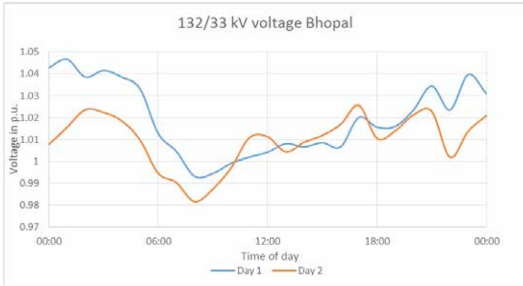
**Figure 37: Voltage measurements in 132/33 kV substation in Bhopal across two days.**
