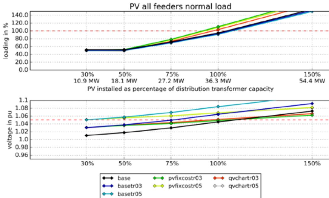
**Figure 42: Maximum asset loading and voltage at different penetrations of rooftop PV, as percentage of distribution transformer capacity.**
