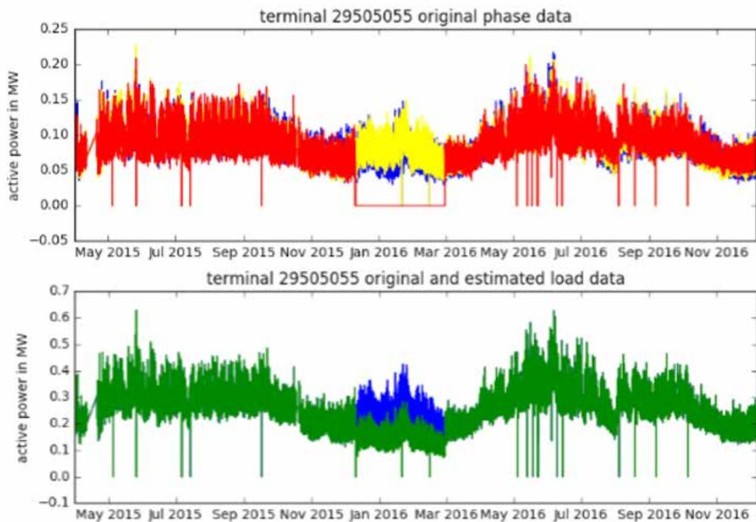
**Figure 26: Load data of a 630 kVA transformer in urban Delhi. Power per phase (upper figure) with one phase clearly missing for two months, calculated (green) and corrected (blue) total power (lower figure.) Total data gap for a week to the left of the figure is filled in by linear interpolation.**
