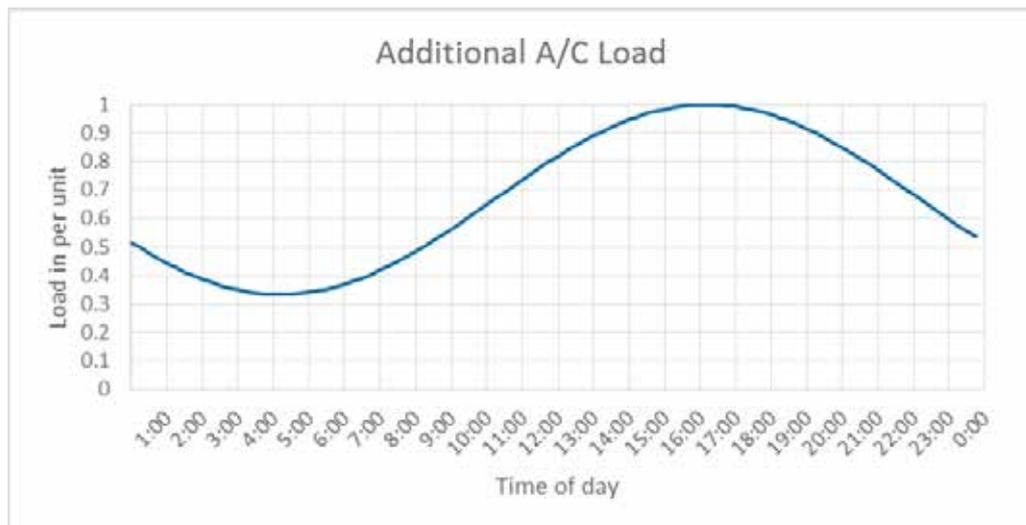
**Figure 49: Synthetic A/C load profile**
