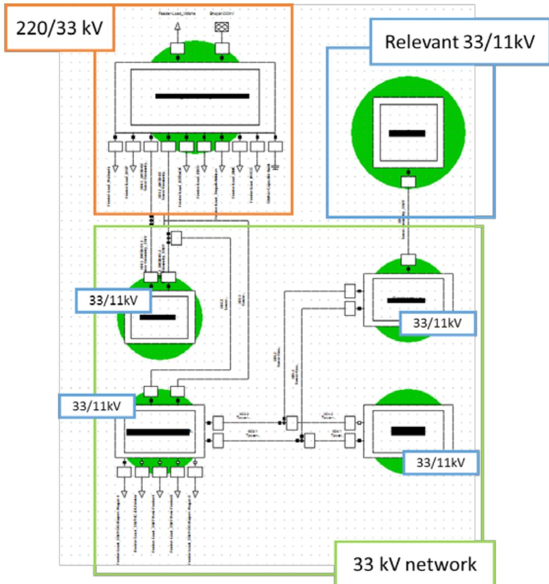
Figure 21: Upstream network structure (PowerFactory SLD.)
