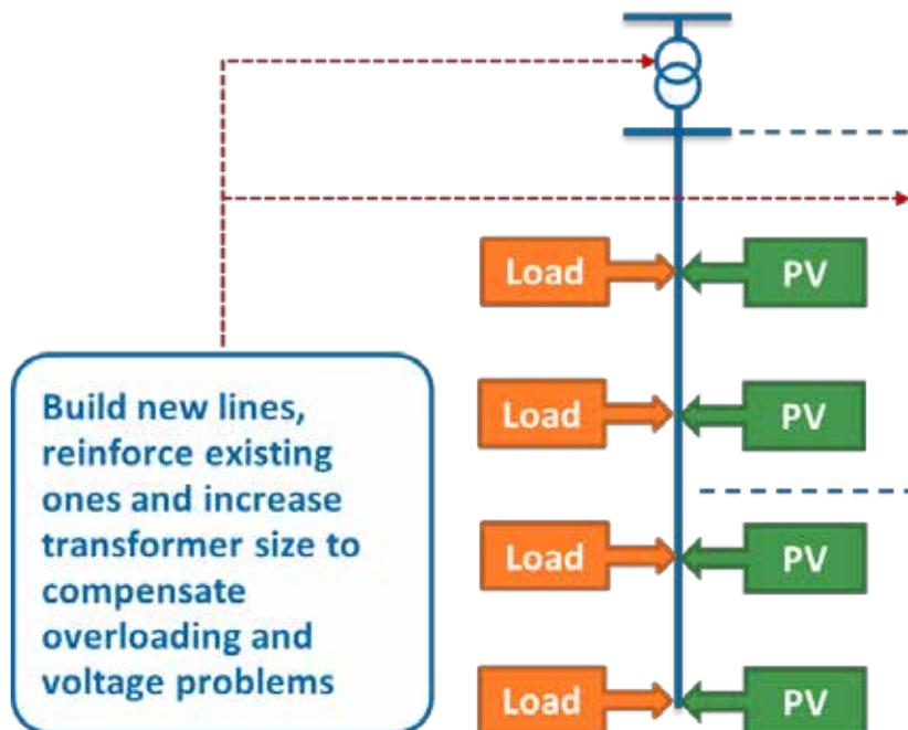
Figure 57: Network Reinforcement
