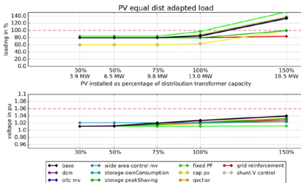
**Figure 71: Simulation results for the urban feeder in Bhopal with rooftop photovoltaic plants equally distributed along the feeder with adapted load considered**
