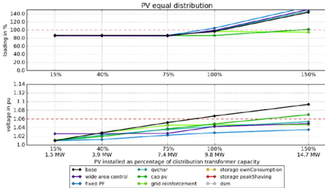
**Figure 66: Simulation results of the rural feeder with two parallel MV feeders and equal PV distribution.**
