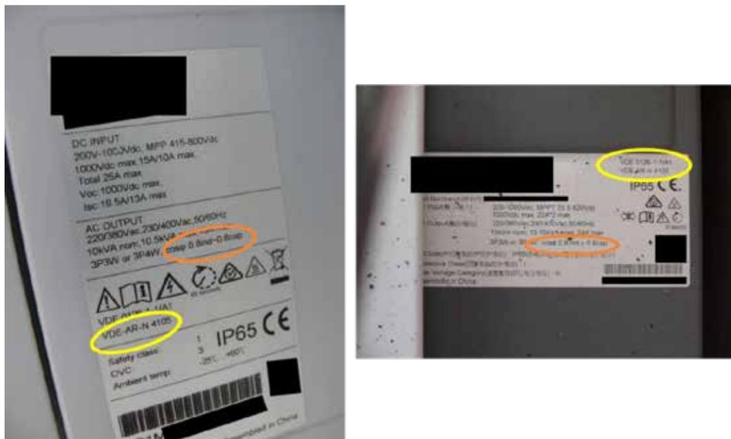
**Figure 38: Nameplates of PV inverters in Bhopal (left) and Delhi (right.) Reactive power range is marked in orange, statement of compliance with the German low voltage grid code in yellow. Serial numbers etc. have been obscured.**
