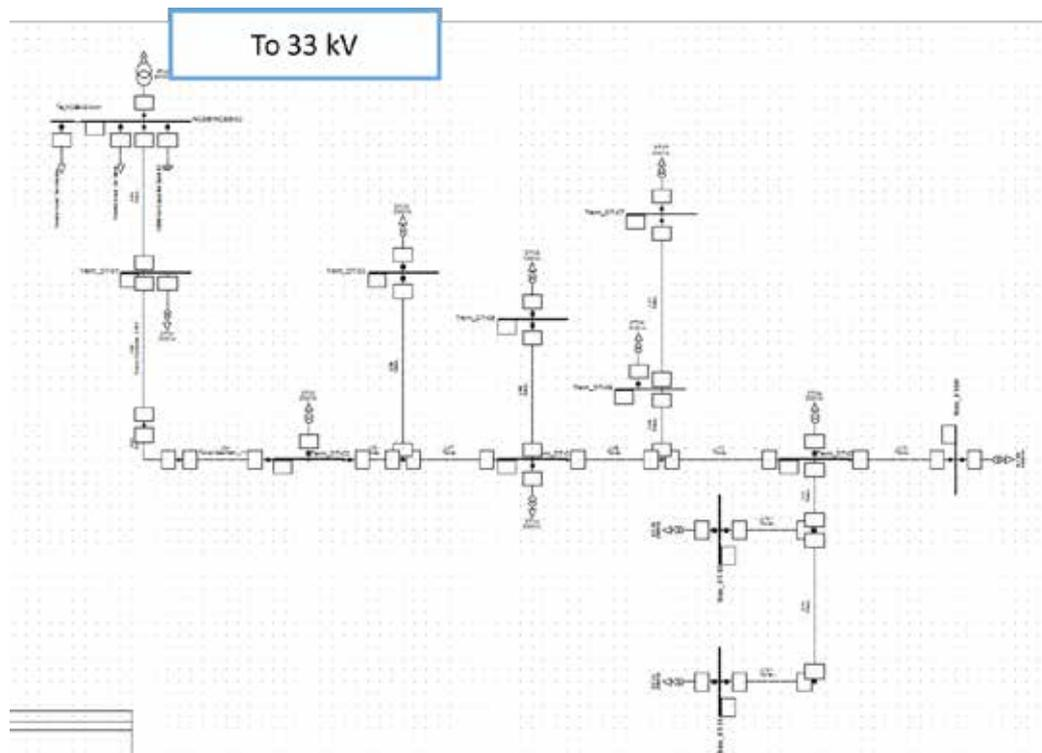
Figure 22: PowerFactory SLD of Bhopal rural 11 kV feeder.
