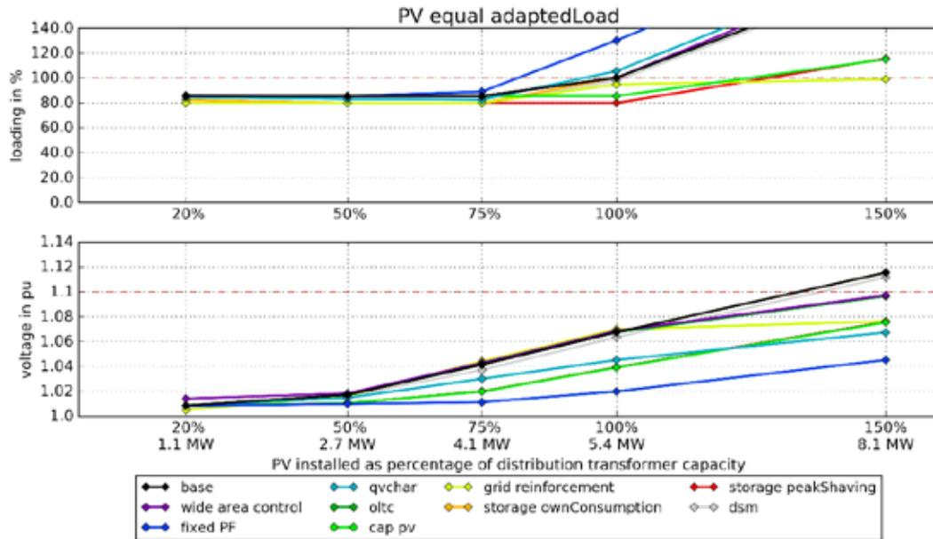
**Figure 60: Simulation results for urban feeder with LV network and equal PV distribution with adapted load.**
