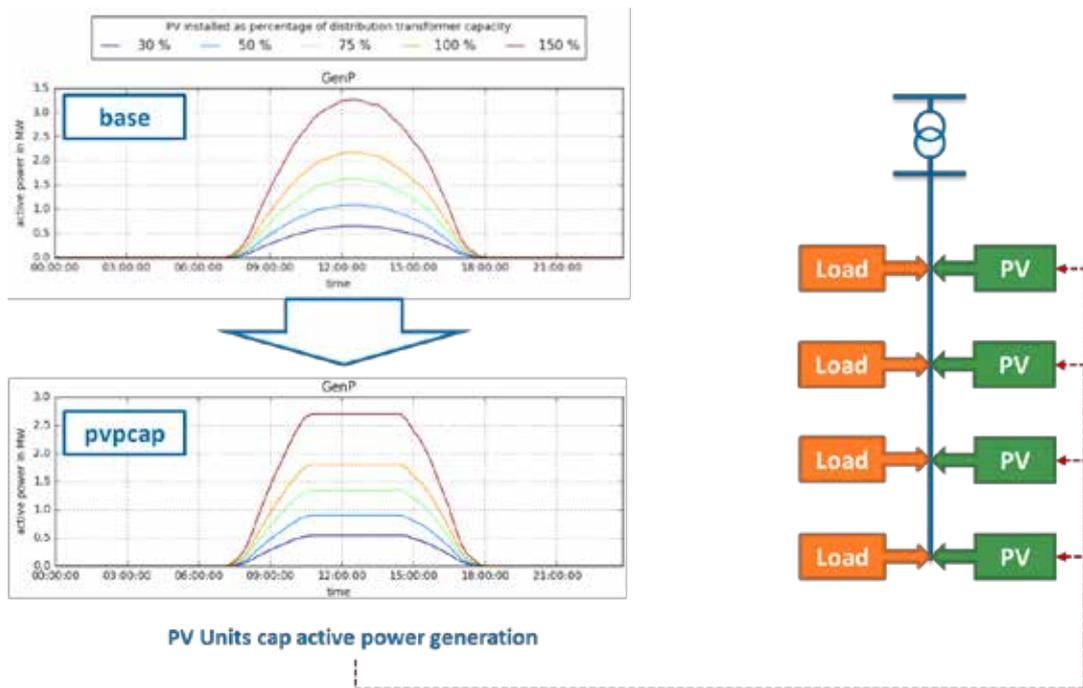
Figure 53: Capping of Photovoltaic plants peak power
