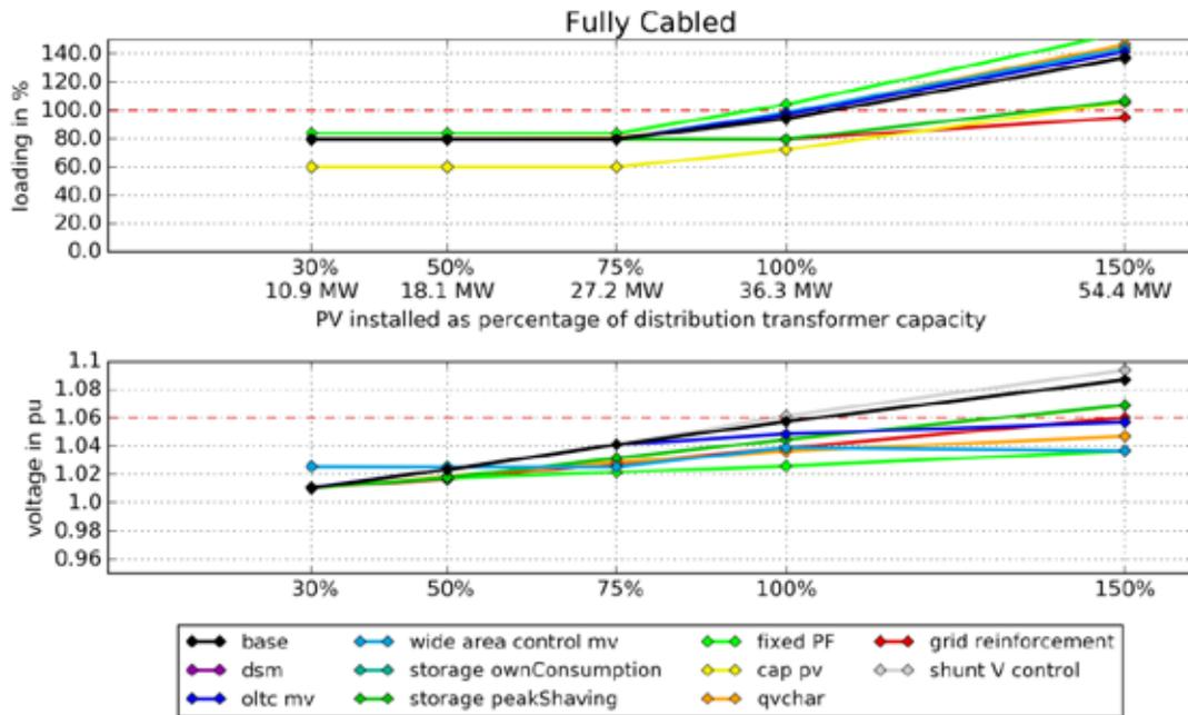
Figure 83: Simulation results for the rural feeder in Bhopal with rooftop photovoltaic plants equally distributed along the feeder with overhead lines replaced with cables considered
