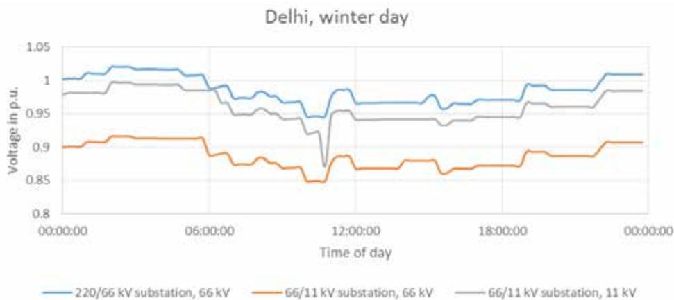
**Figure 33: Voltage measurements of 66 and 11 kV level grids in urban Delhi, winter day. No switching.**
