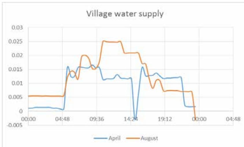
**Figure 31: Load data for a transformer supplying a water supply station on a rural feeder for a day in April and one in August.**
