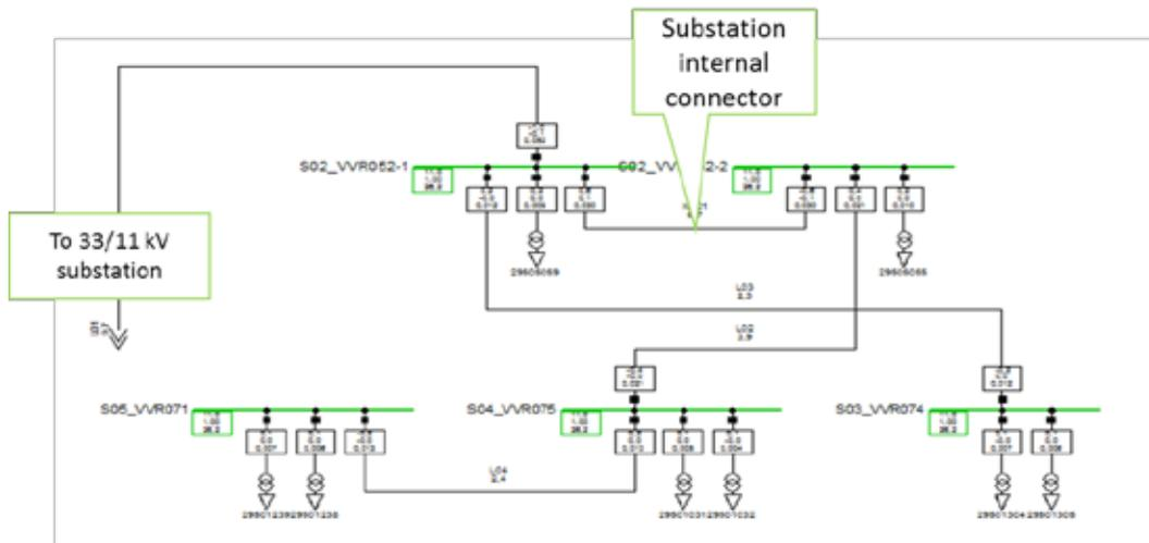
Figure 19: PowerFactory SLD of 11 kV feeder.
