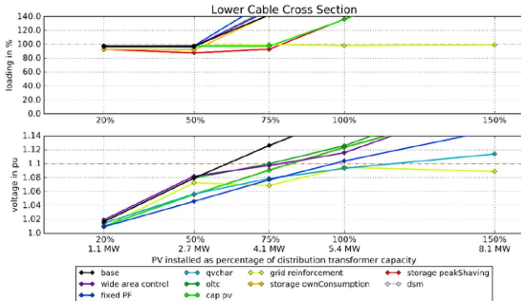
Figure 63: Simulation results for urban feeder with LV network and PV at the end of the feeder with lower cable cross-section.
