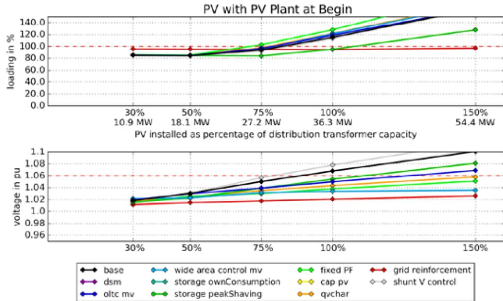
**Figure 80: Simulation results for the rural feeder in Bhopal with rooftop photovoltaic plants equally distributed along the feeder with a utility scale solar plant of 2.5 MWp at the beginning of the feeder considered.**
