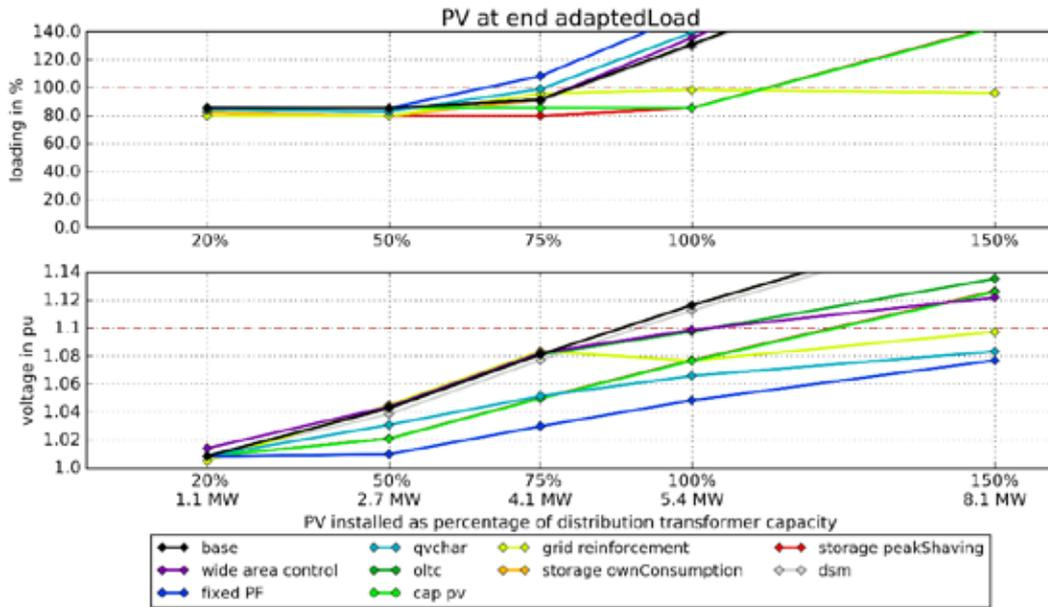
**Figure 62: Simulation results for urban feeder with LV network and PV at the end of the feeder with adapted load.**
