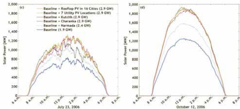
**Figure 17: PV power output calculated from measurements of solar irradiation in Gujarat, 2006, monsoon season and dry season. [64]**
