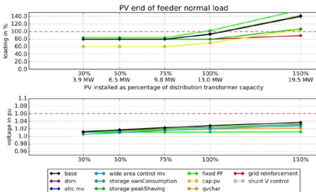
**Figure 72: Simulation results for the urban feeder in Bhopal with rooftop photovoltaic plants higher at the end of the feeder with normal load considered**
