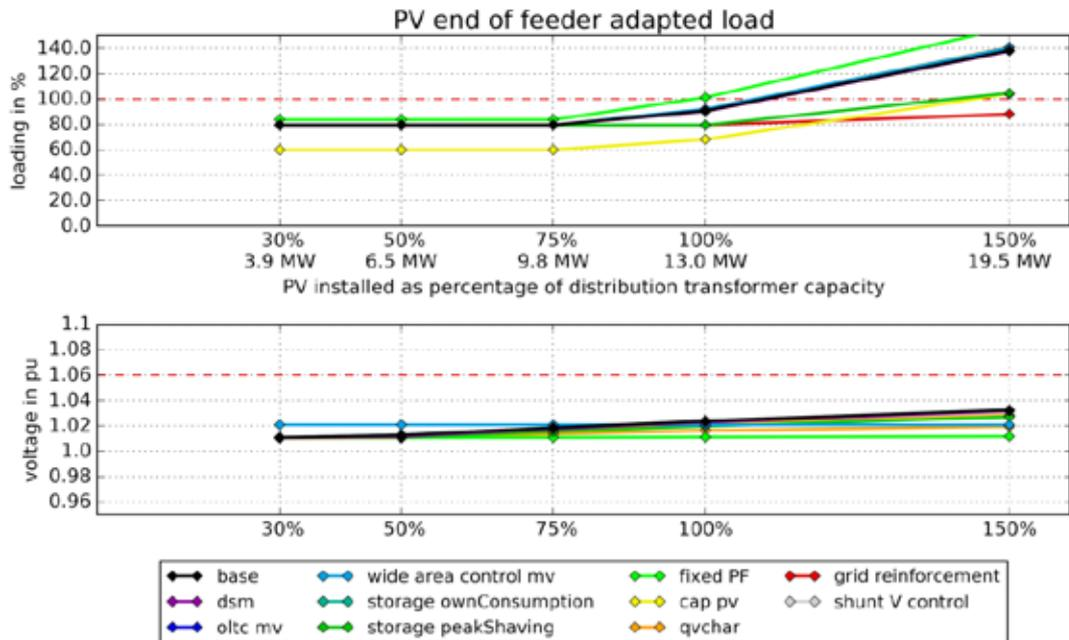
Figure 73: Simulation results for the urban feeder in Bhopal with rooftop photovoltaic plants higher at the end of the feeder with adapted load considered.
