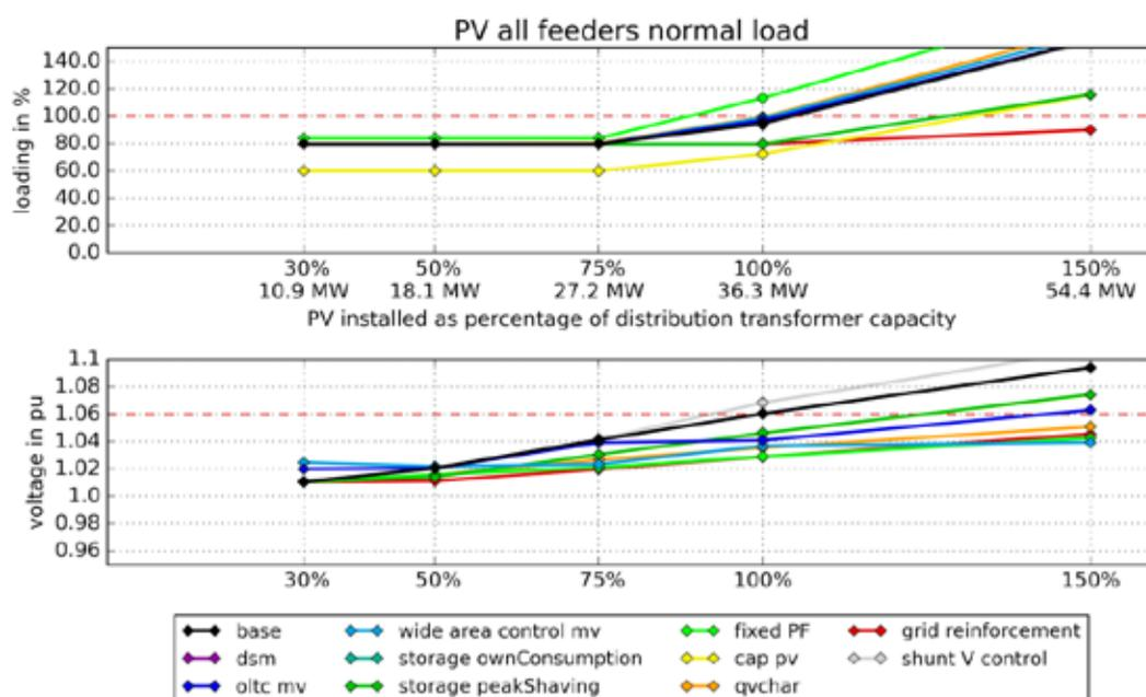
**Figure 75: Simulation results for the rural feeder in Bhopal with rooftop photovoltaic plants equally distributed along the feeder with normal load considered**
