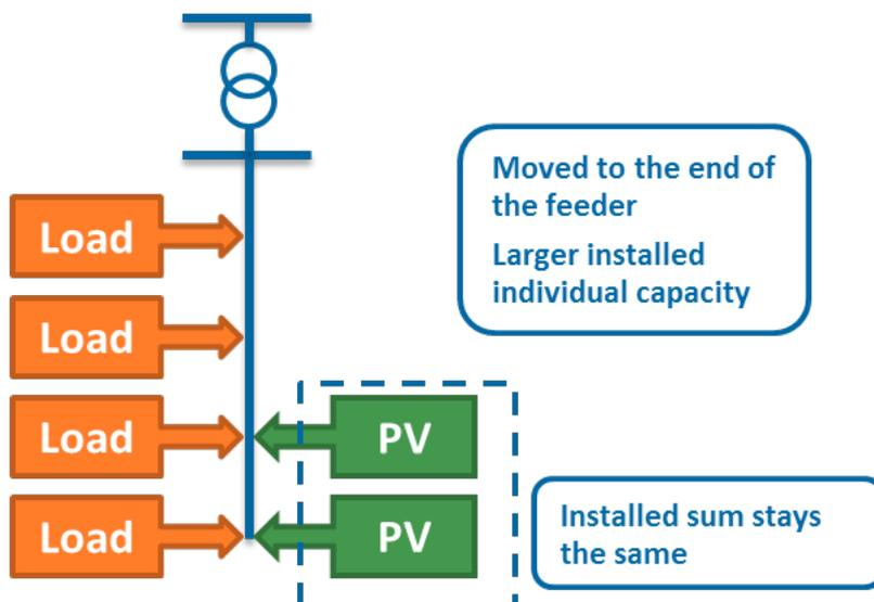
Figure 45: Rooftop photovoltaic plants concentrated at the end of the feeder
