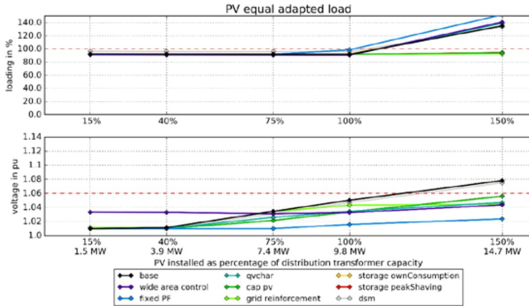
**Figure 67: Simulation results of the rural feeder with two parallel MV feeders and equal PV distribution with adapted load.**
