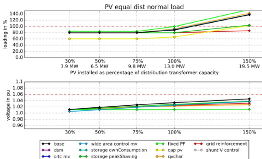
**Figure 70: Simulation results for the urban feeder in Bhopal with rooftop photovoltaic plants equally distributed along the feeder with normal load considered**
