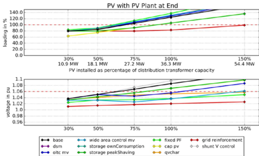
Figure 79: Impact of reactive power injection through the utility scale solar power plant at the end of the feeder
