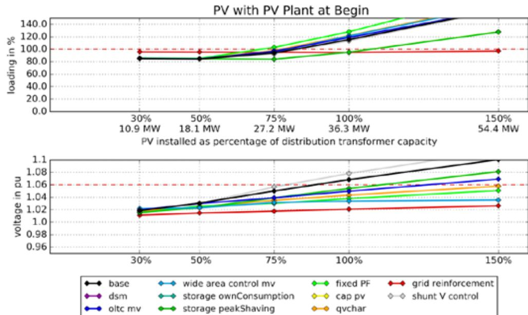
Figure 77: Impact of reactive power injection through the utility scale solar plant at the beginning of the feeder
