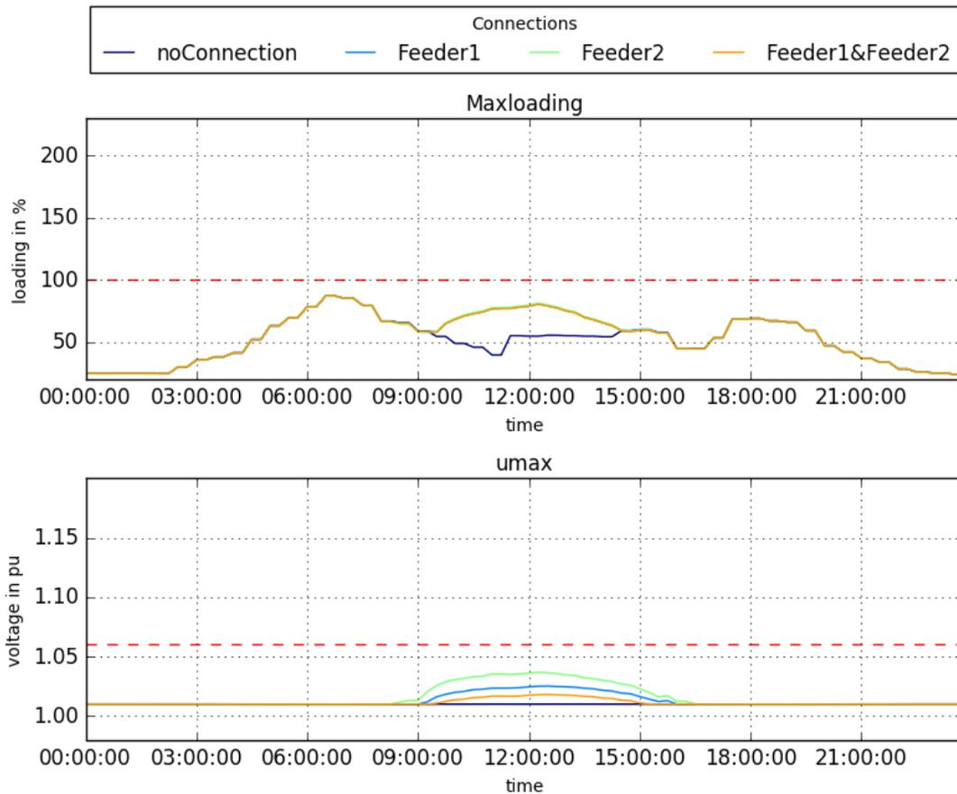
**Figure 65: Simulation results of the rural feeder with two parallel MV feeders and a 3.5 MW power plant with different connection schemes and Q-V-characteristic enabled.**
