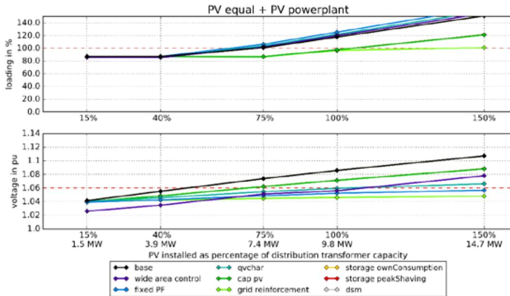
**Figure 68: Simulation results of the rural feeder with two parallel MV feeders and equal PV distribution with a 3.5 MW PV power plant.**
