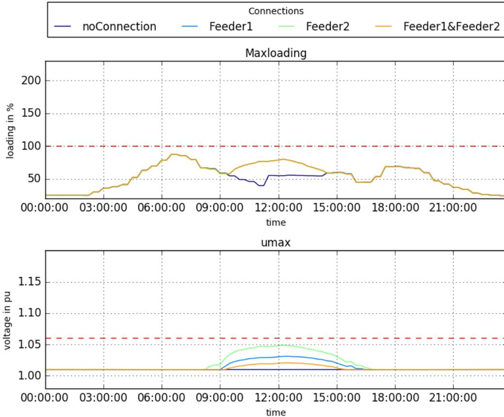
Figure 64: Simulation results of the rural feeder with two parallel MV feeders and a 3.5 MW power plant with different connection schemes.
