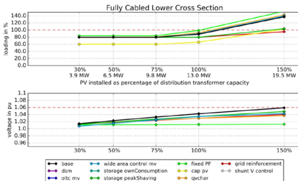
**Figure 74: Simulation results for the urban feeder in Bhopal with rooftop photovoltaic plants equally distributed along the feeder with lower cable cross-section considered.**
