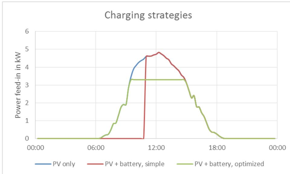
**Figure 7: Power fed back to the grid for different layouts. PV only (blue), PV with battery for self-consumption only (red) and PV with battery for self-consumption, optimized to shave the PV peak off.**
