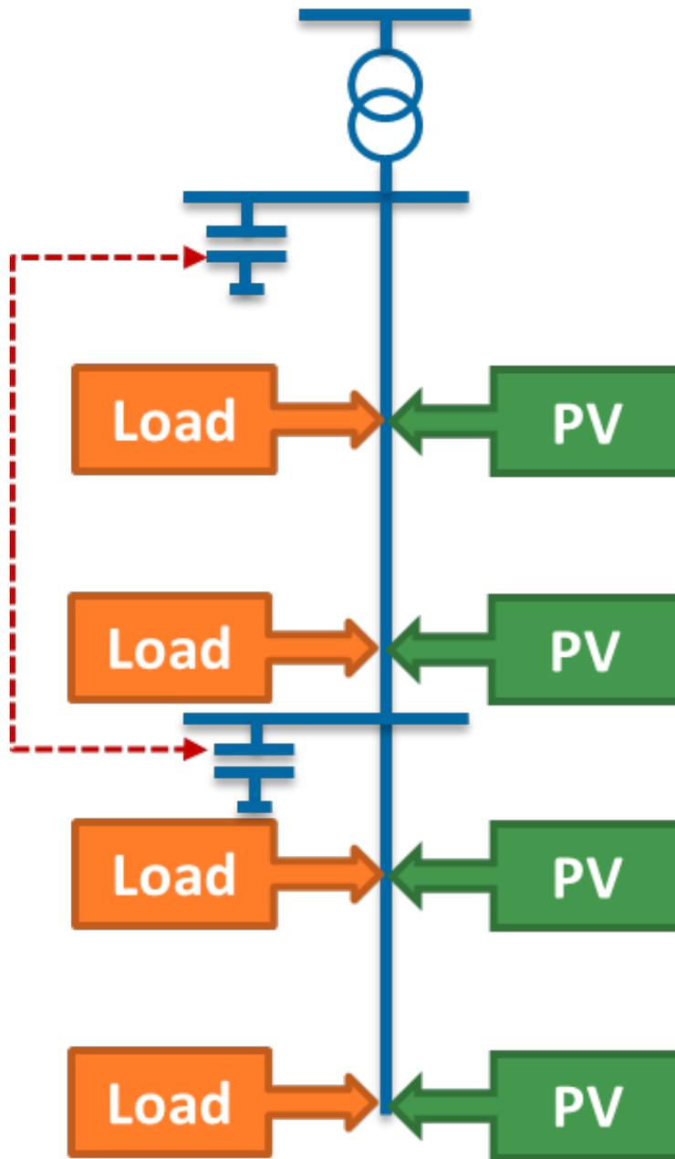
**Figure 51: Shunt Compensator for voltage control**
