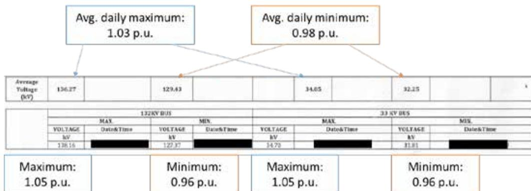
**Figure 36: Voltage measurements from Bhopal for one month, 132 and 33 kV, minima and maxima.**
