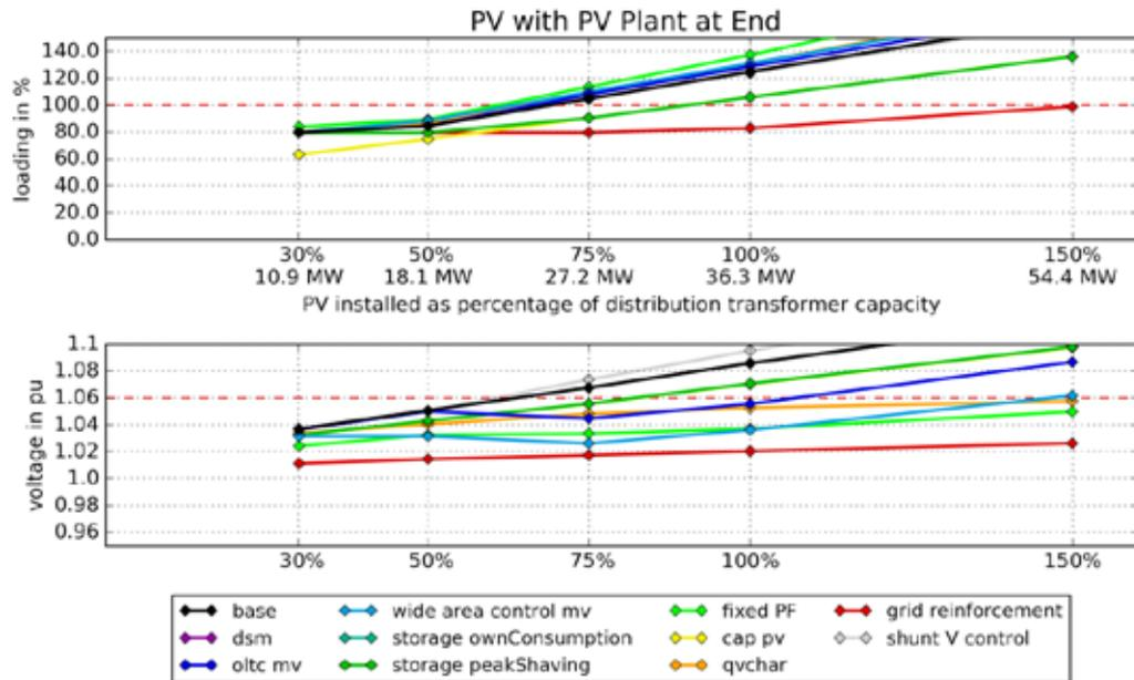
**Figure 82: Simulation results for the rural feeder in Bhopal with rooftop photovoltaic plants equally distributed along the feeder with a utility scale solar plant of 2.5 MWp at the end of the feeder considered**
