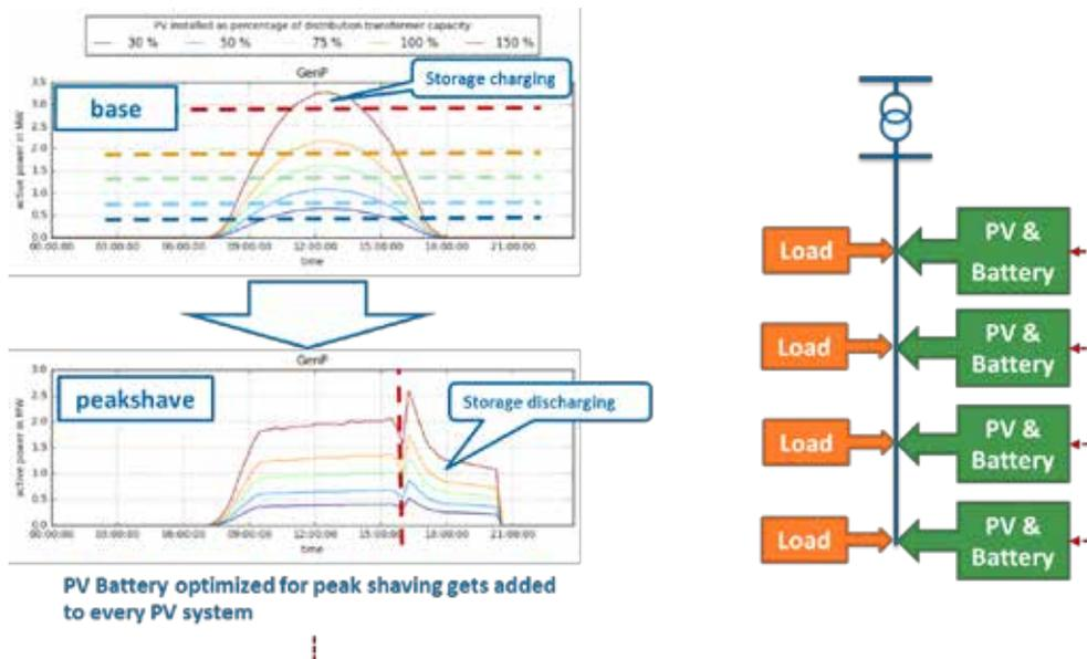
**Figure 55: PV Battery implemented with peak shaving optimization**
