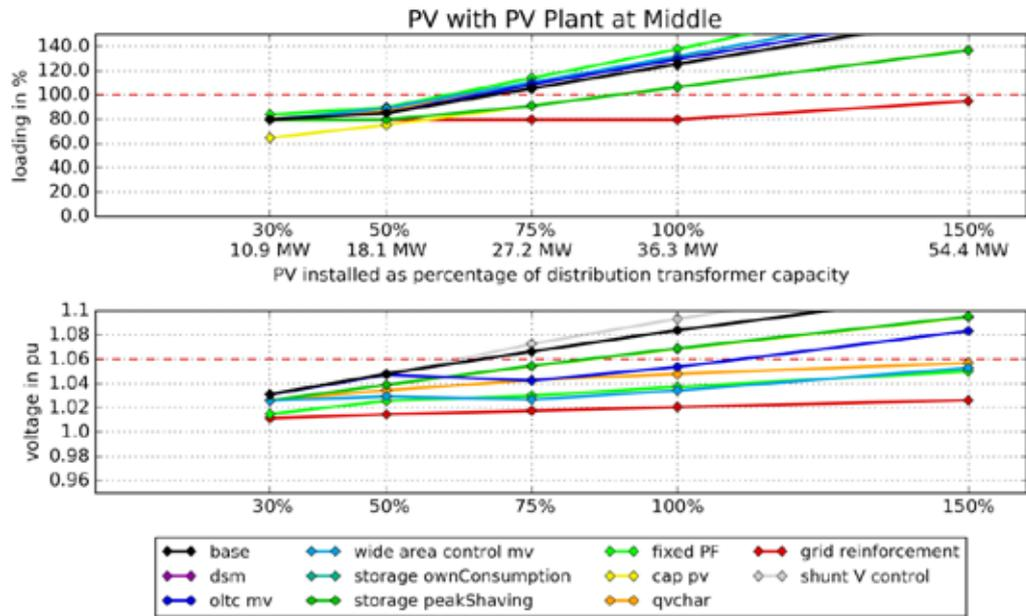
**Figure 81: Simulation results for the rural feeder in Bhopal with rooftop photovoltaic plants equally distributed along the feeder with a utility scale solar plant of 2.5 MWp at the middle of the feeder considered**
