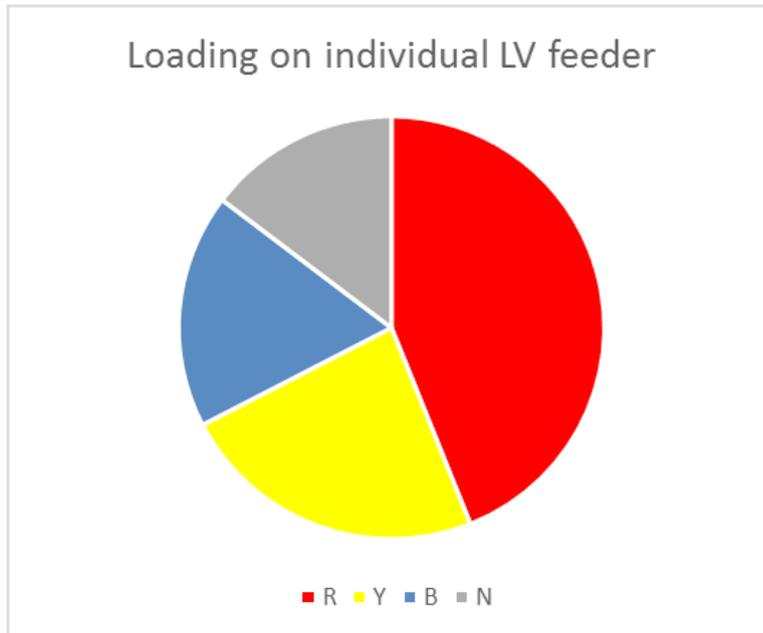
**Figure 20: Loading per conductor (red, yellow, blue are phase conductors, N/grey is neutral) of sample LV feeder, showing highly asymmetrical load.**
