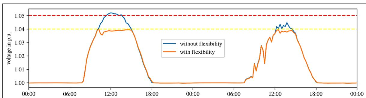
Figure 7: Voltage profile with and without flexibility provided for two days in March
