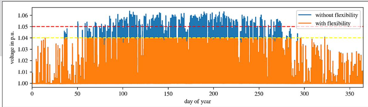
Figure 8: Voltage profile with and without flexibility provided for the entire year
