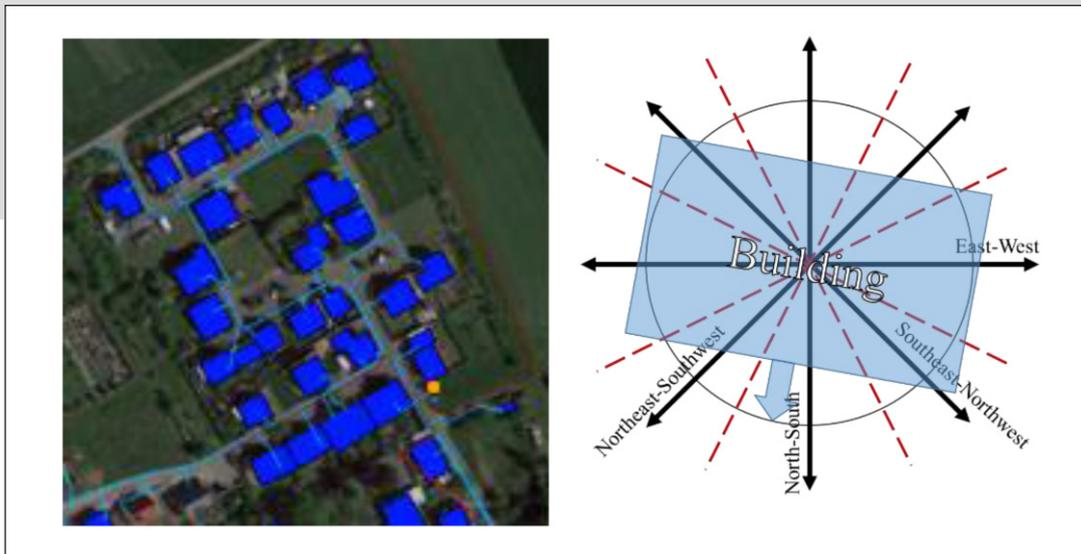
Figure 1: Analysis of rooftop PV potential by GIS data analysis (top) and categorization according to orientation (bottom)
