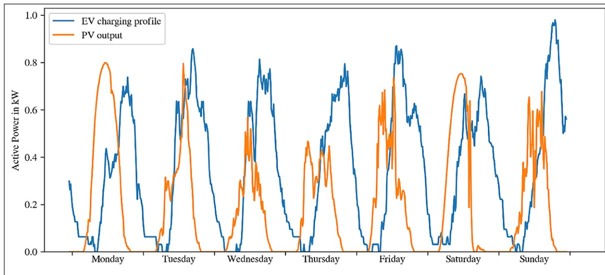
Figure 3: Normalized EV charging profile per EV in blue, normalized PV profile per kWp PV output in orange, both for a summer week
