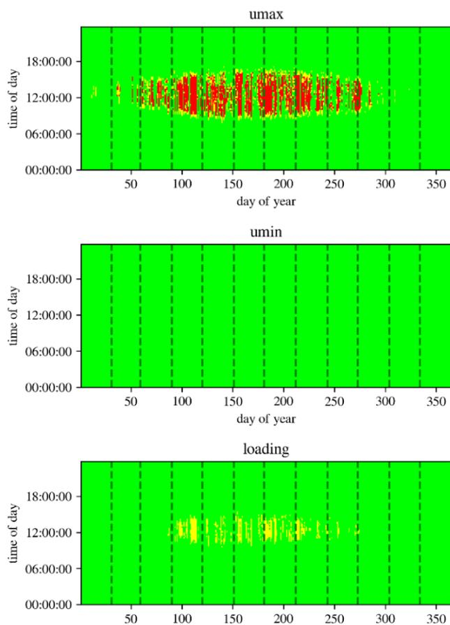
Figure 4: Categorization of maximum and minimum voltage as well as loading into green, amber and red phase of the BDEW traffic light system for the 2030 scenario
