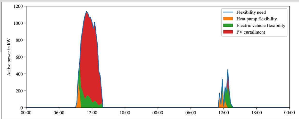
Figure 6: Flexibility activation of heat pumps, electric vehicles and PV curtailment for two days in March
