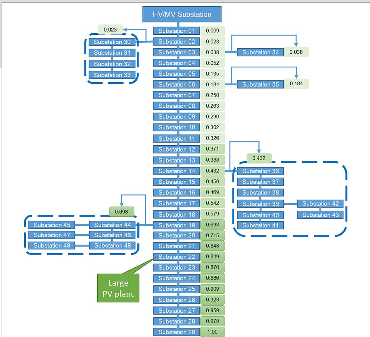
Figure 5: Determination of voltage sensitivities for each substation
