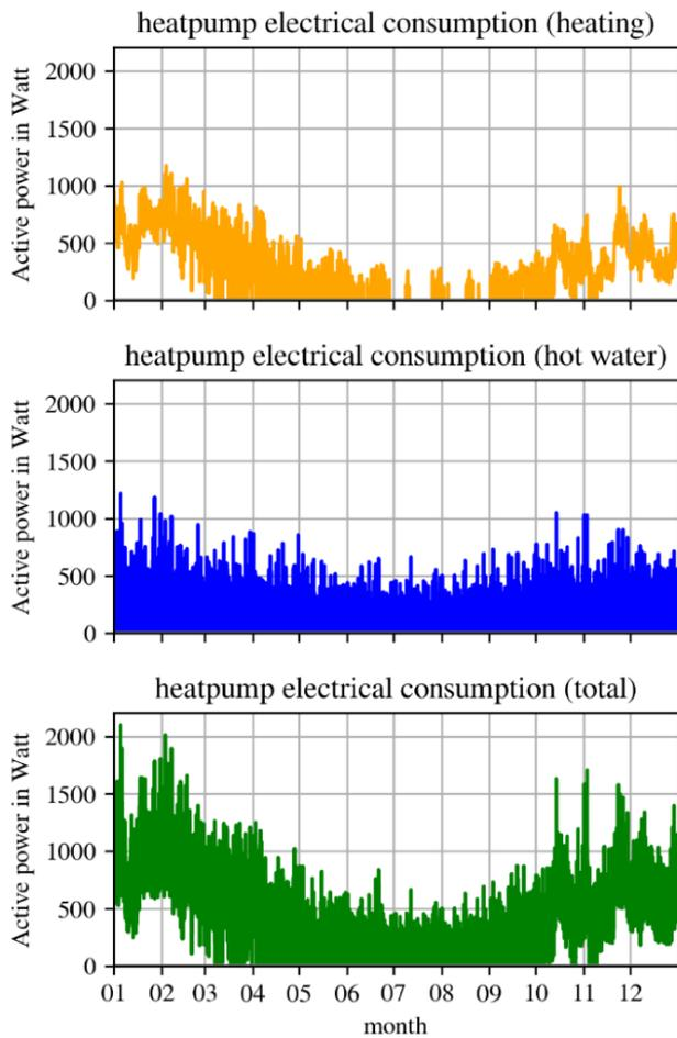
Figure 2: Electrical demand of the heat pump for heating, hot water and in total
