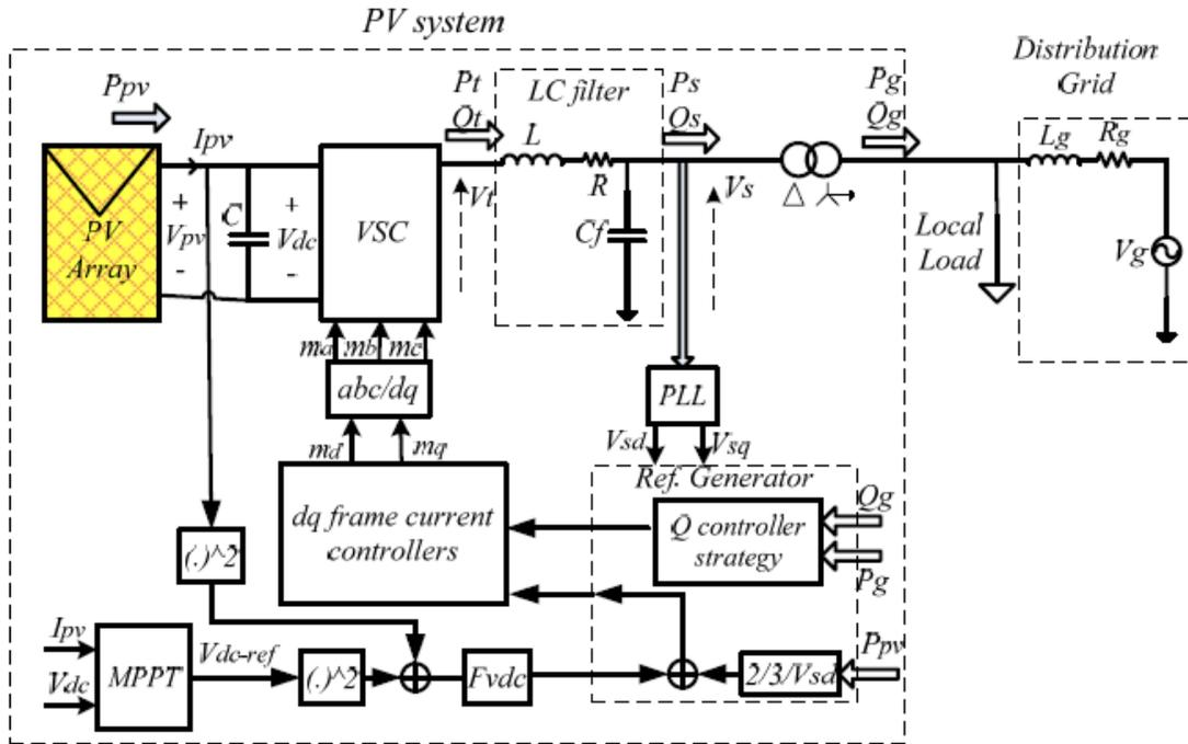
Fig. 3.8 Schematic diagram of the PV system connected to a distribution grid [14]
