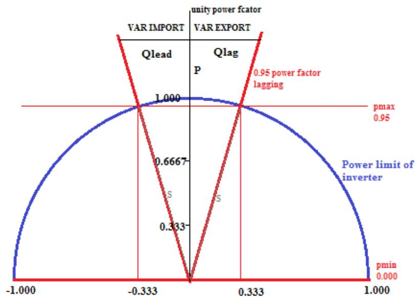
Fig 3.5 Capability curve of the inverter
