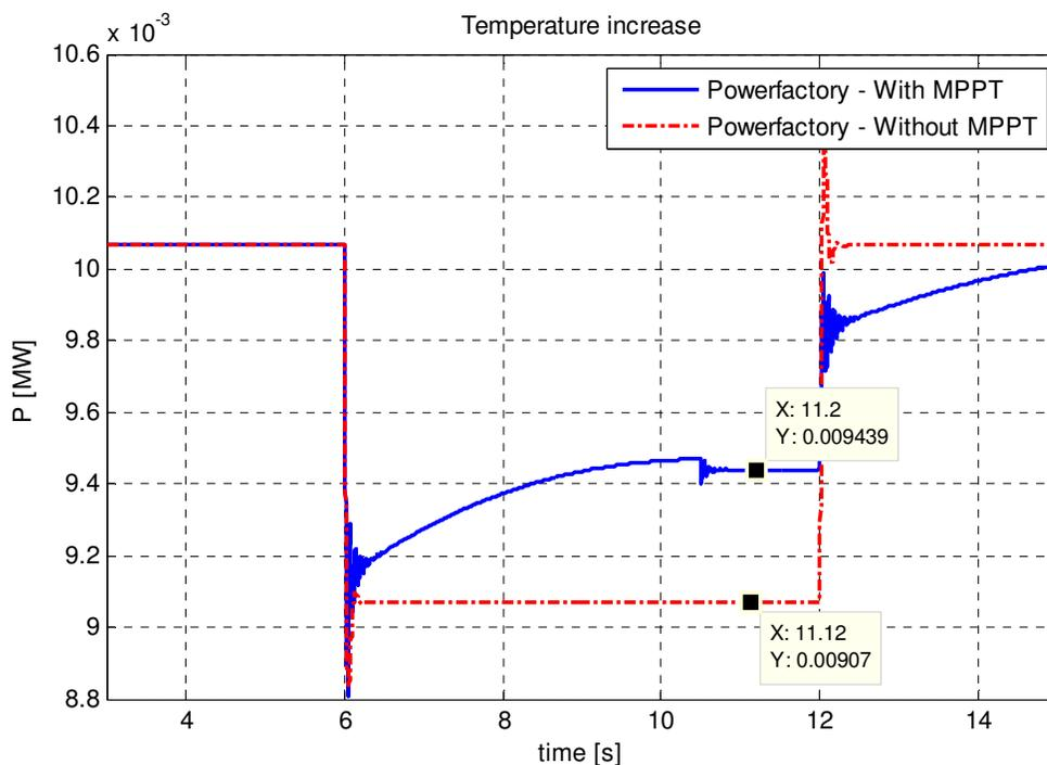
Fig. 5.33 Active power of the PV system
