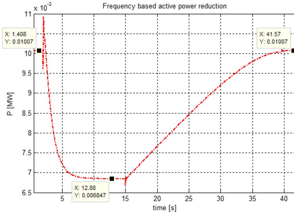
Fig. 5.30 Active power of the PV system
