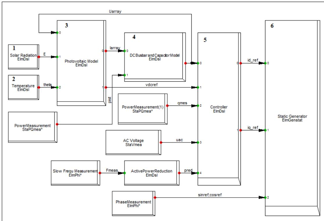
Fig 3.6 Control frame of PV system
