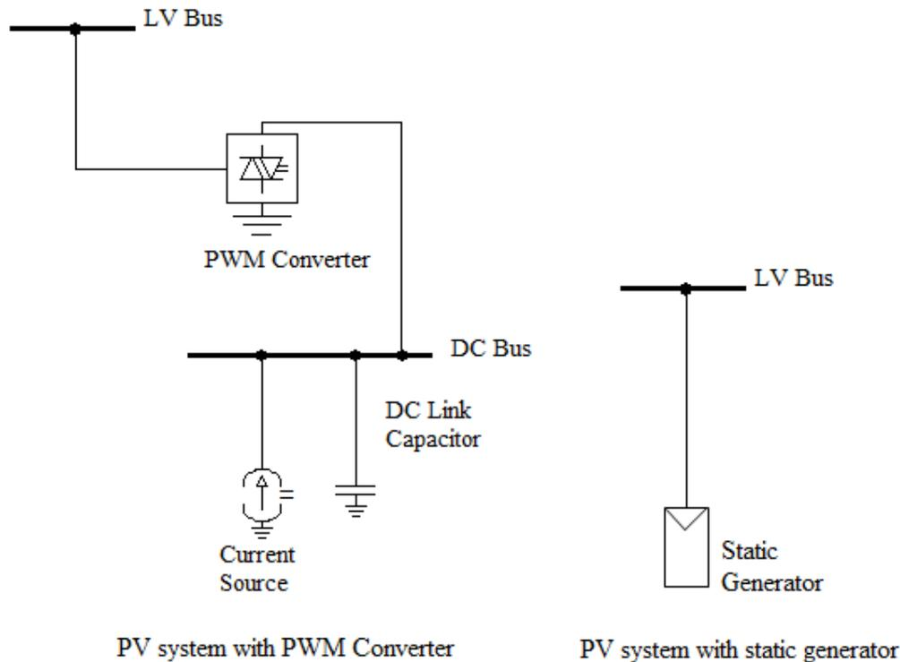
Fig. 3.2 Different PV system modeling in Power factory
