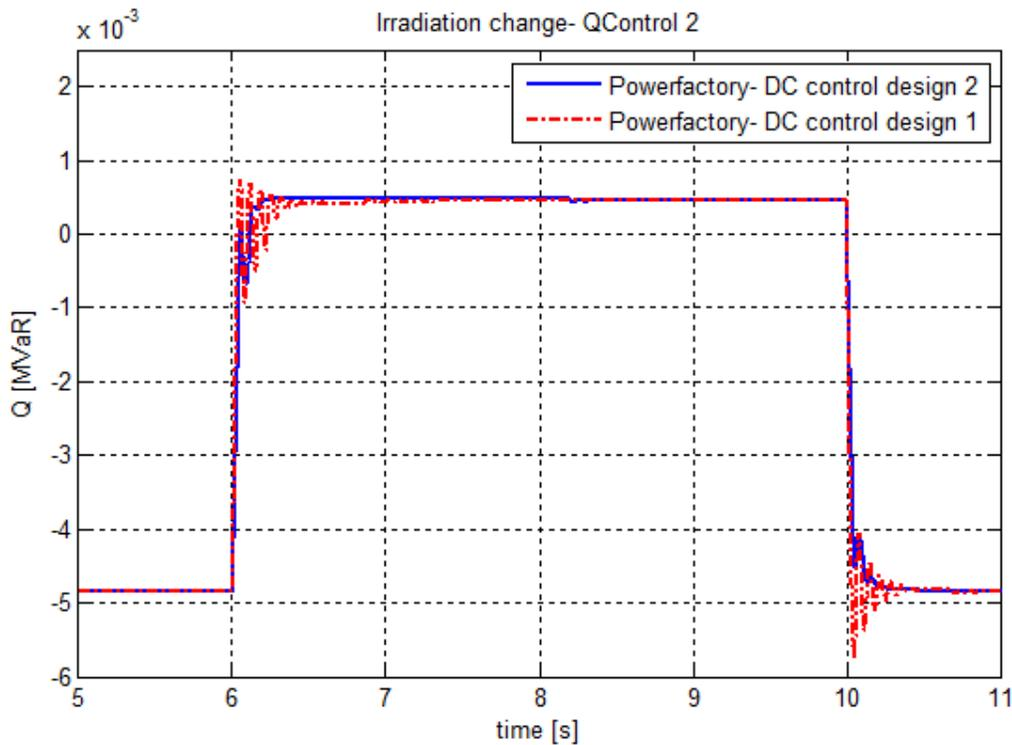
Fig. 5.40 Reactive power of the PV system
