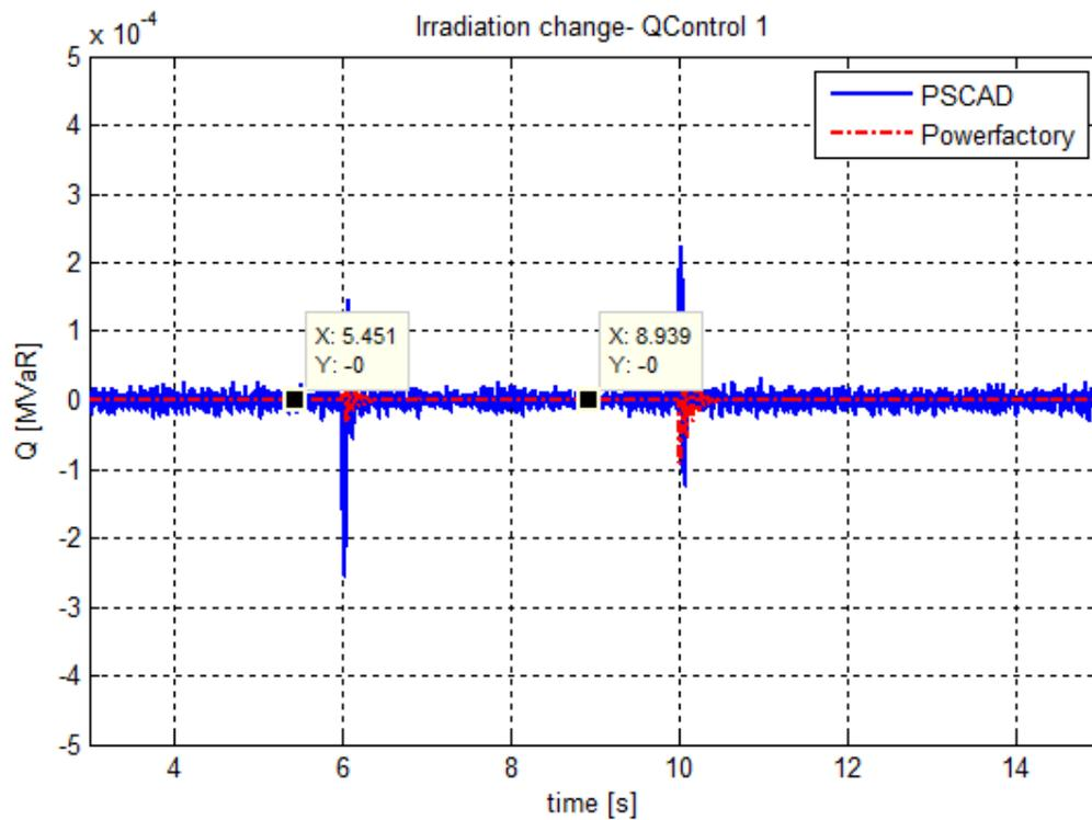
Fig. 5.7 Reactive power of the PV system
