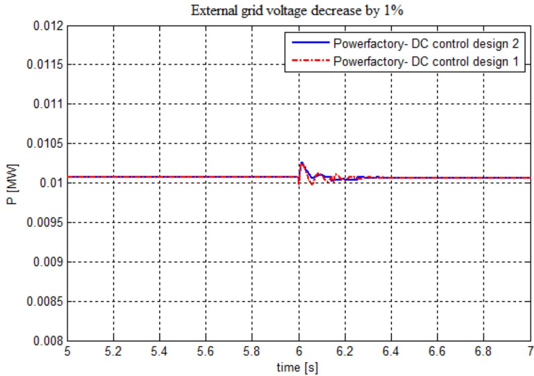
Fig. 8.8 Active power of the PV system
