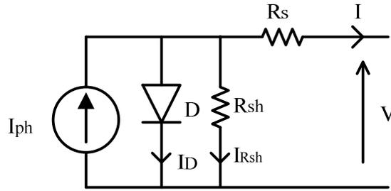
Fig. 2.2 Single diode equivalent circuit of a photovoltaic cell [4]
