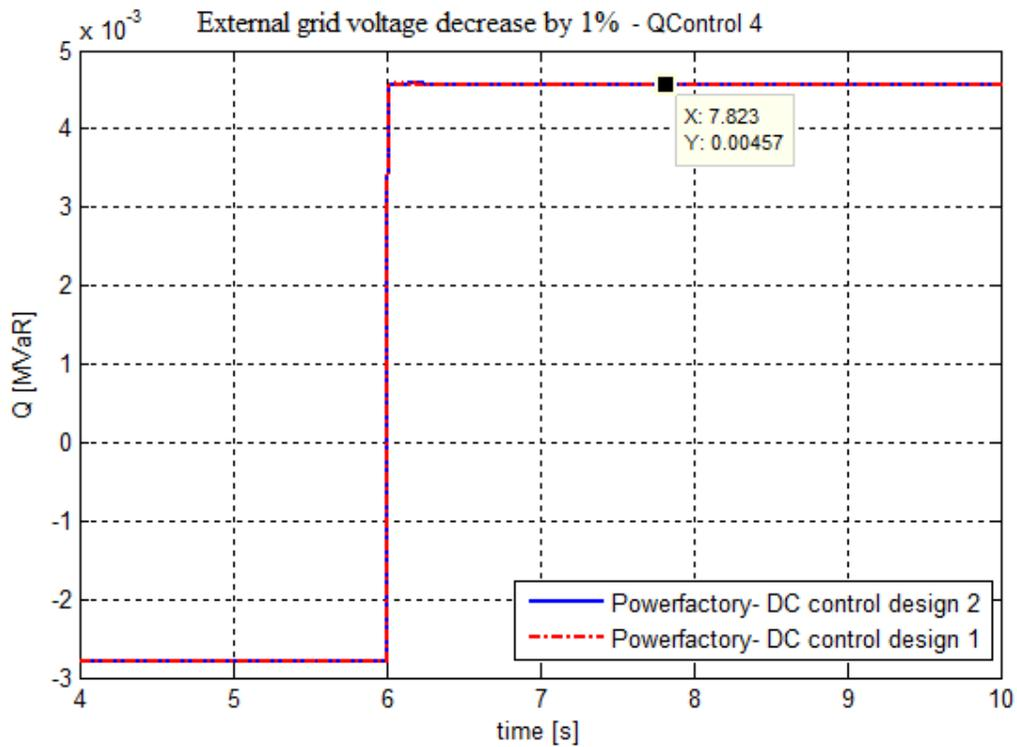
Fig. 8.9 Reactive power of the PV system
