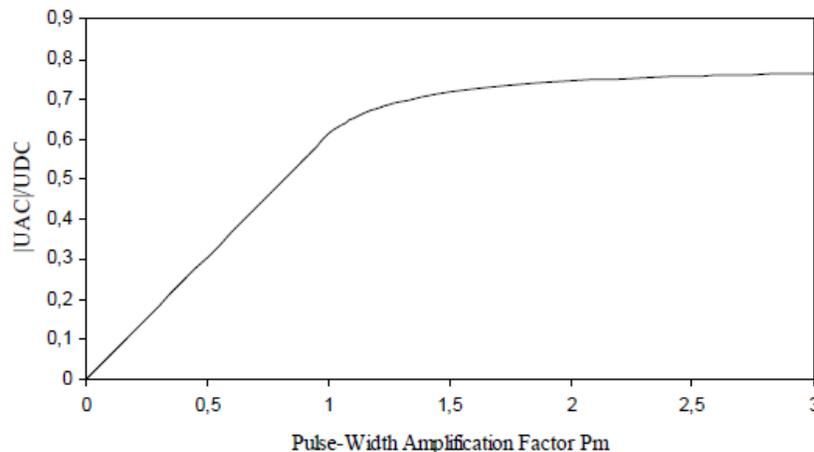
Fig. 4.3 PWM Converter characteristic [19]
