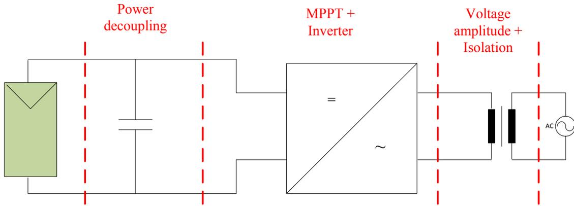
Fig. 2.6 Conventional transformer isolation method [9]
