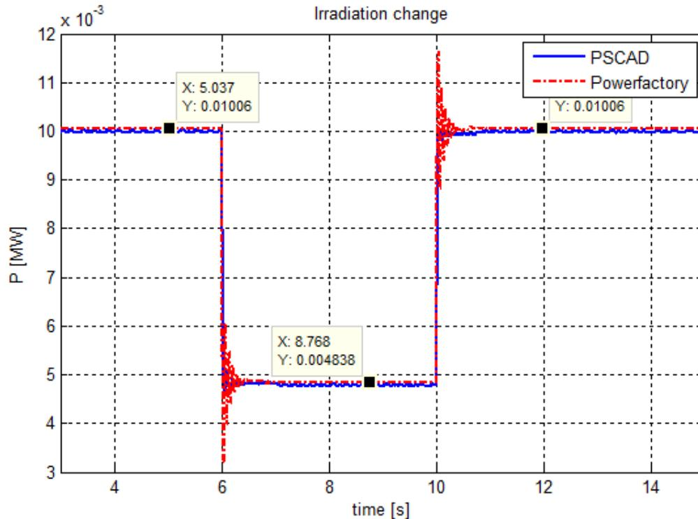
Fig. 5.4 Active power of the PV system
