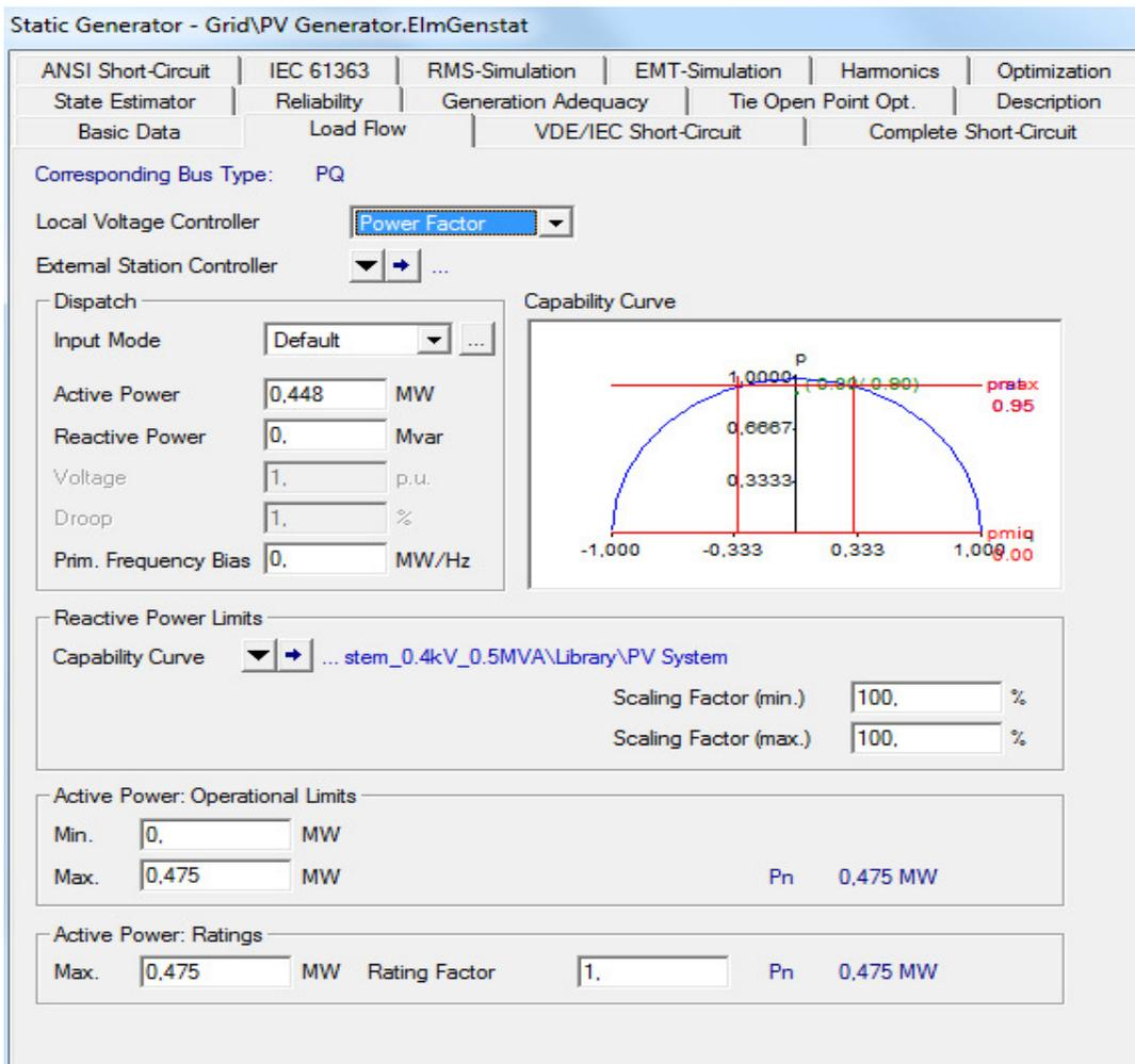
Fig 3.4 Static generator power flow under steady state conditions
