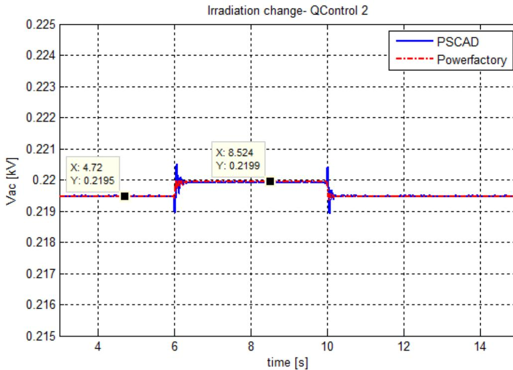
Fig. 5.12 AC voltage at L2 terminal
