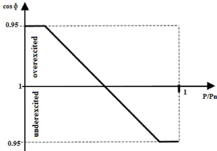
Fig. 2.13 Dynamic power factor operation characteristic [6]
