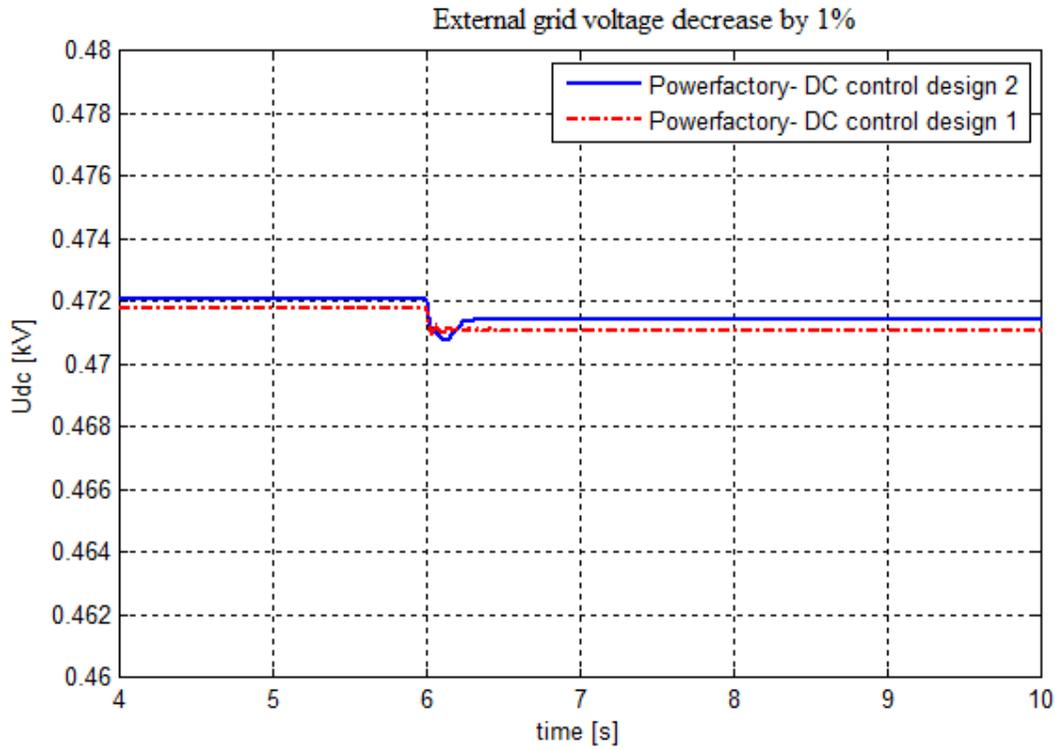
Fig. 8.7 DC voltage of PV system
