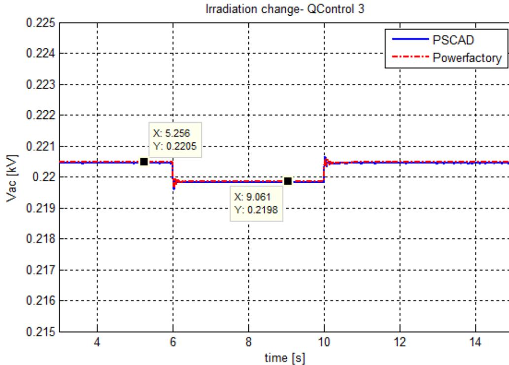
Fig. 5.14 AC voltage at terminal L2
