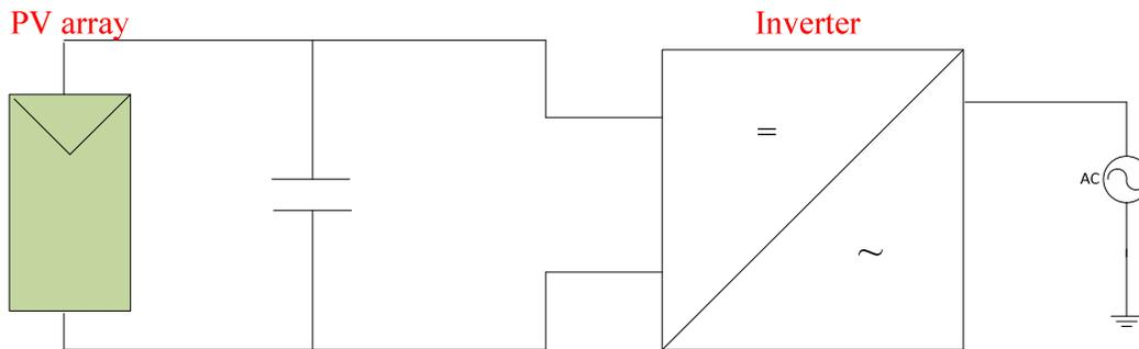
Fig. 3.1 Grid connected PV system model
