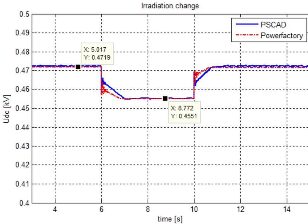
Fig. 5.3 DC voltage of the PV system
