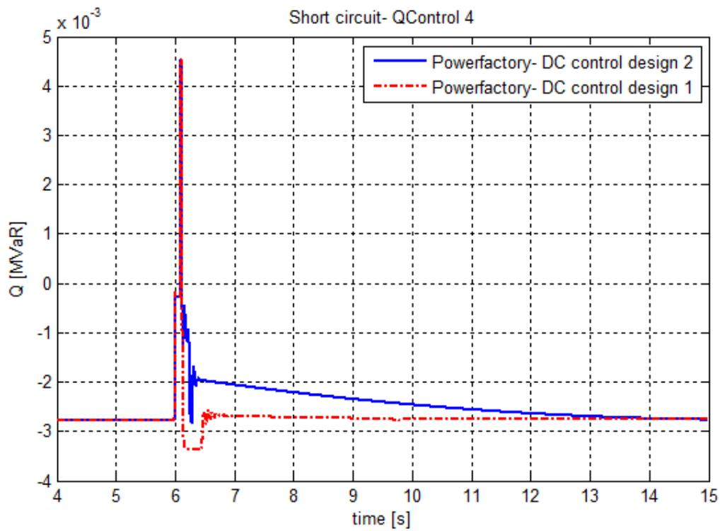
Fig. 8.14 Reactive power of the PV system
