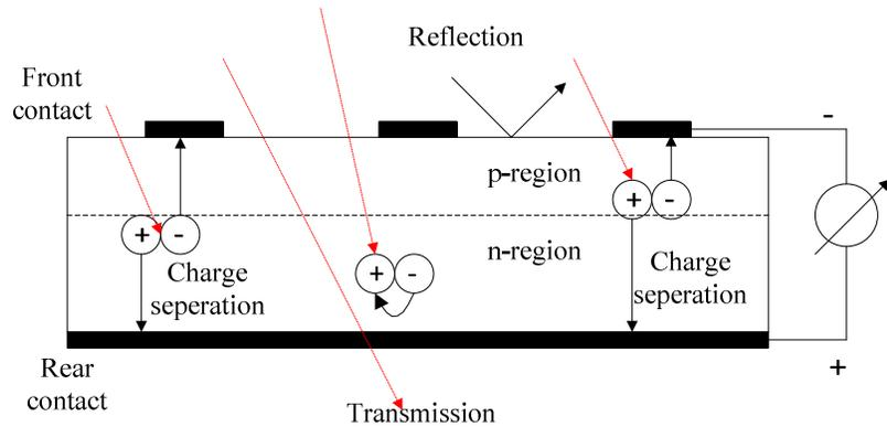
Fig. 2.1 Processes in an irradiated solar cell [3]
