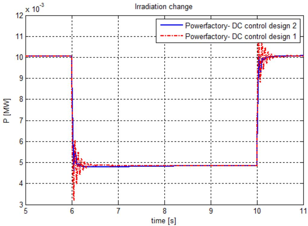
Fig. 5.39 Active power of the PV system
