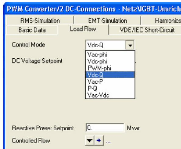
Fig. 4.4 Load Flow tab of PWM converter
