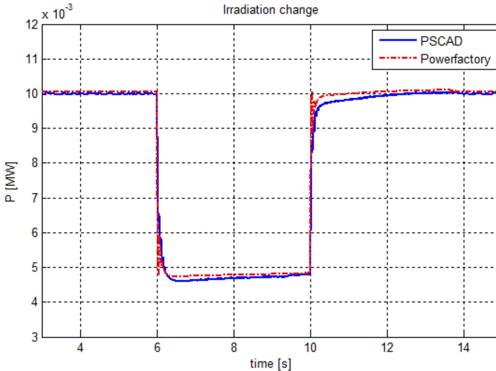
Fig. 5.37 Active power of the PV system
