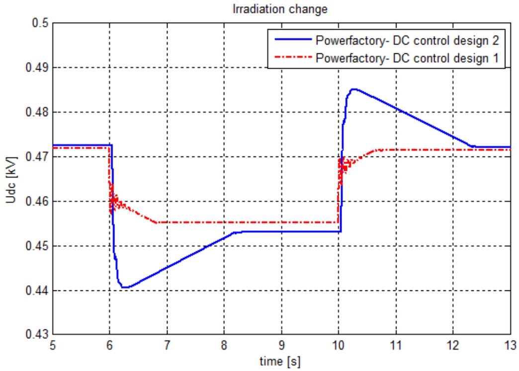
Fig. 5.38 DC voltage of the PV system
