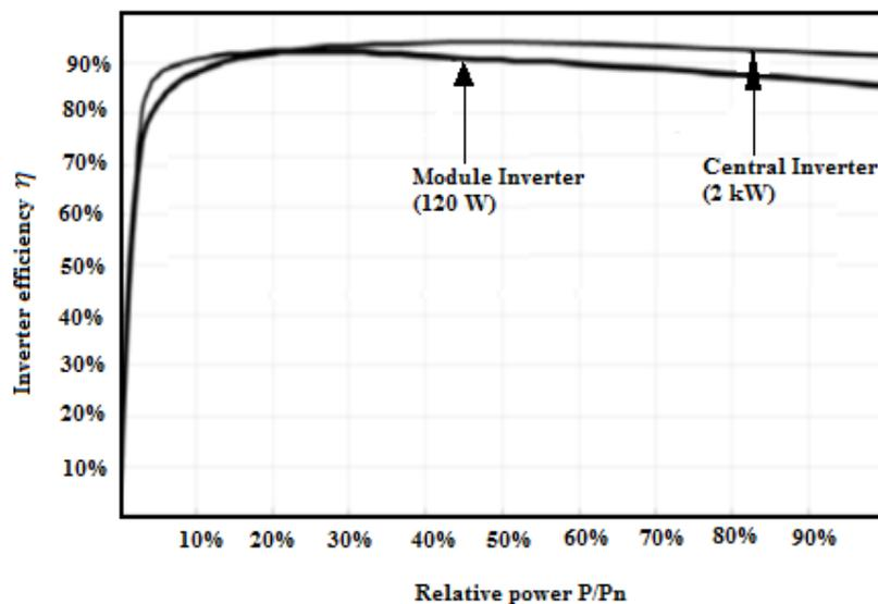
Fig. 2.9 Efficiency over a range of relative photovoltaic generator powers [13]
