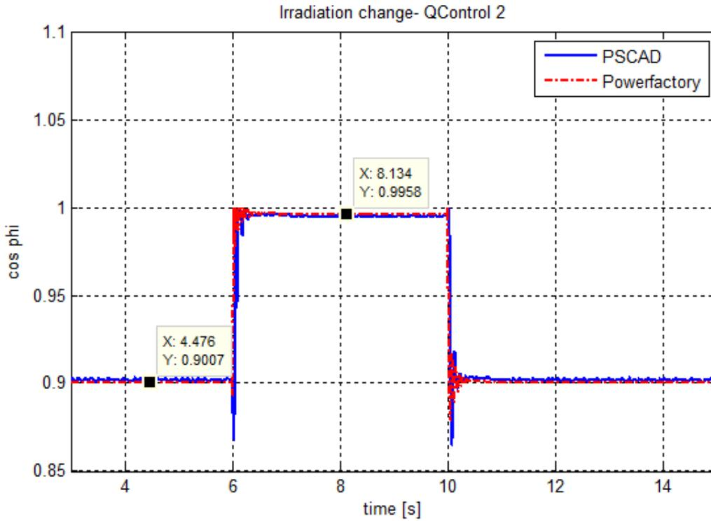
Fig. 5.11 Power factor of the PV system
