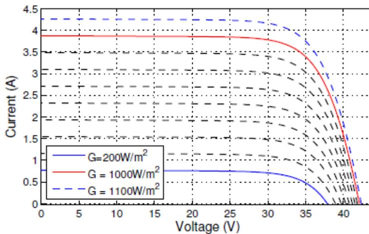
Fig.2.5 Irradiation dependence of Solar cells [4]
