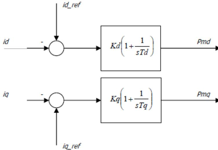
Fig. 4.6 Built-in current controller [19]
