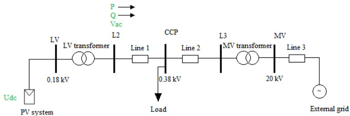
Fig. 5.1 Single-line diagram of the grid connected PV system
