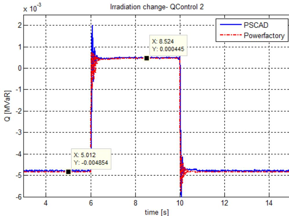
Fig. 5.10 Reactive power of the PV system
