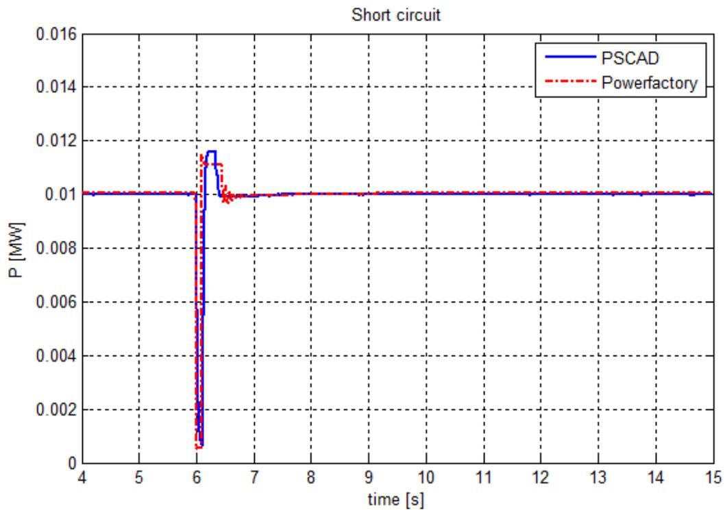
Fig. 5.24 Active power of the PV system
