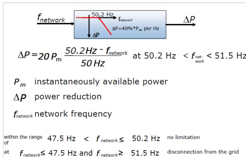
Fig. 2.12 Active power reduction in case of over frequency [5]
