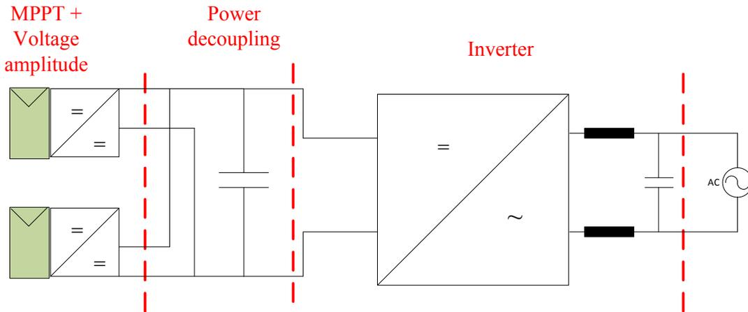
Fig. 2.7 DC-DC converter topology without transformer [9]
