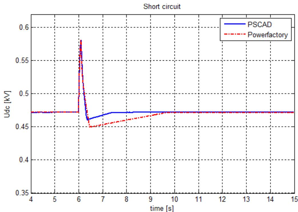
Fig. 5.25 DC voltage of the PV system
