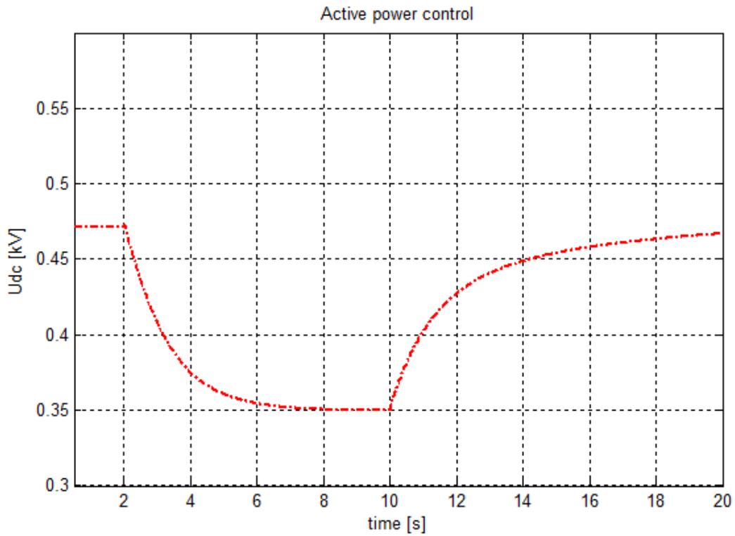
Fig. 5.27 DC voltage during active power control
