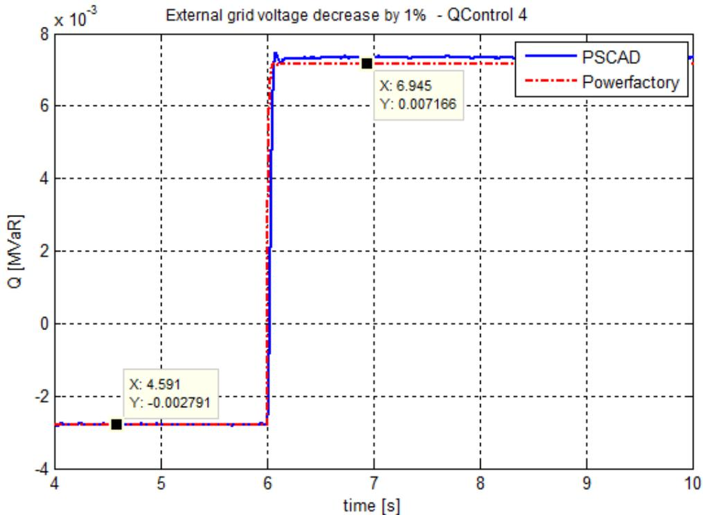
Fig. 5.18 Reactive power of the PV system
