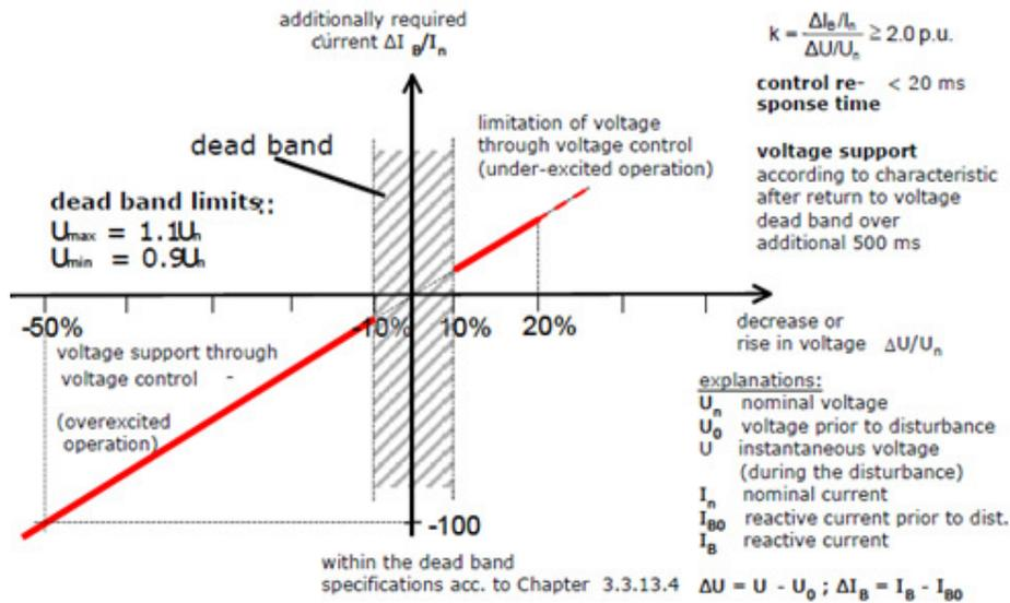
Fig. 2.11 Principle of voltage support at the event of network fault [5]
