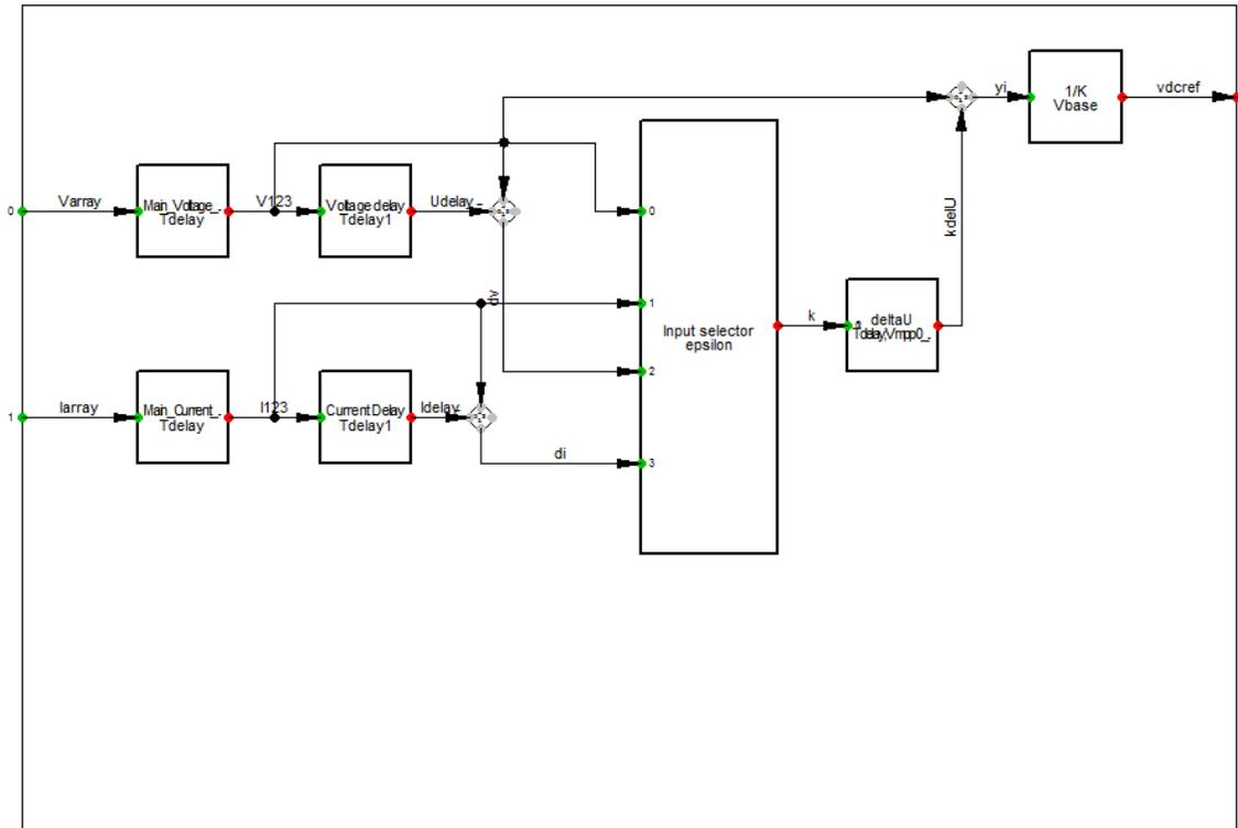
Fig. 8.4 MPPT block (slot 14)
