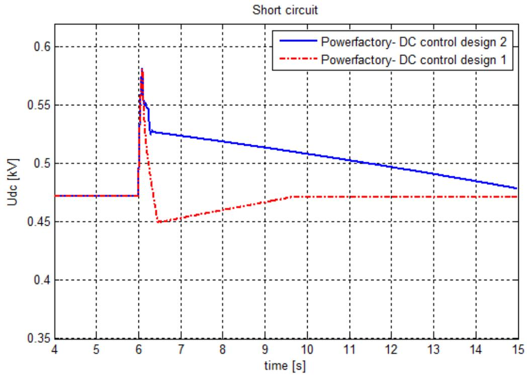
Fig. 8.11 DC voltage of the PV system
