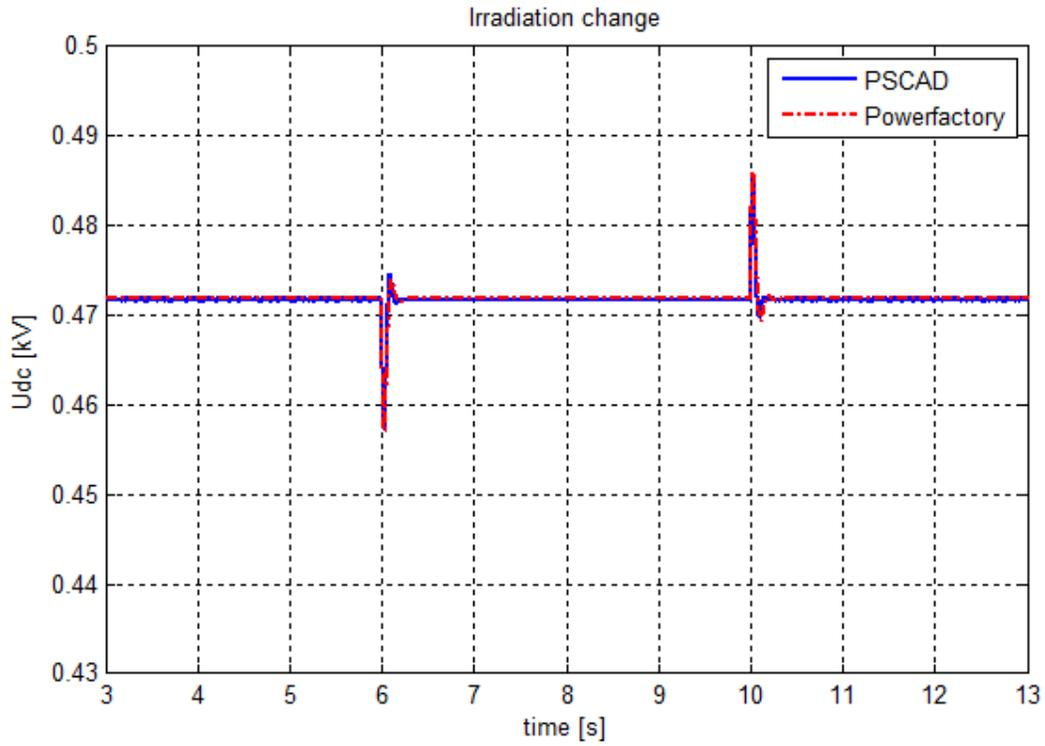
Fig. 5.31 DC voltage of the PV system
