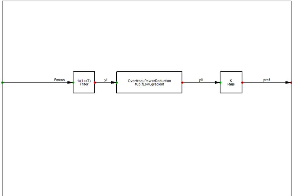
Fig. 4.9 Active power reduction block
