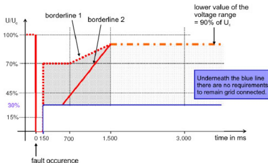
Fig.2.10 Limiting curves of voltage in the event of a network fault [6]
