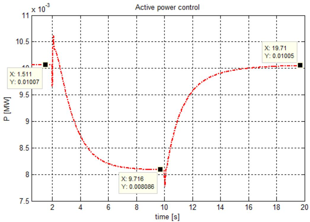
Fig. 5.28 Active power of the PV system
