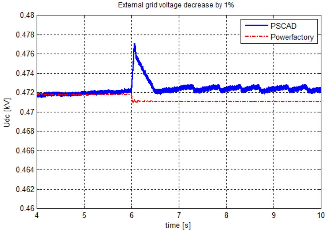
Fig. 5.15 DC voltage of the PV system
