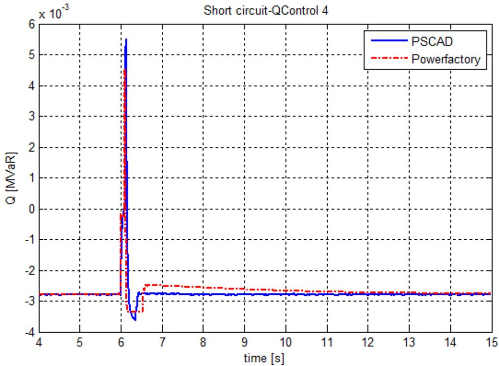
Fig. 5.26 Reactive power of the PV system
