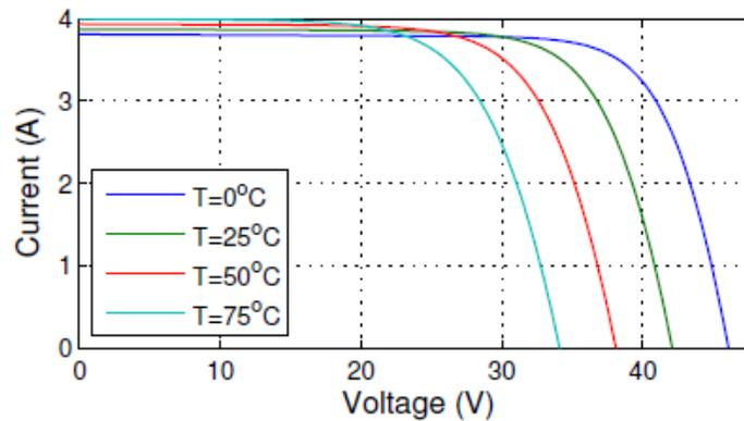
Fig.2.4 Temperature Dependence of Solar Cells [4]
