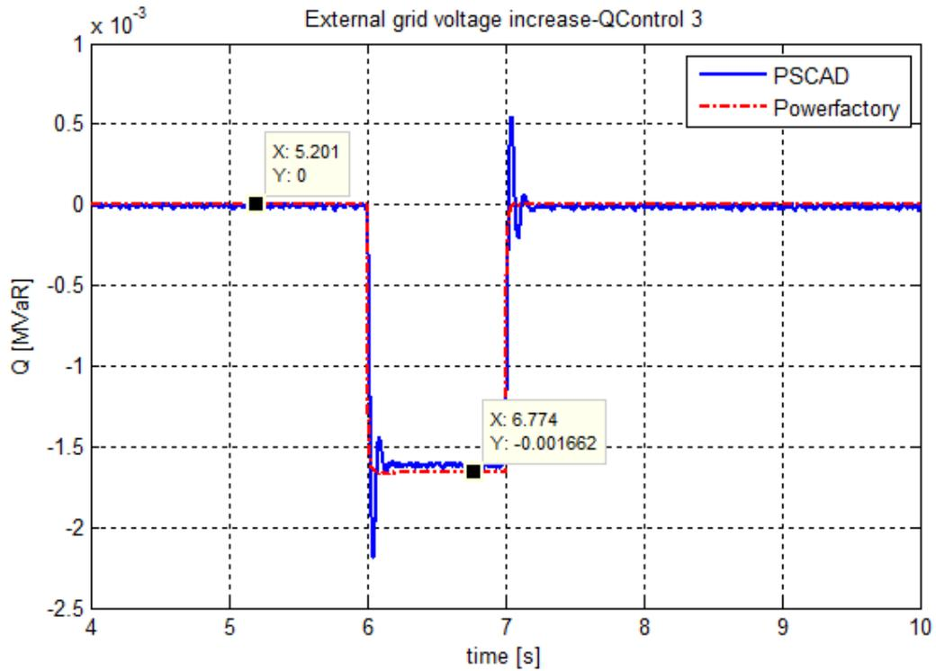
Fig. 5.22 Reactive power of the PV system
