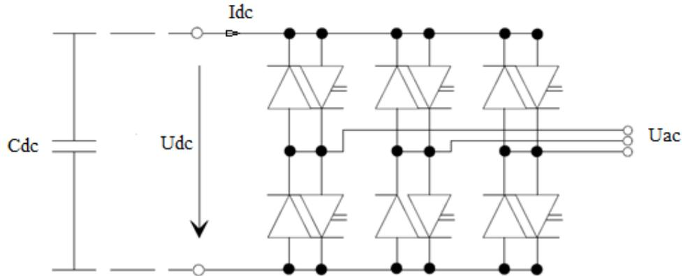
Fig. 4.2 Equivalent circuit with DC-link capacitor [19]
