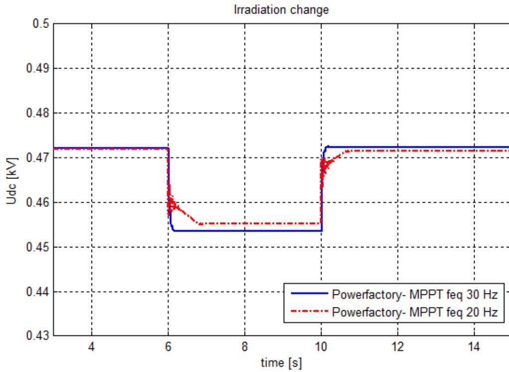
Fig. 5.34 DC voltage of the PV system
