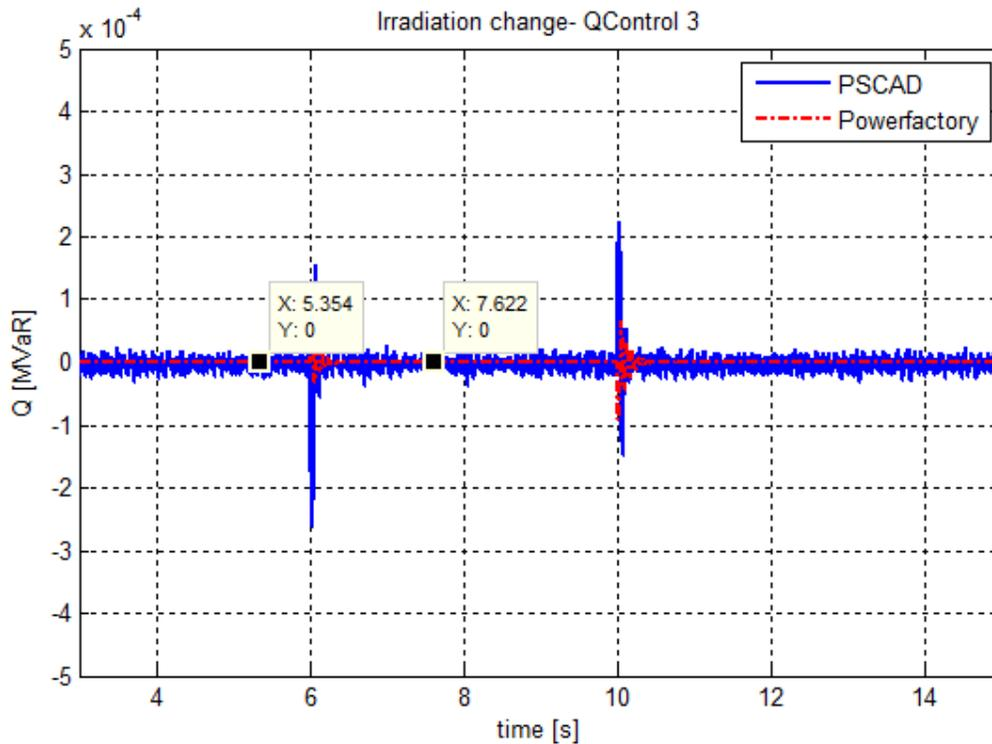
Fig. 5.13 Reactive power output of the PV system
