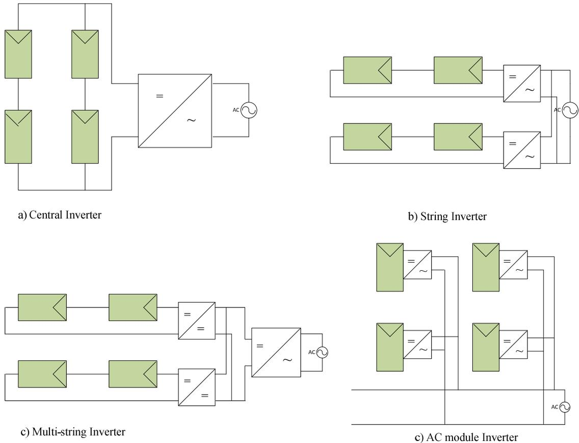
Fig. 2.8 Different configurations for PV system [9]
