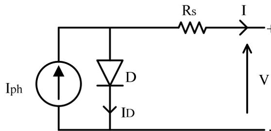
Fig. 4.18 Equivalent circuit of the solar cell
