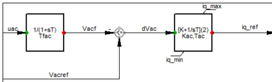
Fig. 4.13 AC voltage regulation
