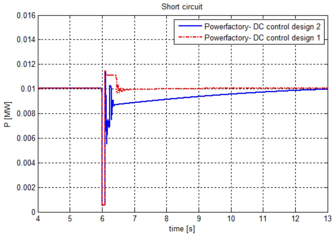
Fig. 8.12 Active power of the PV system
