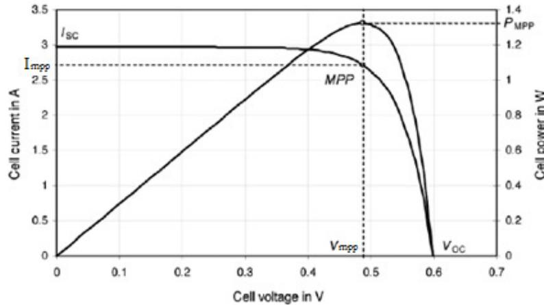
Fig. 2.3 I-V and P-V characteristic of a PV cell with MPP [3]
