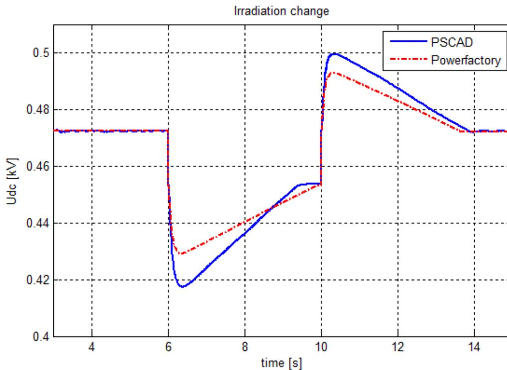
Fig. 5.36 DC voltage of the PV system
