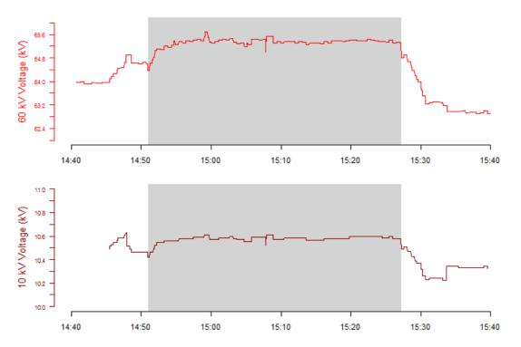
Figure 34 BID Substation Voltage Control during Islanding (60 and 10 kV). The traces compare the 60 kV and the 10 kV voltages at the BID substation during the test.
