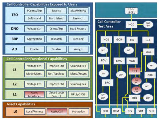
Figure 26 Cell Controller Configuration during Mini-Island Test (Wind Only Operation).
