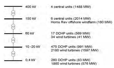
Figure 3 Production capacity per voltage level in the western part of Denmark in 2004.
