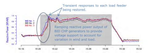
Figure 37 Reactive Power Support during Preload Plan with Small Import Test. Due to the significant presence of wind generation, the Cell Controller successfully dispatches the generation of reactive power to balance the cell.
