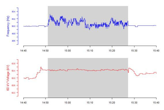
Figure 33 Cell Frequency and 60 kV Island Voltage Control as measured at the primary interconnect at Holsted. The region shaded grey indicates the time when the primary interconnect was open.
