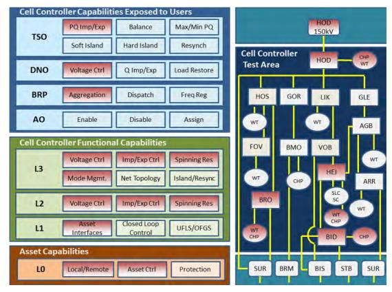
Figure 38 Cell Controller Configuration during Grid Connected Multi-Function Test. The left panels indicate which Cell Controller capabilities were being used during the test (highlighted in red) and the right panel highlights the Holsted Cell assets involved in the test.
