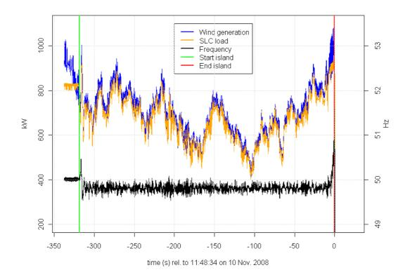
Figure 27 Effect of SLC during the Mini-Island Test. The black trace plots the observed frequency (Hz); the blue and orange traces plot wind generation (kW) and the SLC response (kW), respectively. The Cell Controller was able to maintain a stable frequency (nominal 50 Hz) during the test prior to black out. Note the SLC's ability to balance the wind generation.
