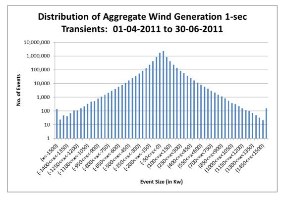
Figure 21 Distribution of Aggregated Wind Generation One-second Transients; the transients equal the second-to-second changes in total monitored wind generation in the Holsted Cell during the second quarter of 2011.
