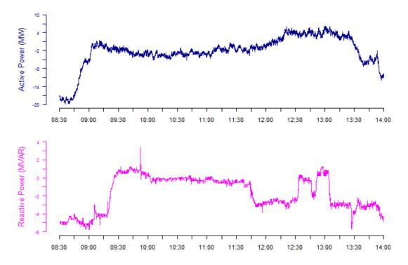
Figure 44 Recorded active (MW) and reactive power (MVAR) measurements while testing Multi-Function Operations over the course of the extended test.
