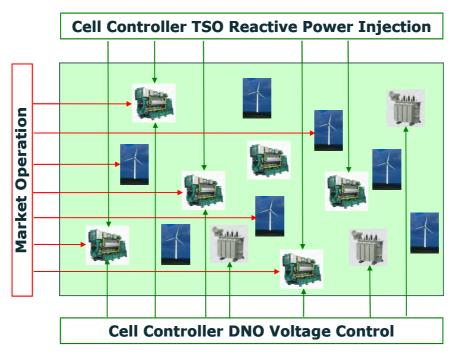
Figure 39 Multiple functionality of Cell Controller while in normal market operation
