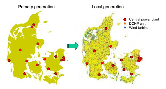
Figure 2 The development in Denmark from centralised to decentralised generation systems.
