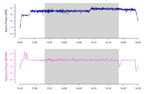
Figure 31 Brørup CHP in L1 Droop Mode. The active power of the cell (MW), the reactive power (kVAR). Note the stability of each trace; the active power was intentionally raised at 14:08 to accommodate changing condition within the cell. The region shaded grey indicates the time where the primary interconnect was open.
