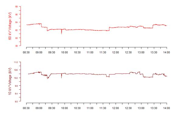
Figure 45 Recorded high (60 kV) and low (10 kV) side voltages at the primary interconnect (HOD) during testing of Multi-Function Operations
