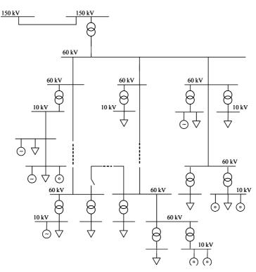
Figure 5 Simplified section of typical 60 kV distribution grid with DCHP plants (synchronous generators), WTs (induction generators) and 10 kV load feeders indicated.
