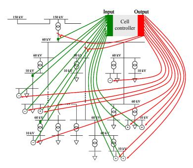
Figure 6 Cell Controller functionalities. Measuring and monitoring of load and production indicated by (green) arrows pointing towards the Cell Controller. Control actions on generators, load feeders and main power circuit breakers indicated by (red) arrows pointing away from the Cell Controller.
