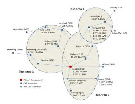
Figure 11 Topology of the Holsted Cell. The cell was divided into three test areas; testing prior to 2008 was performed in Area 1 only; the testing region was expanded to include Area 2 for 2008 and 2009, and all three Areas were involved in the testing done in 2010 and 2011.
