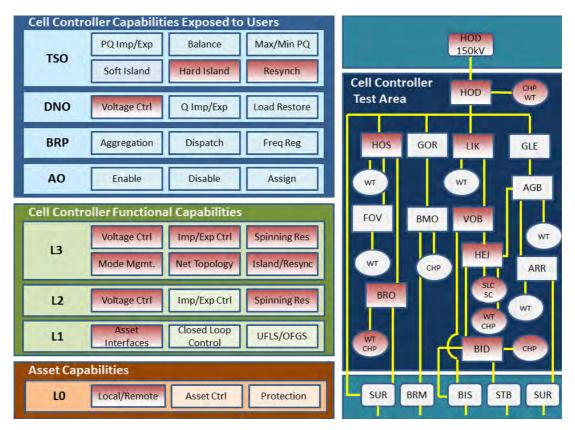
Figure 32 Cell Controller Configuration During Managed Island Test. The left panels indicate which Cell Controller capabilities were being used during the test (highlighted in red) and the right panel highlights the Holsted Cell assets involved in the test.
