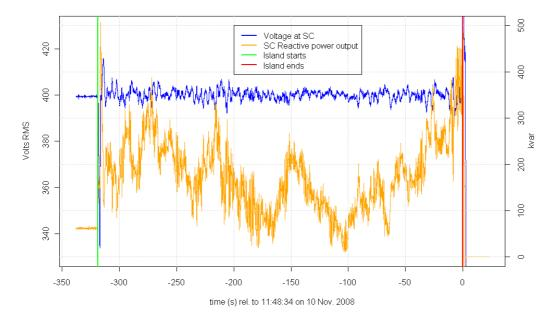
Figure 28 Effect of SC during the Mini-Island Test. The blue and orange traces plot the voltage and kVAR, respectively, measured at the SC. The Cell Controller was able to maintain a stable voltage until black out; as expected, the trace of the SC closely follows the wind generation trace.
