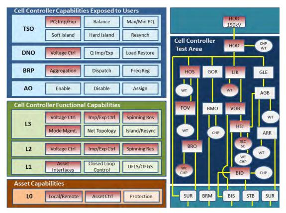
Figure 43 Cell Controller Configuration during Grid Connected Multi-Function Extended Run Test. The left panels indicate which Cell Controller capabilities were being used during the test (highlighted in red) and the right panel highlights the Holsted Cells assets involved in the test.
