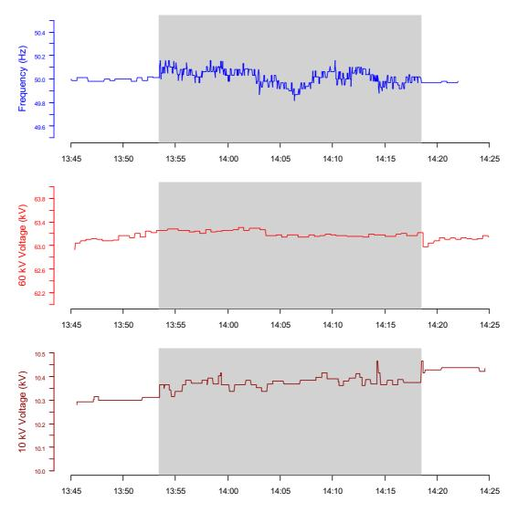
*Figure 30* Brørup CHP in L1 Droop Mode. The traces, from top to bottom, plot the cell frequency (Hz), the 60 kV voltage, and the 10 kV voltage as measured at the Holsted substation. The region shaded grey indicates the time where the primary interconnect was open.
