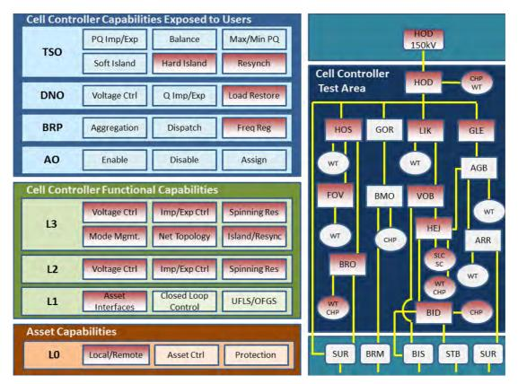
Figure 35 Cell Controller Configuration during Preload Plan with Small Import Test. The left panels indicate which Cell Controller capabilities were being used during the test (highlighted in red) and the right panel highlights the Holsted Cell assets involved in the test.
