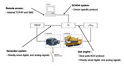
Figure 8 Typical existing communication system loop of a gas engine CHP unit designed for parallel operation with the grid. Exhaust boiler system not shown.
