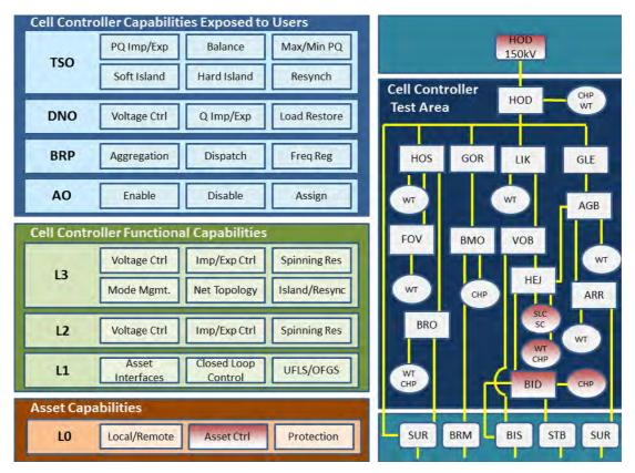
Figure 22 Cell Controller Configuration during SLC performance analysis. The left panels indicate which Cell Controller capabilities were being used during the test (highlighted in red) and the right panel highlights the Holsted Cells assets involved in the test.
