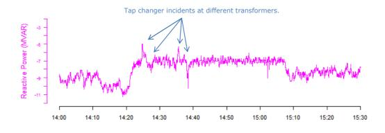
Figure 40 Resulting Cell area total reactive power import
