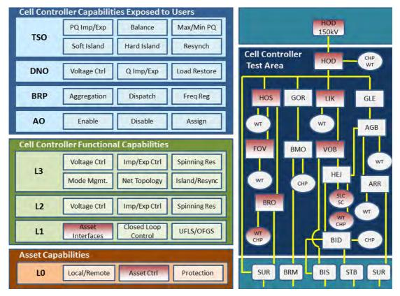
Figure 29 Cell Configuration during L1 Testing. The left panels indicate which Cell Controller capabilities were being used during the test (highlighted in red) and the right panel highlights the Holsted Cells assets involved in the test.
