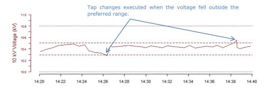
Figure 41 Example of Cell Controller adjusting tap on 60/10 kV transformer. The preferred and allowable ranges are indicated by the dashed and dotted lines, respectively.
