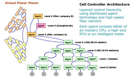
Figure 7 Basic Cell Controller architecture for one cell indicated in green.
