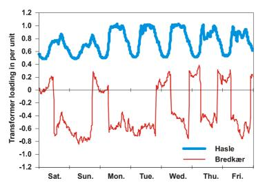
Figure 4 Power flow in two 150/60 kV distribution transformers measured during one ordinary week in 2004.
