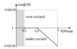
Fig. 1: Standard characteristic curve for cos (P)
