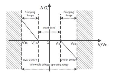
Fig.2 : Graphical schematic of droop-based voltage control.
