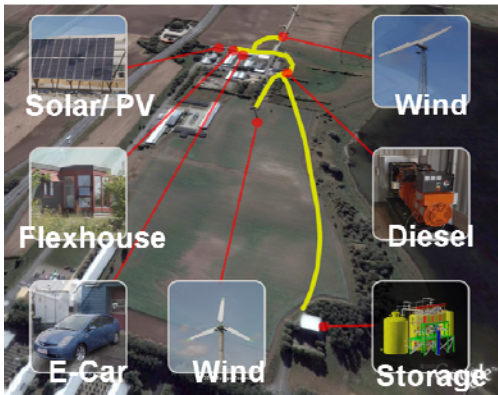
Figure 2: The SYSLAB experimental power system at DTU, Risø Campus. The large and rapid power fluctuations caused by these passing clouds is a challenge for the power system – for the control, the power quality and the stability. However, the fluctuations of the aggregated power from the distributed PV panels are clearly reduced.
